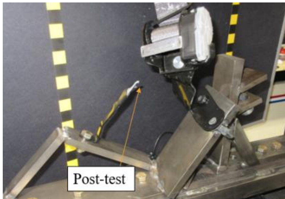
Figure 12. 2011 Ford Explorer Inflatable Belt Lap Belt Retractor Fracture.
