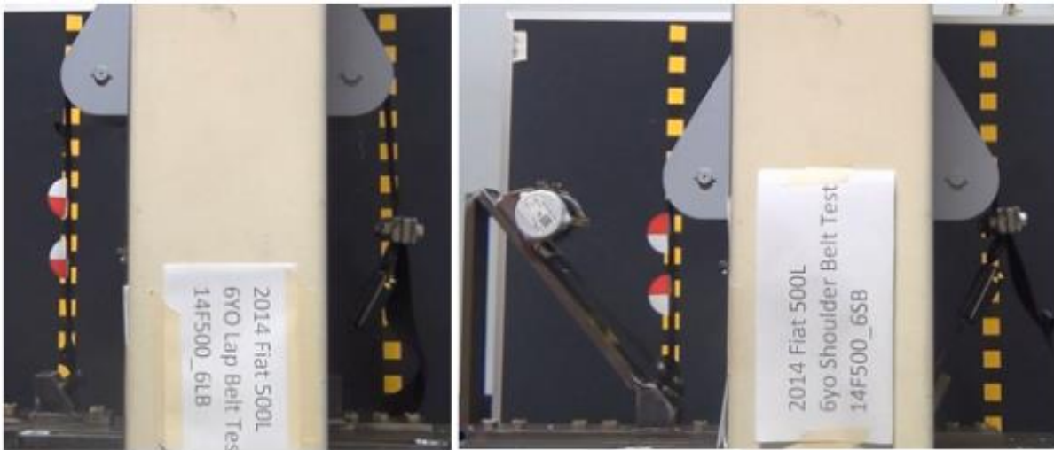
Figure 24. Updated Test Set-Up for Pelvis Loop (left) and Upper Torso Loop (right) of 2014 Fiat 500L Seat Belt Assembly.
