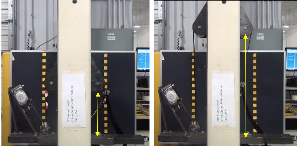
Figure E1. Crosshead of the Tensile Test Machine at Starting Position (left) Compared to Top of Stroke (right).
