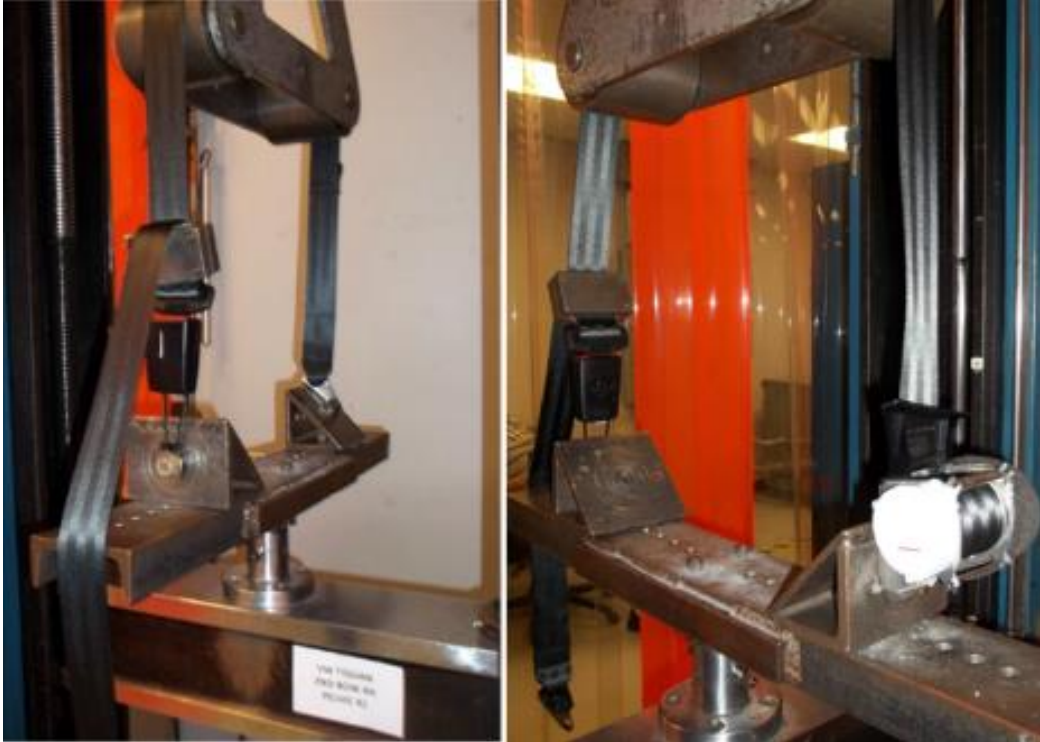
Figure 25. FMVSS No. 209 Test Set-Up for Pelvis Loop (left) and Upper Torso Loop (right) of 2014 Volkswagen Tiguan Seat Belt Assembly.
