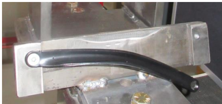
Figure 14. 2012 Mercedes S400 Guide Bar Fracture.
