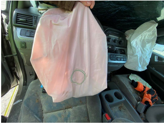
Figure 9. View of the driver's deployed frontal air bag in the Honda
