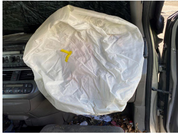
Figure 10. View of the passenger's deployed frontal air bag in the Honda
