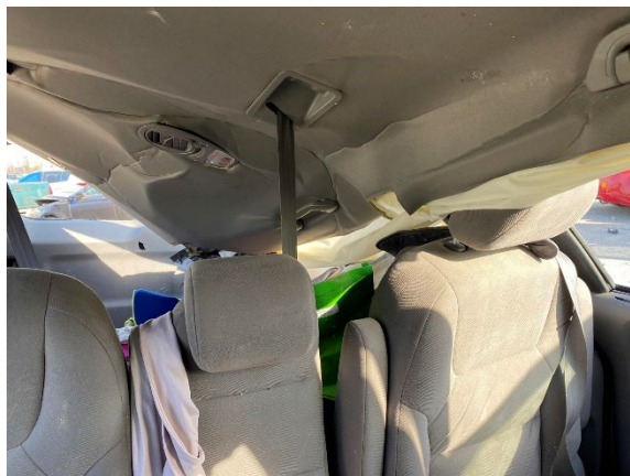
Figure 8. View of the interior of the Honda depicting the left-side intrusions at the C and D-pillars
