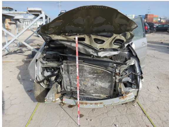
Figure 6. View of the front-plane damage of the Honda Odyssey
