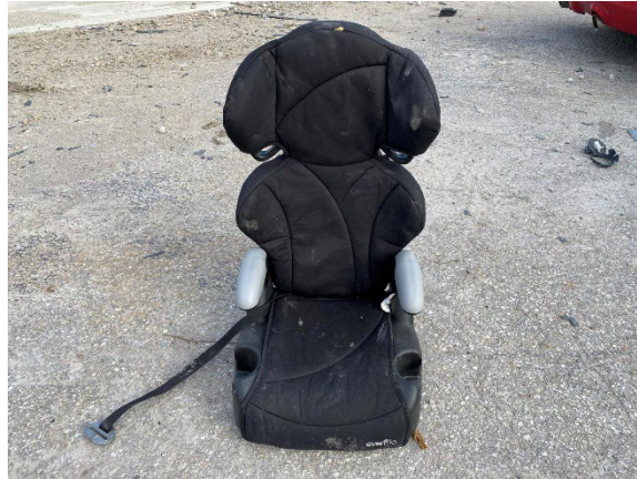
Figure 13. Child restraint system that was secured in the second-row-left seating position of the Honda
