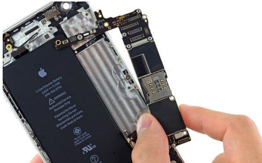
Removing an iPhone circuit board to recover the data, a service that Apple does not provide.
