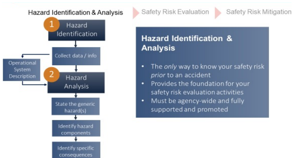
Figure 2-2 Hazard Identification and Analysis
