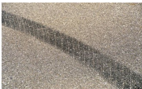
Figure B-20 Close-up View of Scuff Mark with Striations
