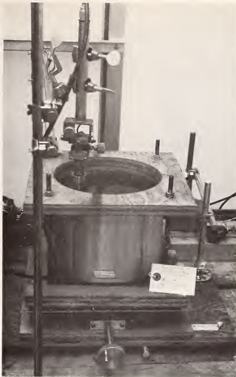
Figure 10. Bottomless Bucket Immersion Tank for Slab Specimens one or five MHz, with active face diameters of 1" and 3/4" respectively. Data were taken at test distances well within the near field distances ( N = \frac{D^2}{4\lambda} , where \lambda is measured in water) which are 4.25" and 12.0" respectively. Within this range the radiation field from such transducers is approximately a collimated beam having a cross section diameter equal to that of the active face. Thus the size of the surface resolution element is approximately 1" or 3/4" for the 1-MHz and 5-MHz data respectively.
