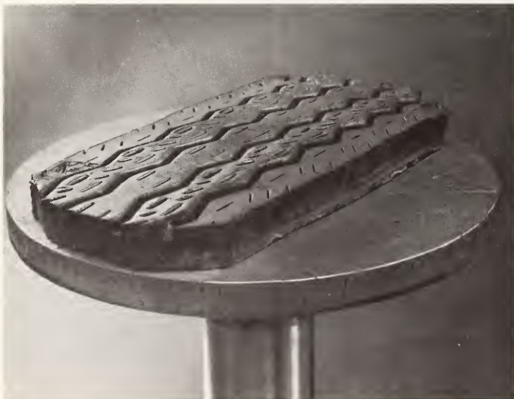
Figure 27. Worn Tread Section Scanned in Figs. 26, 29, 30, and 31.
