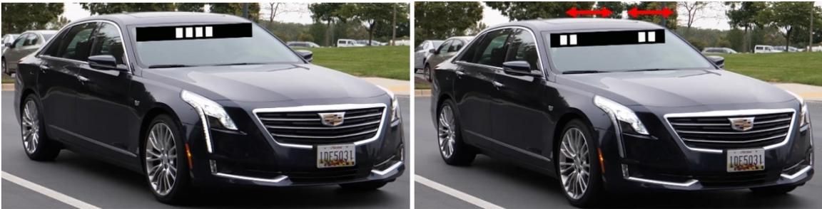
Figure 35. Light bar “in motion” (left) and “yielding” (right)
