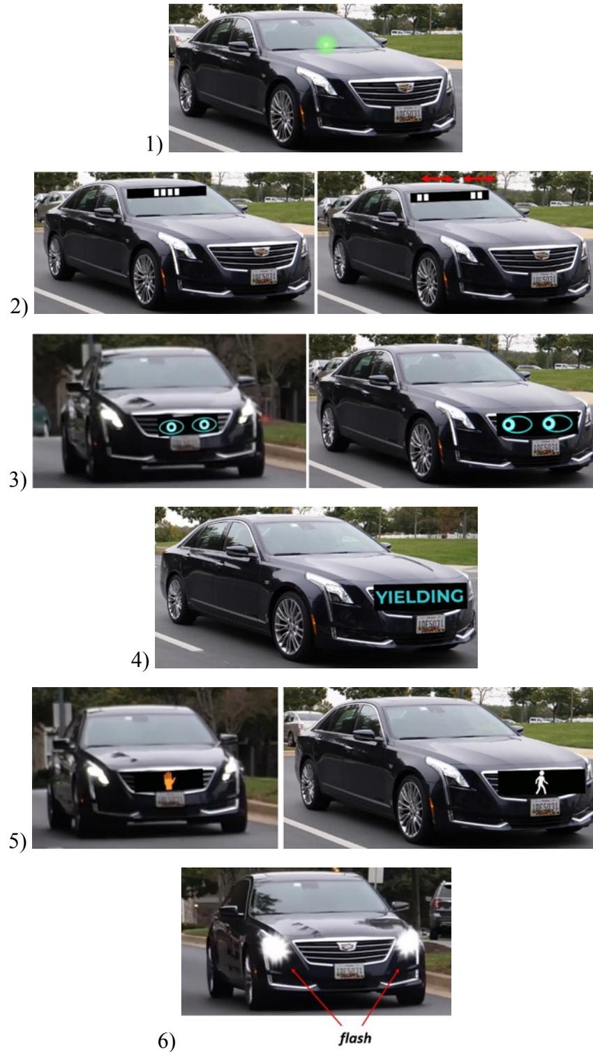
Figure E1. The eHMIs used in Study 3: 1) ADS beacon, 2) light bar, 3) “I see you” eyes, 4) “Yielding” text, 5) WALK/DON’T WALK icons, 6) headlamp flash
