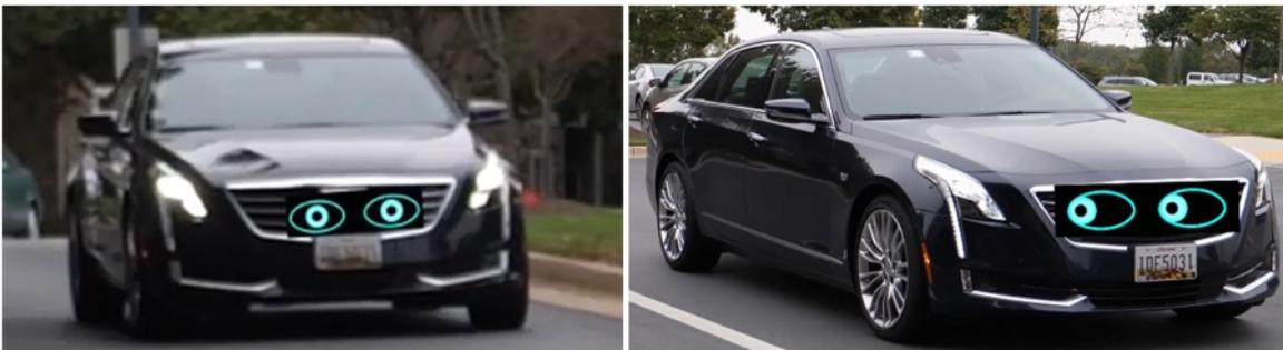
Figure 36. “I see you” eyes looking straight (left) and looking right (right)
