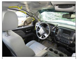
**Figure 18:** Left interior view depicting the driver contact evidence.
