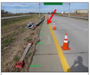
**Figure 4:** Northwest trajectory view at the end terminal impact. The location of the right rear tire mark is denoted by the red arrow.
