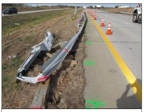
Figure 1: Northwest-facing view of the deformed ET-Plus guardrail end treatment and crash site.
