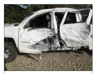
Figure 17: Left side of the Chevrolet depicting the Event 2 pole impact damage.
