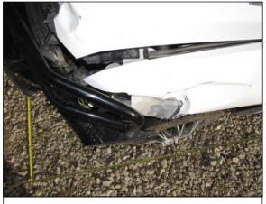
**Figure 16:** Overhead view of the front left corner of the Chevrolet depicting the impact deformation.
