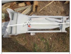
**Figure 13:** Overhead image of the end terminal depicting its deformation.
