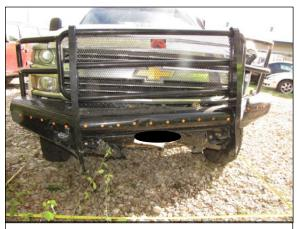
**Figure 15:** Front view of the Chevrolet and the deformation of the aftermarket bumper.
