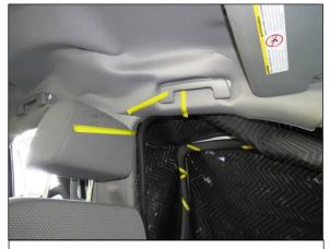
Figure 19: Interior view of the driver's rebound contact evidence.
