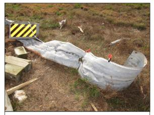
Figure 12: South-facing image of the extruded W-beam and the impact face of the end terminal.
