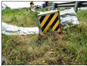
Figure 9: Image depicting the impact-face of the end terminal looking to the west.
