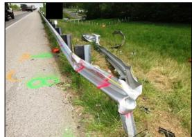
Figure 10: East-looking image of the deformed Wbeam wrapped around Post 7.
