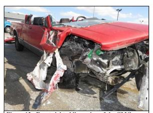
Figure 12: Front right oblique view of the GMC depicting the impact damage.
