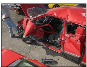
Figure 14: Left view of the GMC depicting the impact damage and intrusion at its left door.
