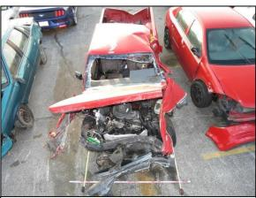
Figure 11: Overhead view of the GMC depicting its frontal damage.
