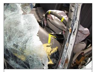
**Figure 16:** Penetration damage to the windshield, instrument panel, and steering wheel rim from the guardrail associated with Event 2.
