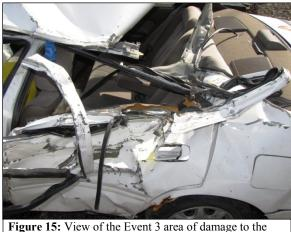
**Figure 15:** View of the Event 3 area of damage to the Toyota's left plane.
