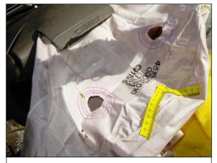
**Figure 21:** Abrasion to the top of the Toyota's driver air bag from contact with the intruded guardrail.
