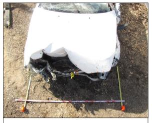
**Figure 12:** Overhead view of the Toyota depicting the frontal deformation.
