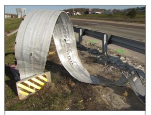
**Figure 5:** West-facing view of the ET-Plus end terminal impact head and deformed W-beam guardrail in their displaced position following the crash.
