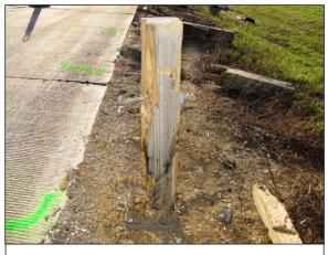
Figure 8: View of damaged Post 2 (repositioned for documentation during SCI reconstruction) and other sheared posts at the crash site.
