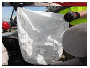
**Figure 23:** View of the deployed front right air bag in the Toyota at the time of the SCI inspection.
