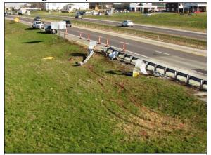
**Figure 3:** East-facing view of the crash site, the deformed guardrail, and vehicle tire marks, visible from a nearby overpass at the time of the SCI inspection.
