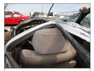
**Figure 19:** Intrusion of the Toyota's left B-pillar and left roof side rail induced by the engagement of the kinked guardrail with the roof structure.
