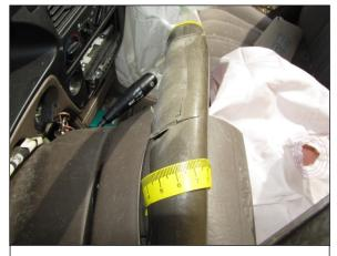
**Figure 17:** Damage to the steering wheel rim that resulted from contact with the guardrail as it penetrated into the Toyota's interior.
