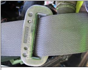
**Figure 16:** Heavy loading evidence in the belt path of the front right passenger's seat belt system within the Scion.
