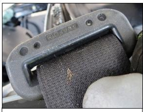
**Figure 14:** Loading evidence within the belt path of the driver's latch plate in the Scion.
