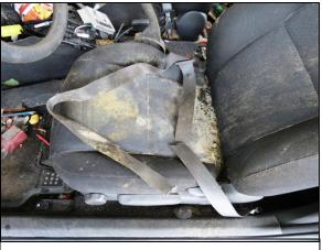
**Figure 15:** View of the cut driver's seat belt system within the Scion at the time of the SCI inspection.
