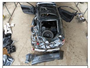
**Figure 9:** Rear view of the Scion's top plane and visible rollover damage from a rear perspective.
