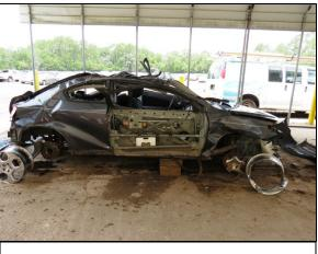
Figure 7: Right plane damage to the Scion.
