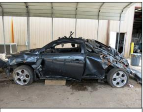
**Figure 6:** Left plane damage and rollover crush to the Scion's left roof side rail and left C-pillar.
