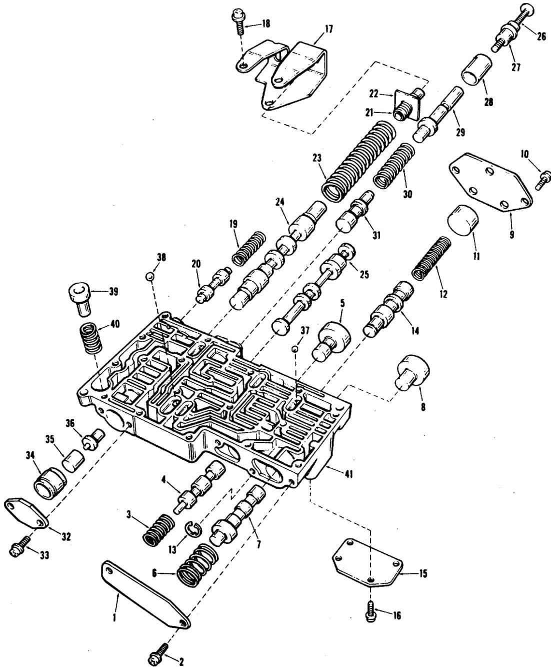
Figure 6-32. Control Valve Assembly - Internal Parts
