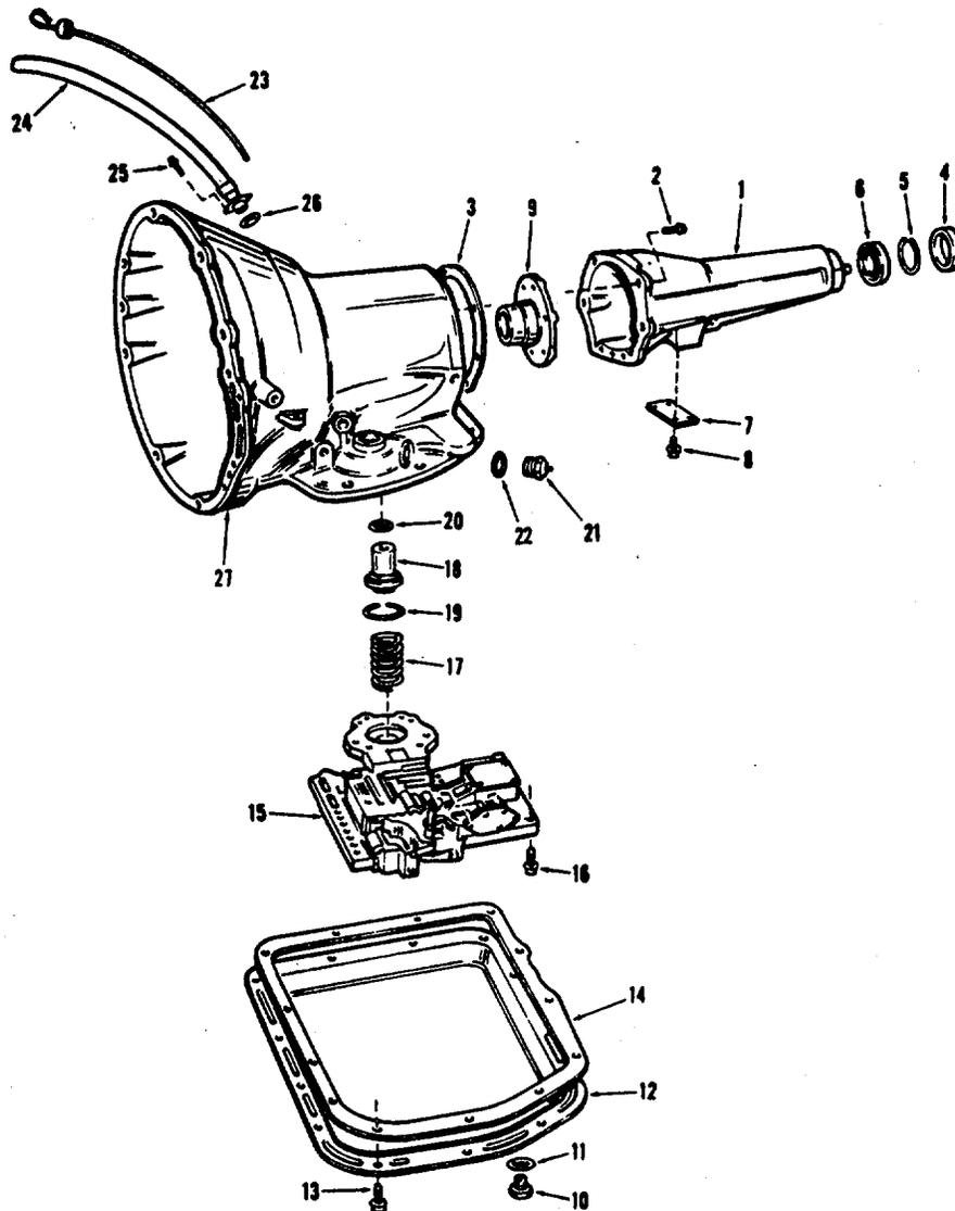
Figure 6-30. Transmission Assembly
