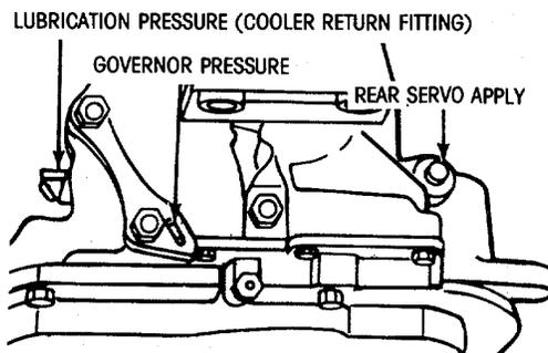
Figure 5-19. Pressure Test Locations (Rear End of Transmission)
