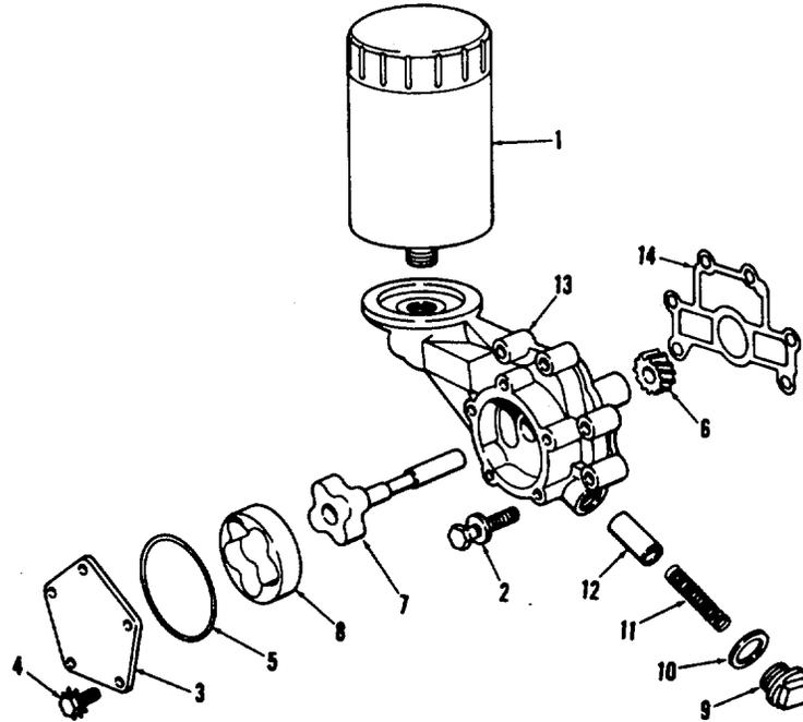
Figure 6-12. Engine Oil Pump and Filter Assembly
