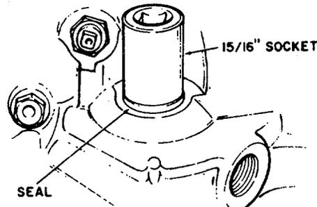
*Figure 5-15. Installation of Manual Lever Shaft Seal*
