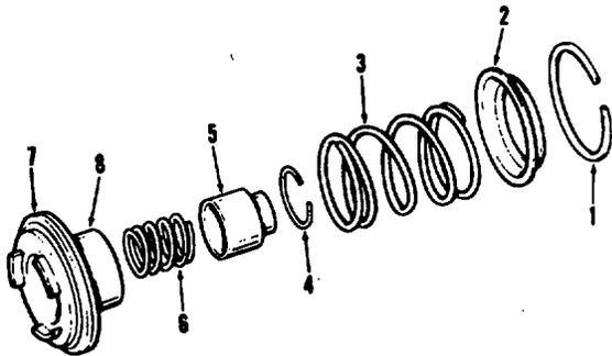
Figure 6-34. Low and Reverse Servo Assembly
