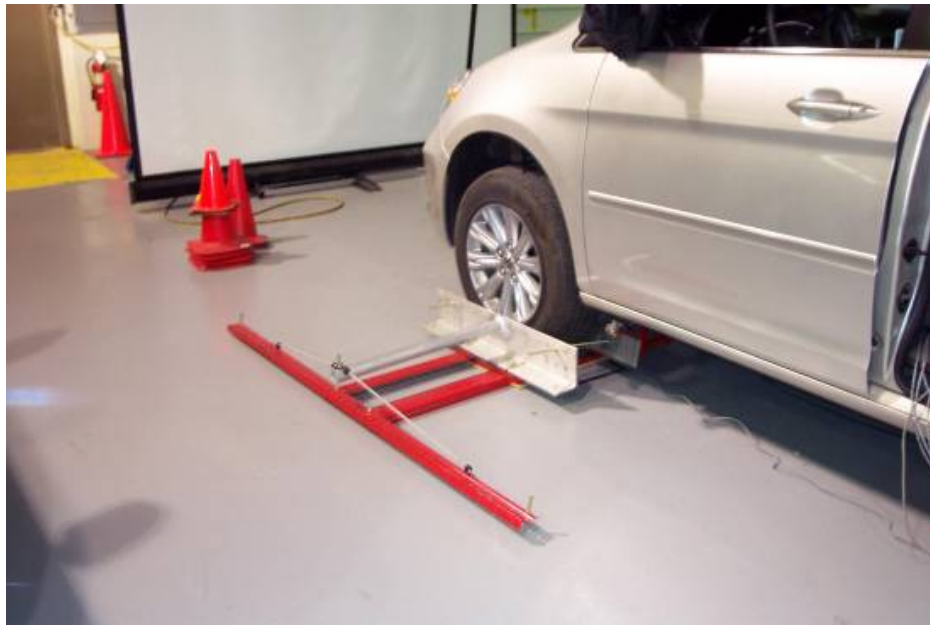
Figure 7. Steering Apparatus Installed on Front Tire
