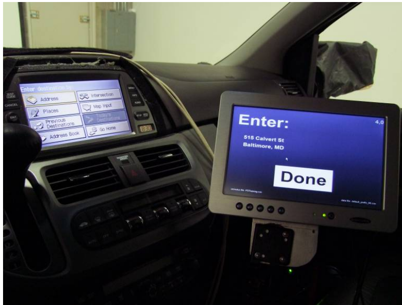
Figure 5. Odyssey Interior and Touch Screen Showing Secondary Task Stimulus
