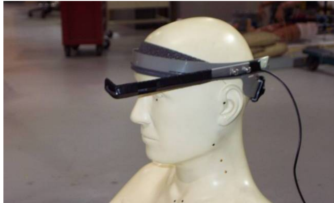
Figure 2. Head-Mounted Detection Task (HDT)
