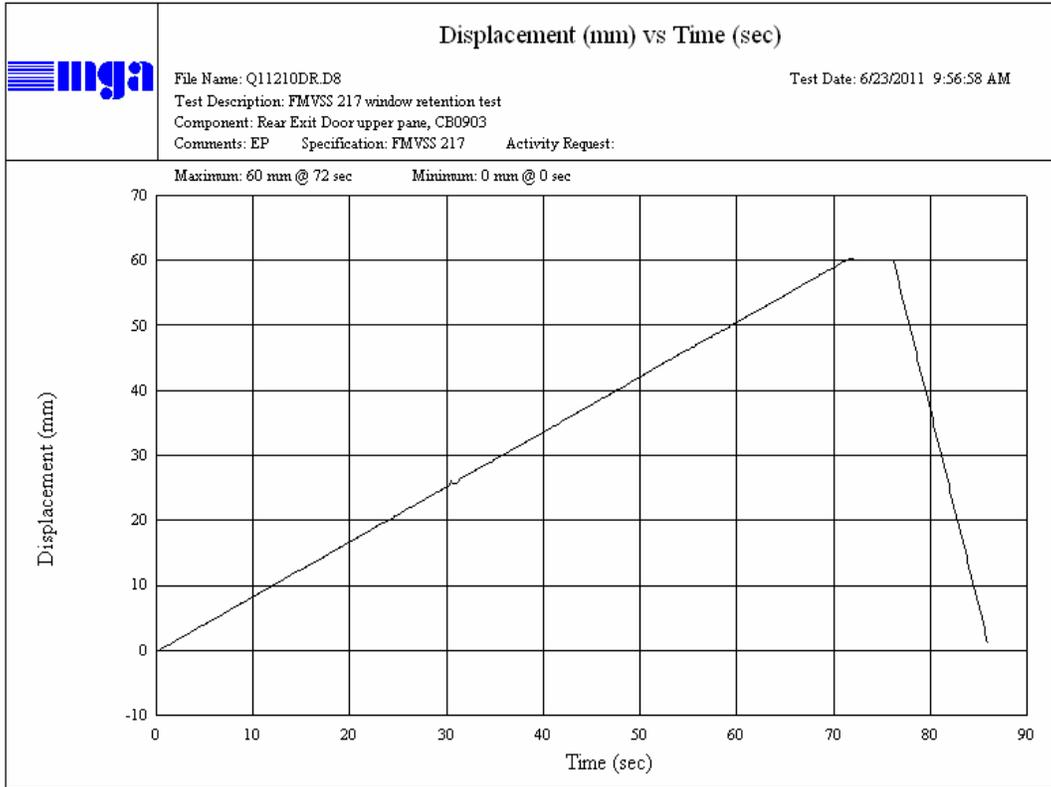
Rear Emergency Door Upper Window Displacement vs. Time
