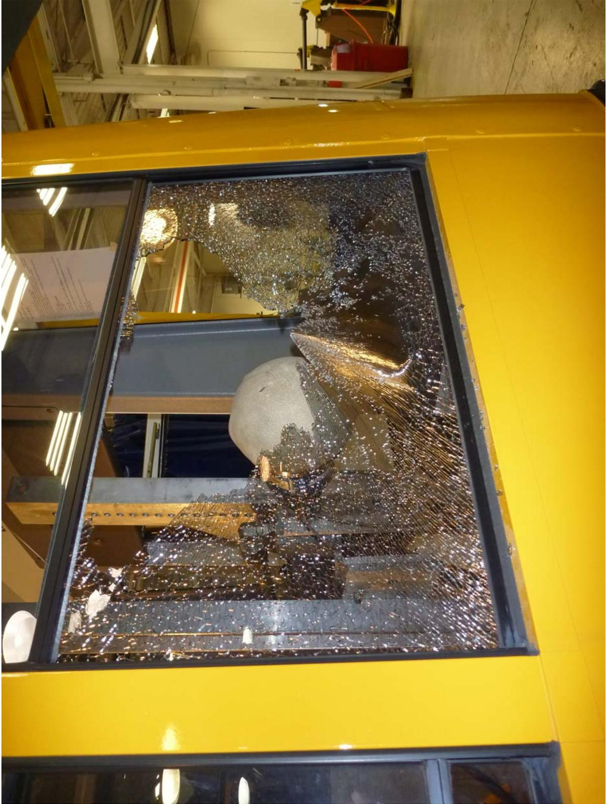
Window Retention Test of W4 Rearmost Driver Side Lower Window Outside View (Post-Test)
