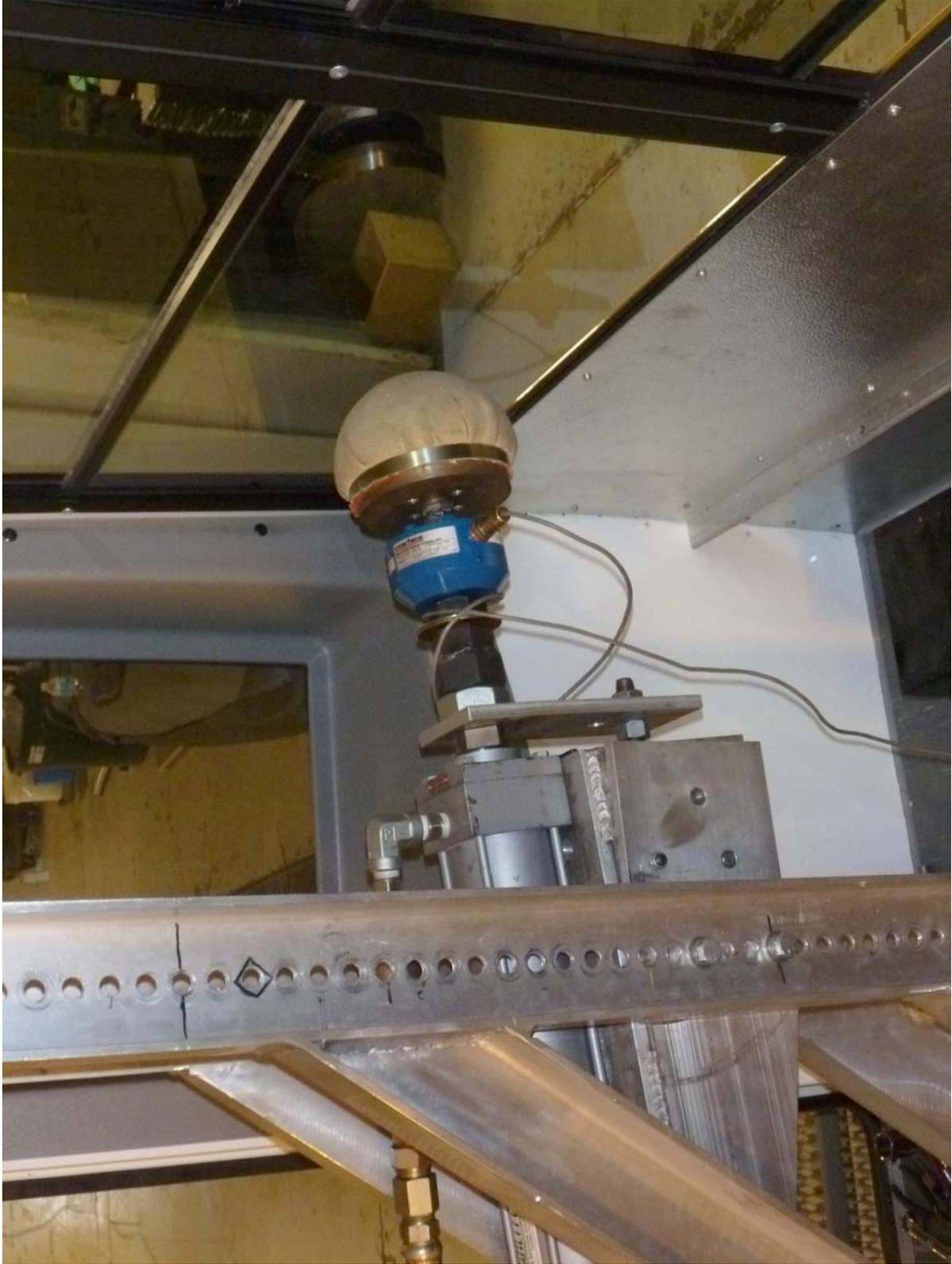
Window Retention Test of W4 Rearmost Driver Side Lower Window (Pre-Test)
