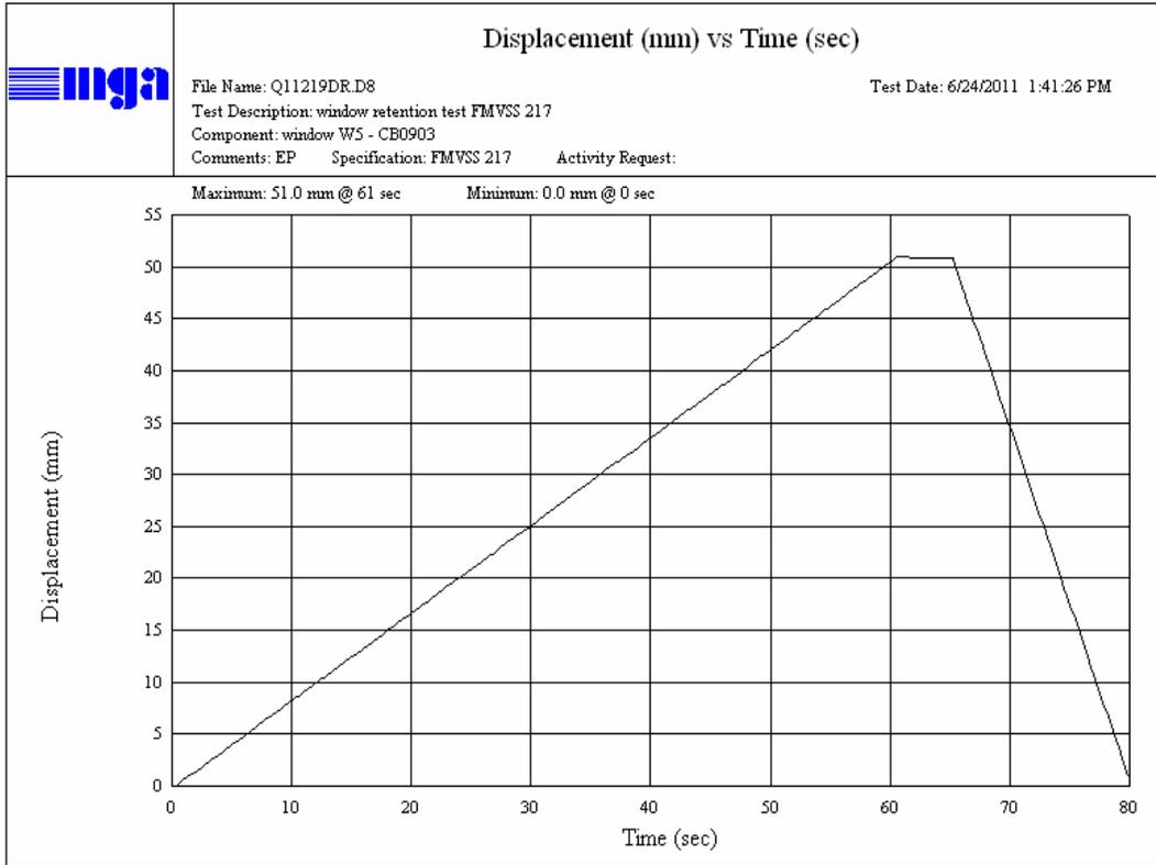
W5 Rearmost Passenger Side Upper Window Displacement vs. Time
