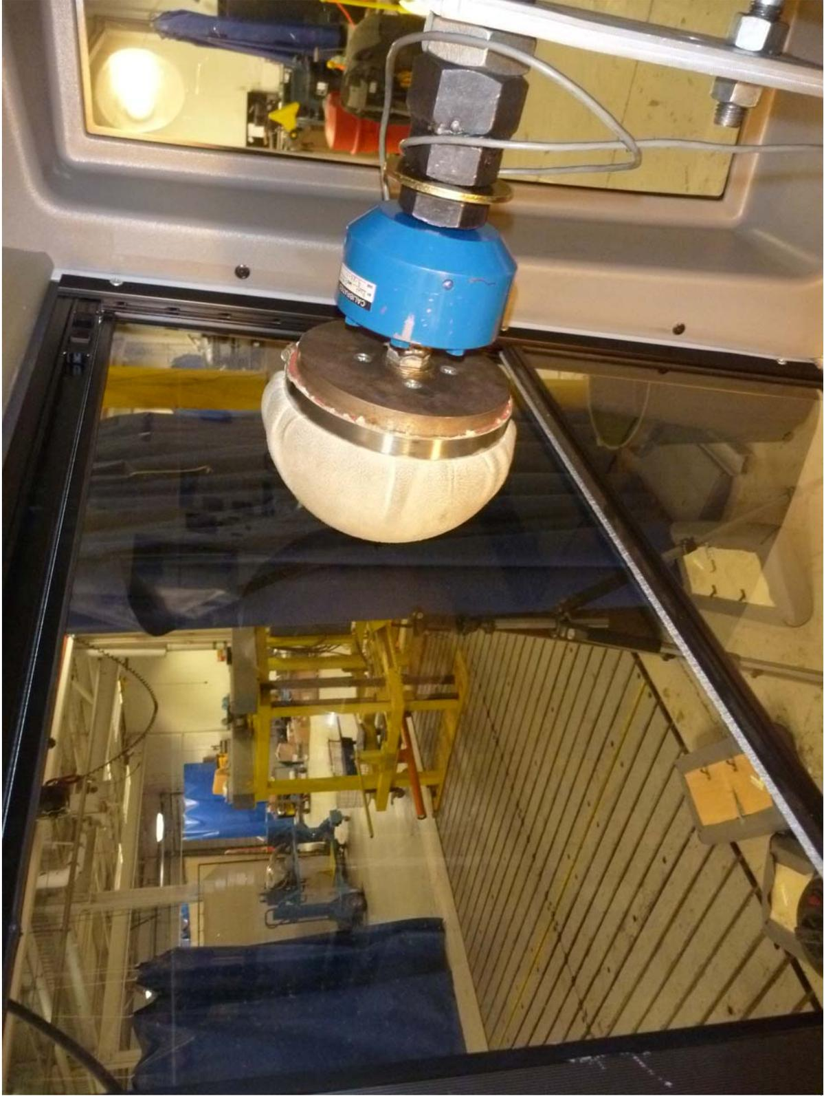
Window Retention Test of W5 Rearmost Passenger Side Upper Window (Pre-Test)
