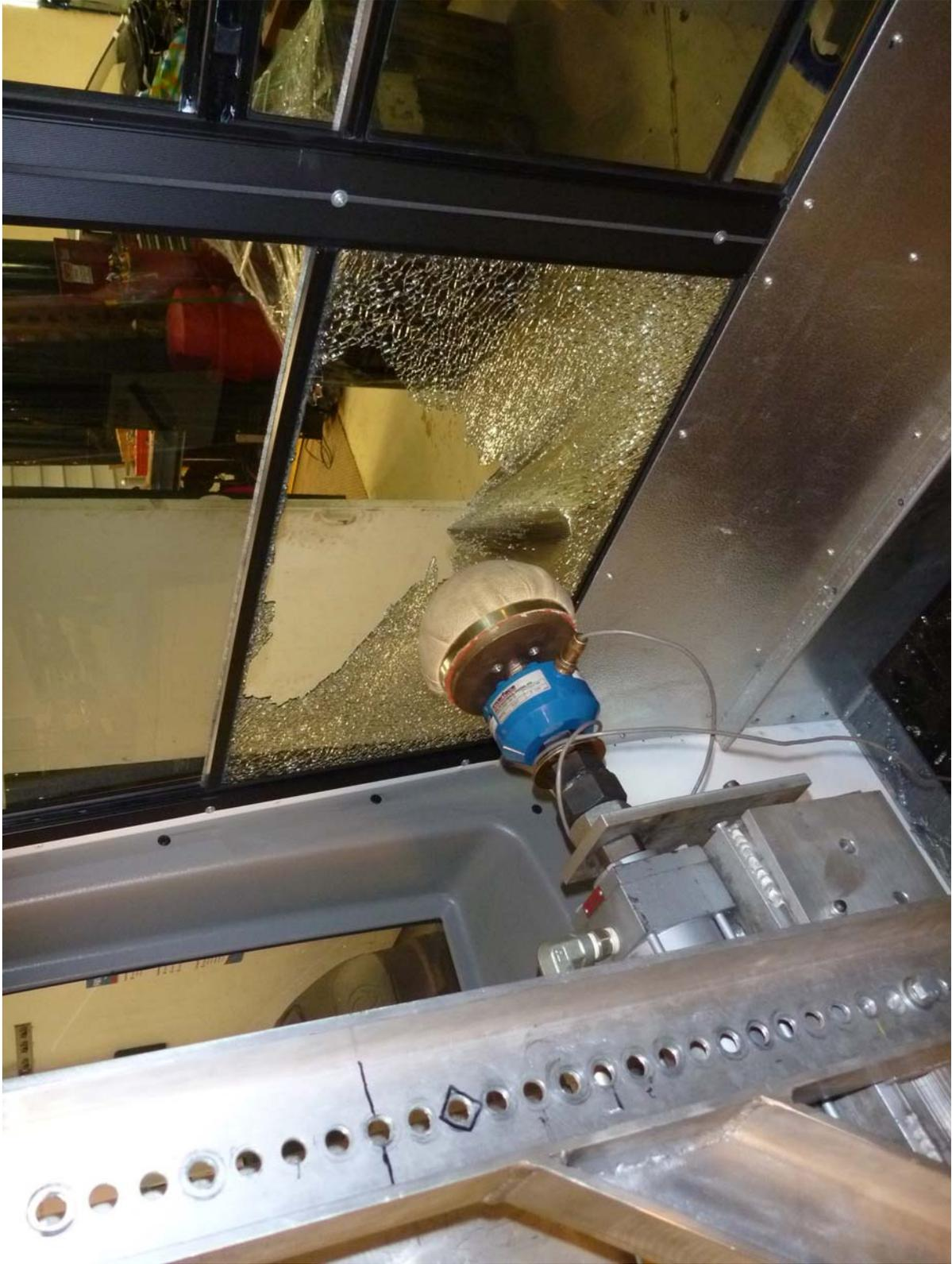
Window Retention Test of W4 Rearmost Driver Side Lower Window (Post-Test)
