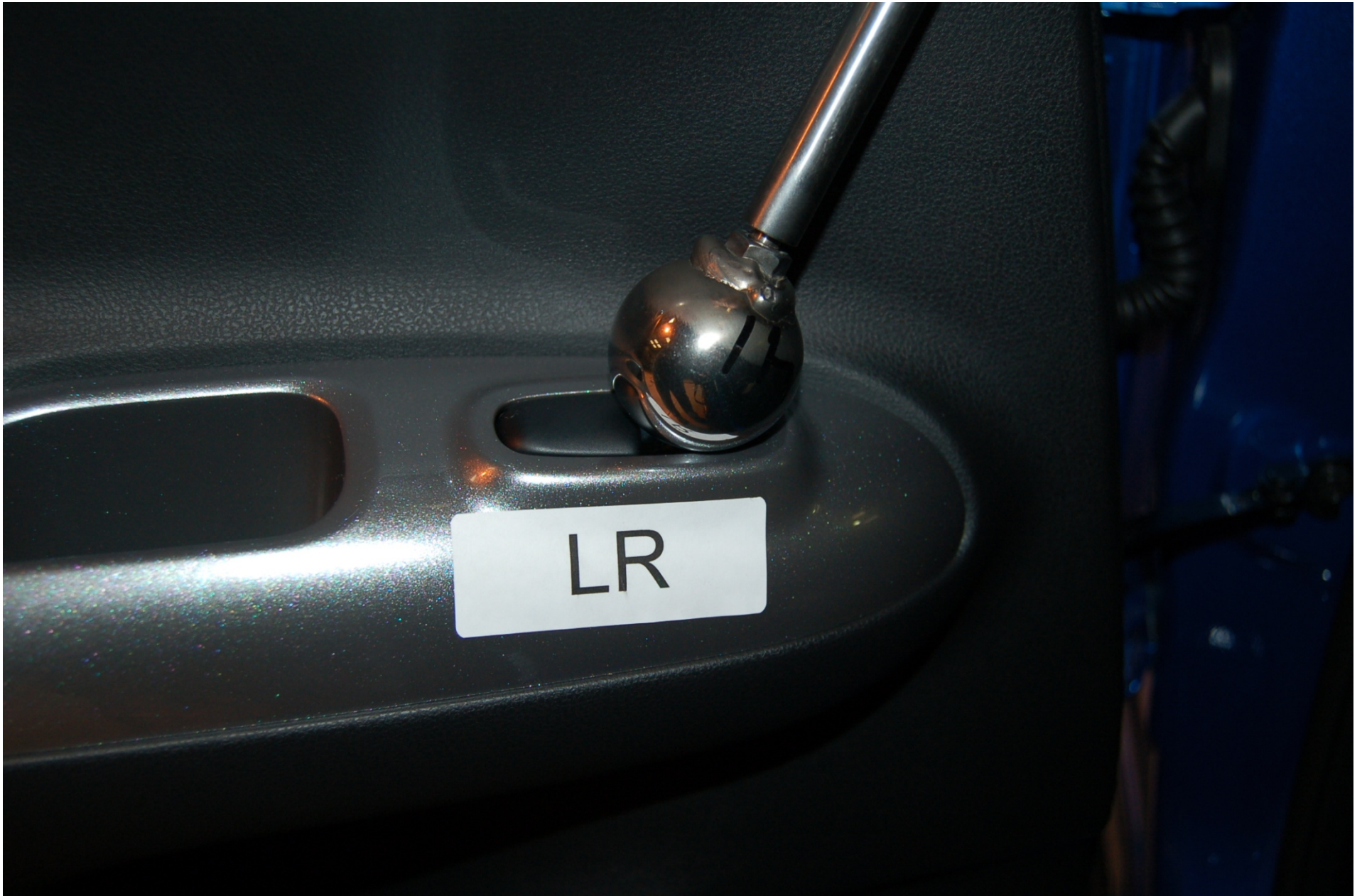
FIGURE 5.14 SPHERE TEST ON LEFT REAR SWITCH
