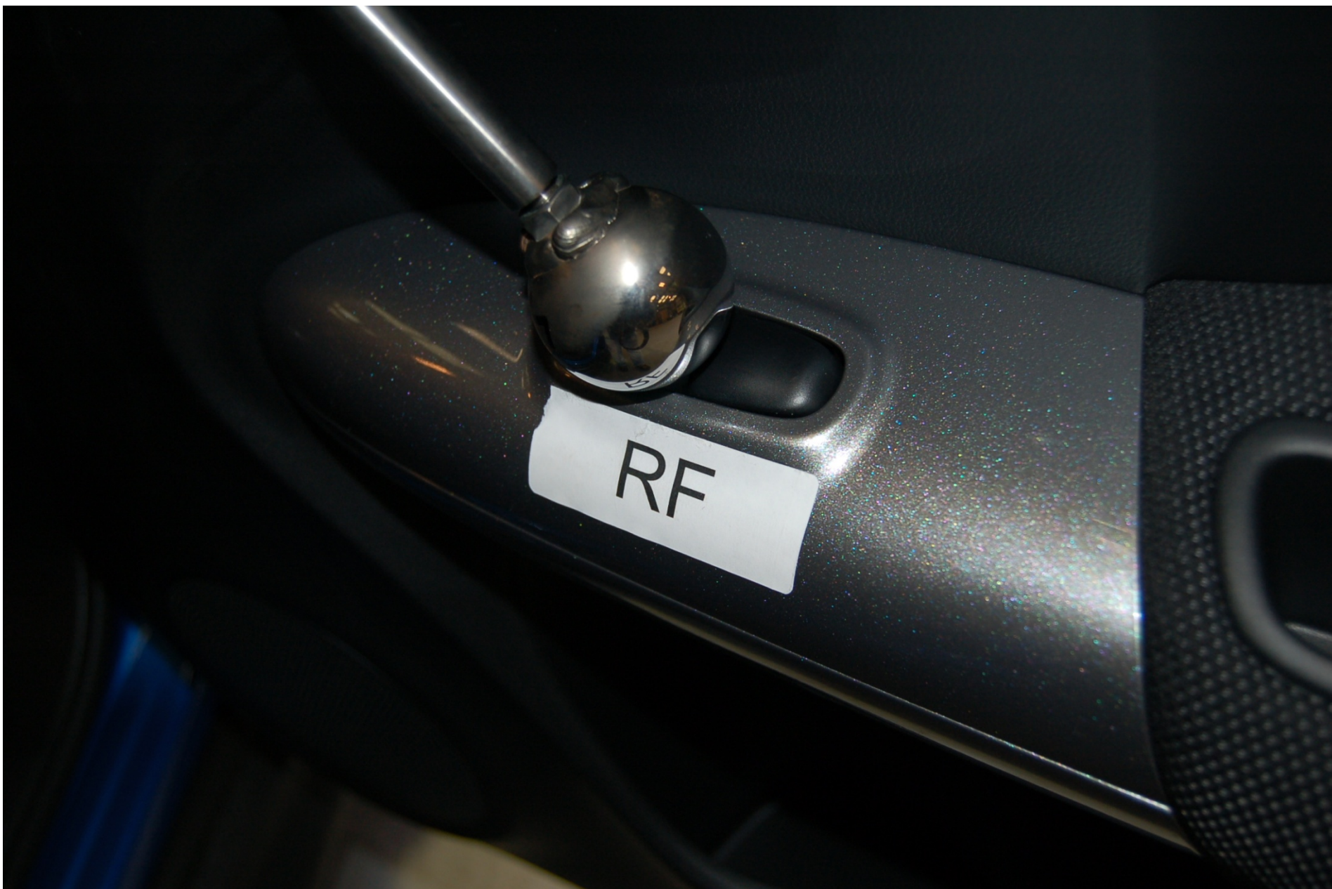
FIGURE 5.13 SPHERE TEST ON RIGHT FRONT SWITCH
