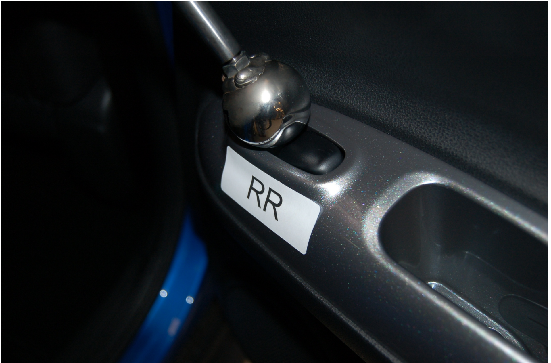
FIGURE 5.15 SPHERE TEST ON RIGHT REAR SWITCH
