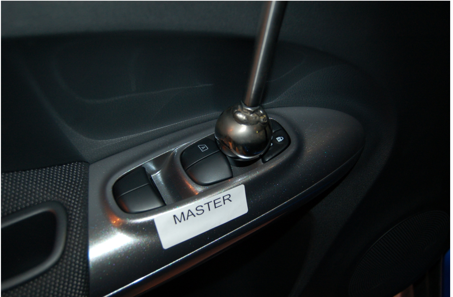
FIGURE 5.12 SPHERE TEST ON MASTER SWITCH
