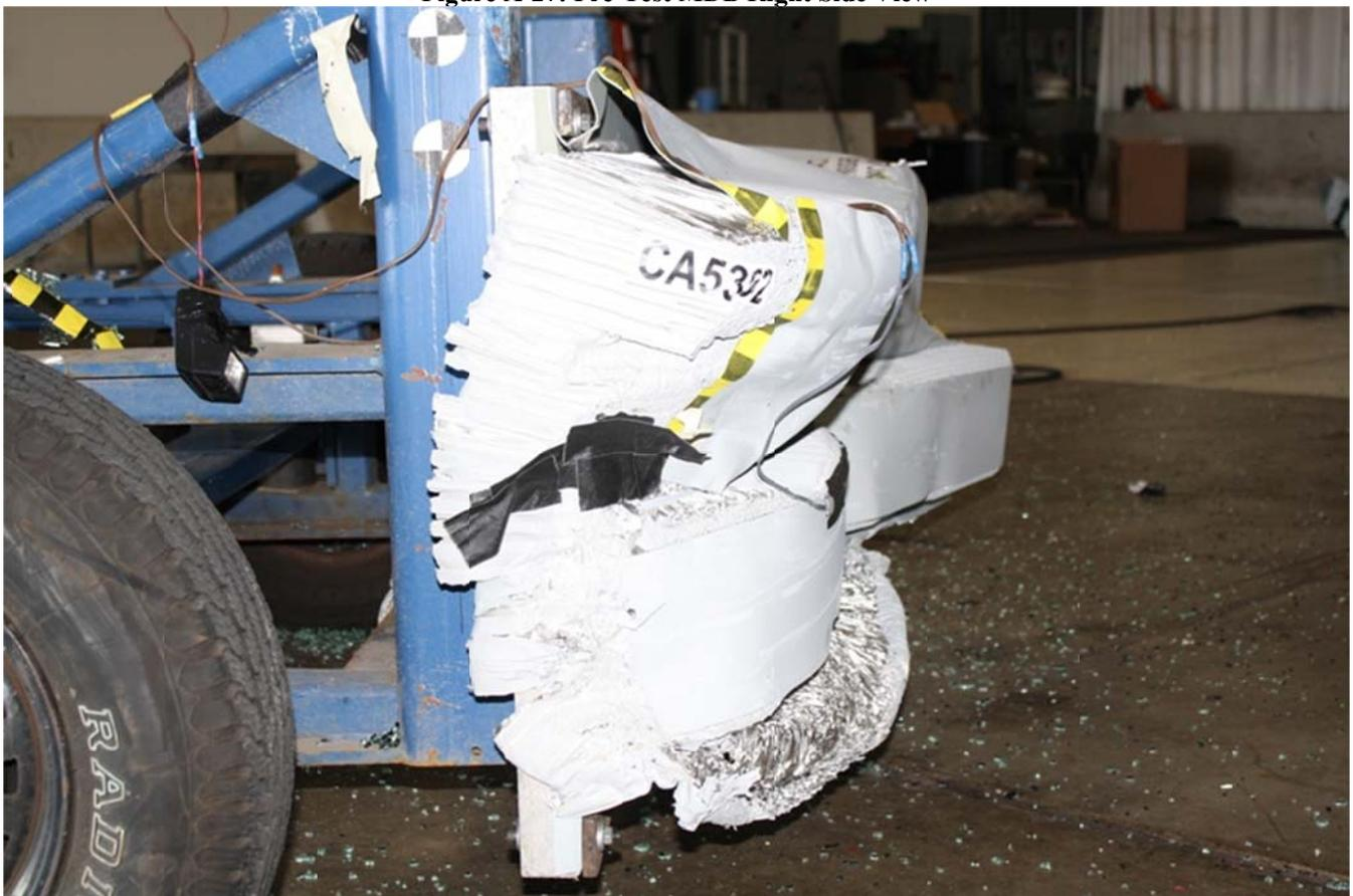
**Figure A-28: Post-Test MDB Right Side View**
