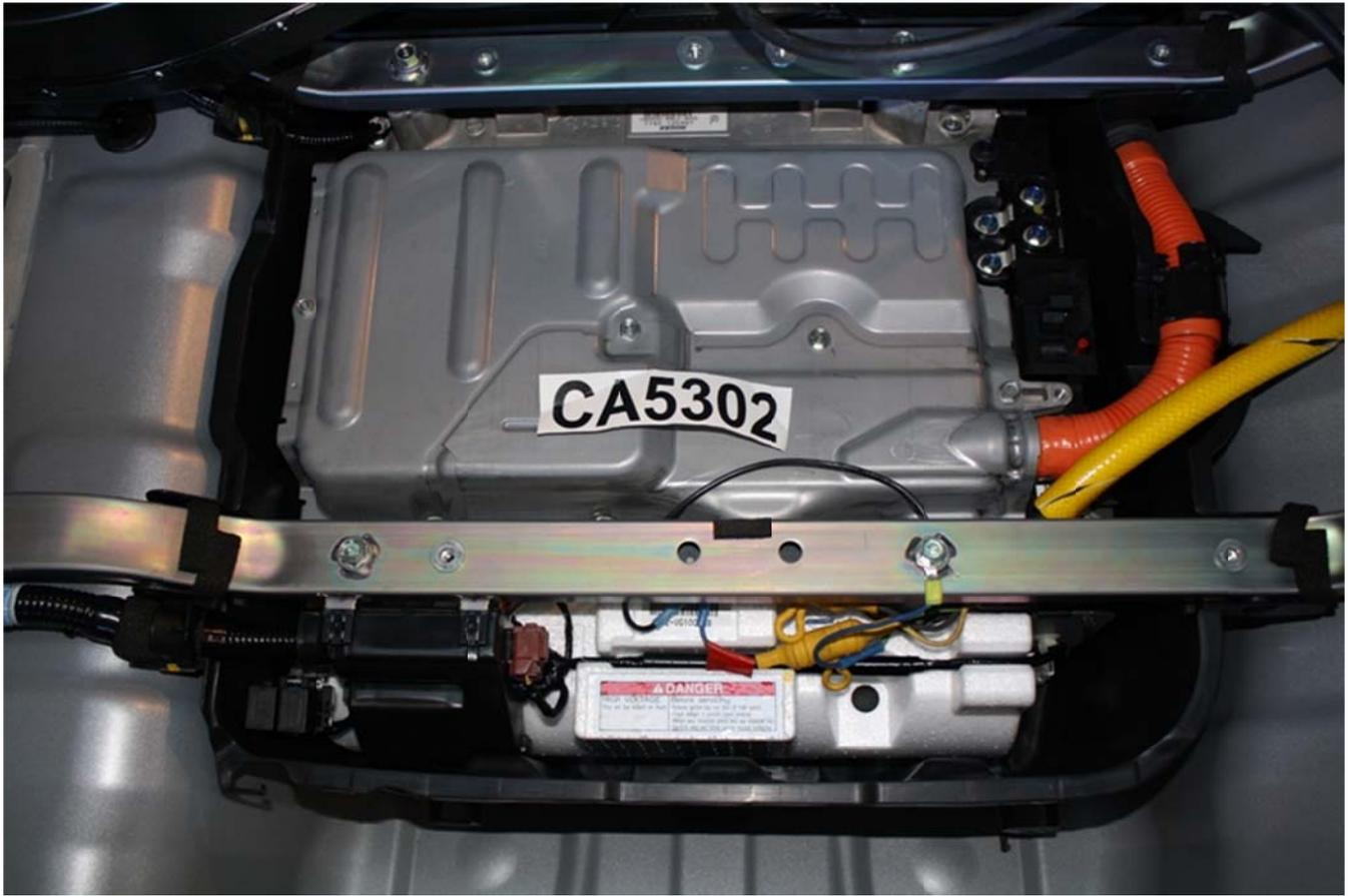
**Figure A-41: Pre-Test Battery Venting System View**
