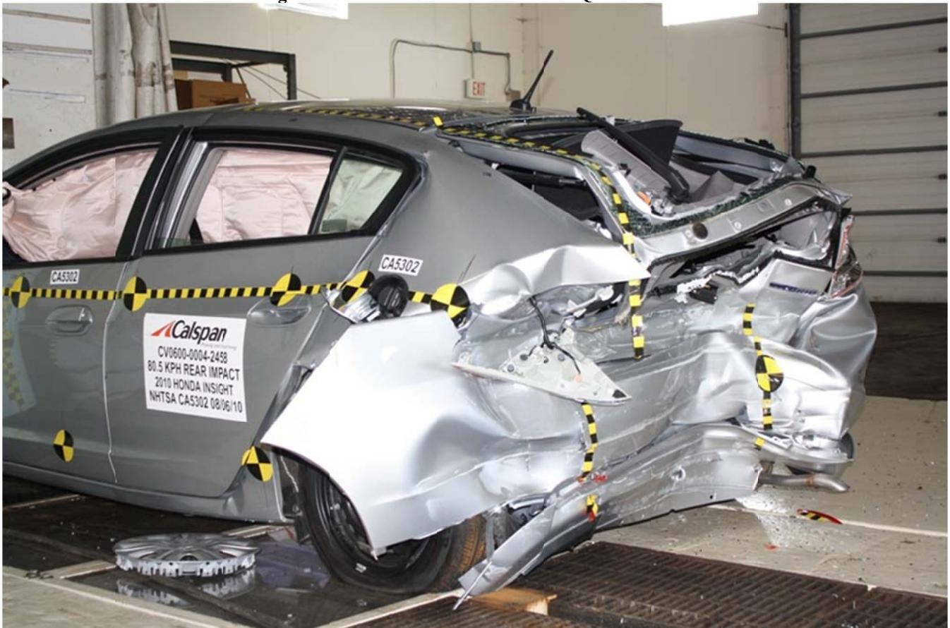
**Figure A-18: Post-Test Left Rear Three-Quarter View**
