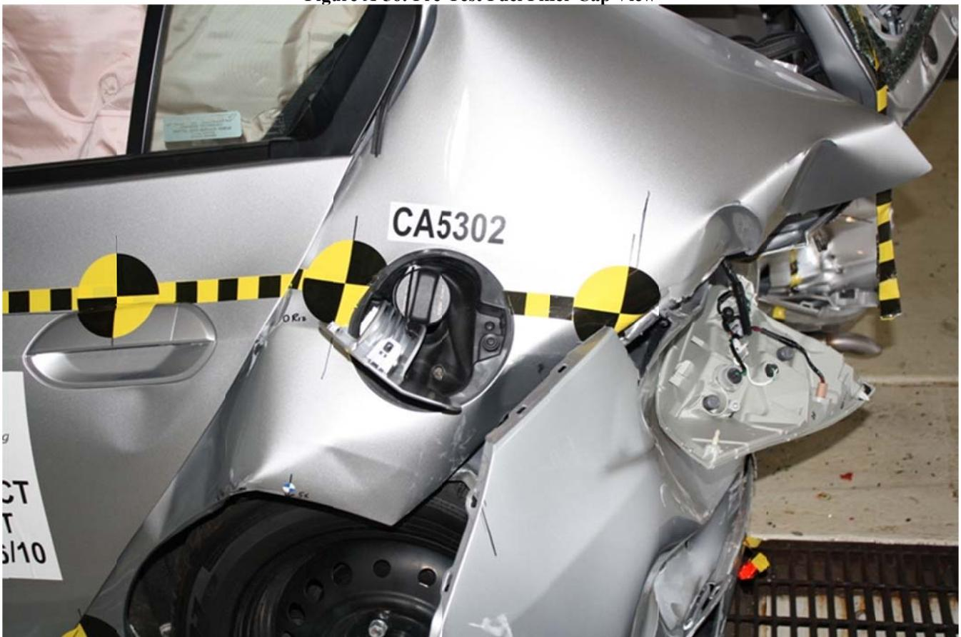
**Figure A-57: Post-Test Fuel Filler Cap View**
