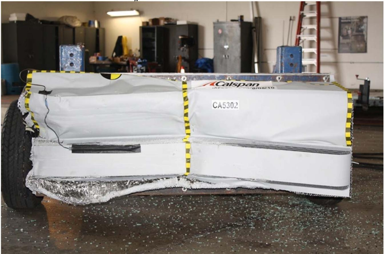
**Figure A-24: Post-Test MDB Front View**
