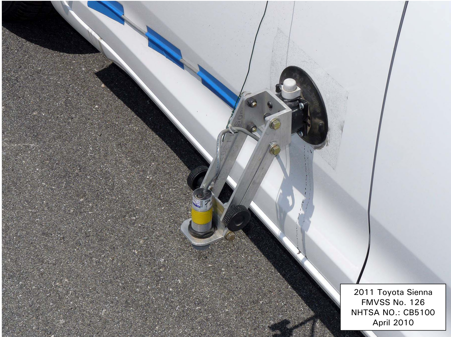
Figure 5.12. Ultrasonic Height Sensor Mounted on Left Side of Vehicle for Determining Body Roll Angle
