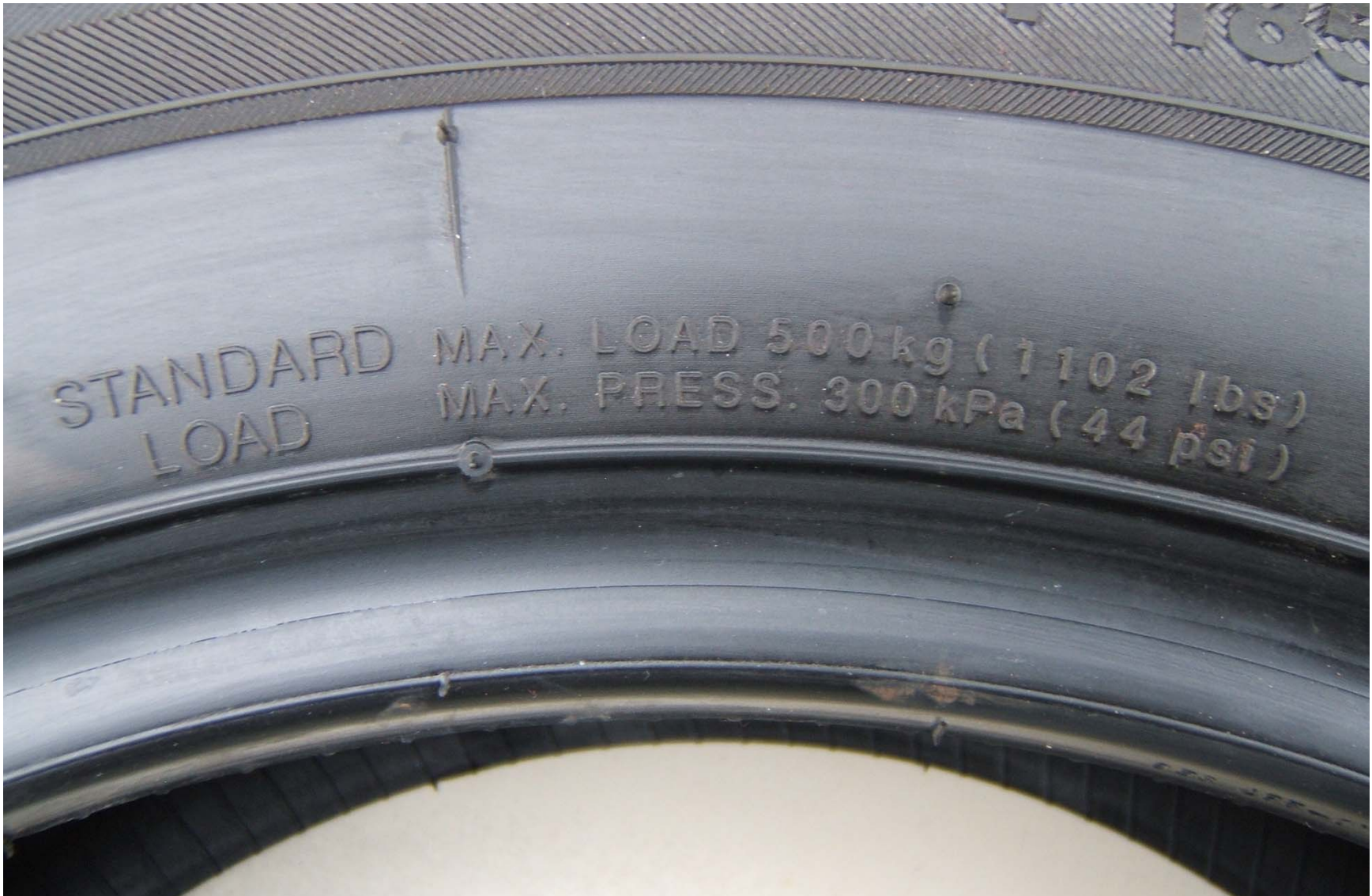
FIGURE 5.8 TIRE SHOWING MAX LOAD RATING AND MAX INFLATION PRESSURE
