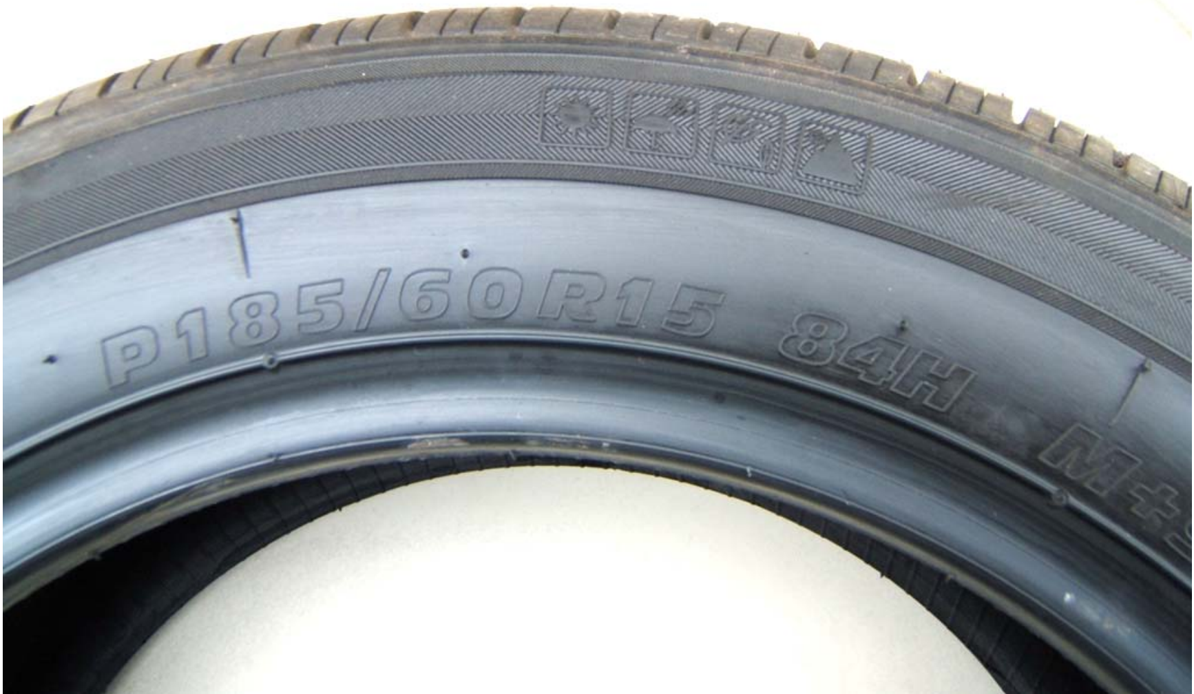
FIGURE 5.7 TIRE SHOWING SIZE, LOAD INDEX, AND SPEED SYMBOL
