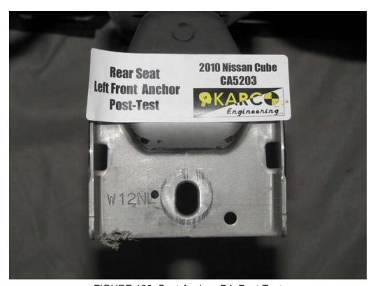
FIGURE 126. Seat Anchor, P4, Post-Test
