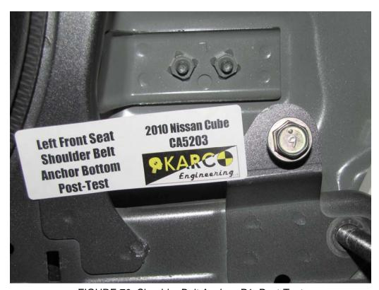
FIGURE 70. Shoulder Belt Anchor, P1, Post-Test
