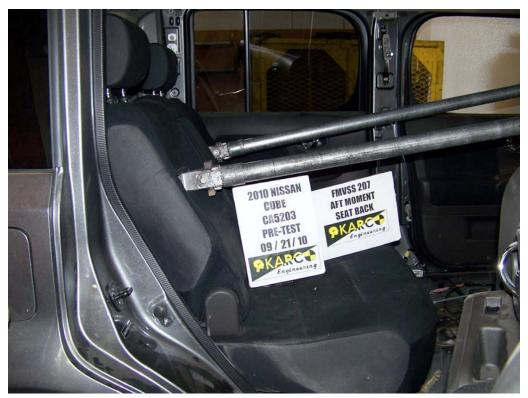
FIGURE 29. Aft Moment on Seat Back, P2, Pre-Test
