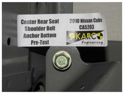
FIGURE 141. Shoulder Belt Anchor, P6, Pre-Test
