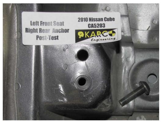
FIGURE 64. Floor Pan Anchor, P1, Post-Test
