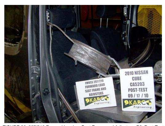
FIGURE 26. 207/210 Forward Load on Seat Frame and Adjusters, P2, Post-Test
