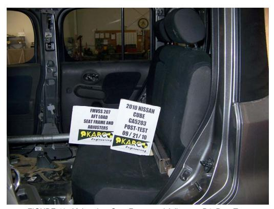
FIGURE 40. Aft Load on Seat Frame and Adjusters, P4, Post-Test
