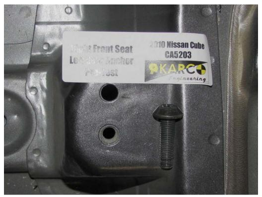
FIGURE 87. Floor Pan Anchor, P2, Pre-Test
