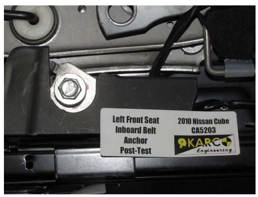
FIGURE 74. Belt Anchor, P1, Post-Test
