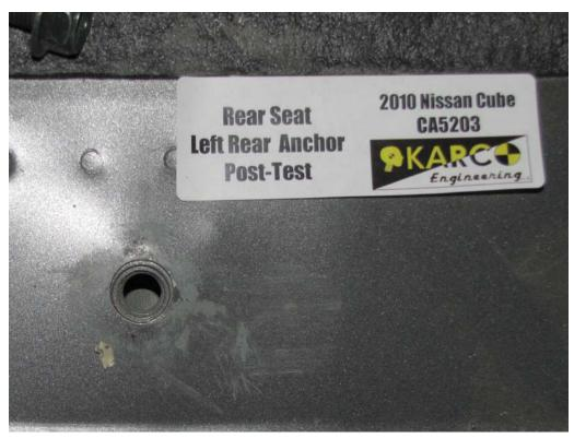
FIGURE 128. Floor Pan Anchor, P4, Post-Test
