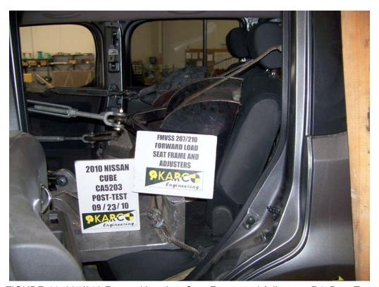
FIGURE 44. 207/210 Forward Load on Seat Frame and Adjusters, P4, Post-Test
