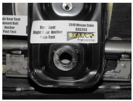
FIGURE 114. Seat Anchor, P3, Post-Test
