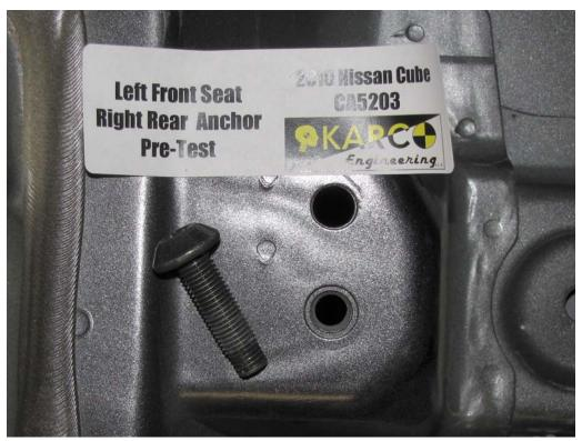
FIGURE 63. Floor Pan Anchor, P1, Pre-Test
