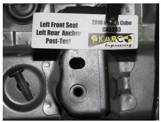
FIGURE 60. Floor Pan Anchor, P1, Post-Test
