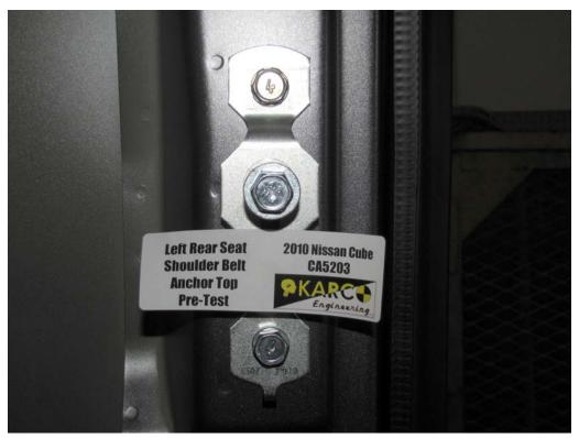
FIGURE 131. Shoulder Belt Anchor, P4, Pre-Test
