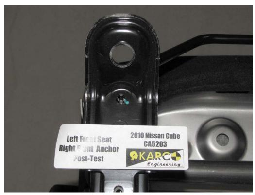
FIGURE 58. Seat Anchor, P1, Post-Test
