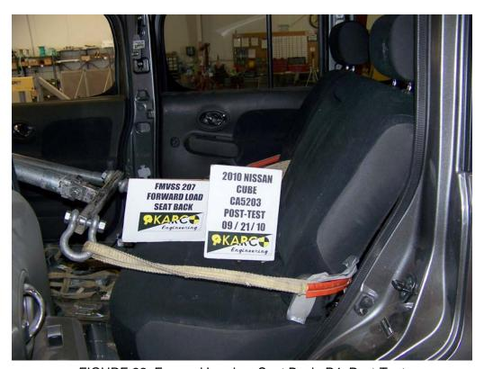
FIGURE 32. Forward Load on Seat Back, P4, Post-Test
