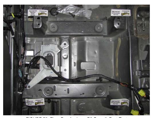
FIGURE 76. Floor Pan Anchors, P2 Overall, Post-Test
