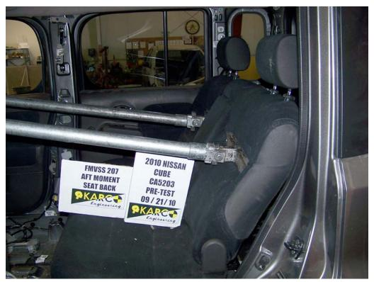
FIGURE 27. Aft Moment on Seat Back, P1, Pre-Test
