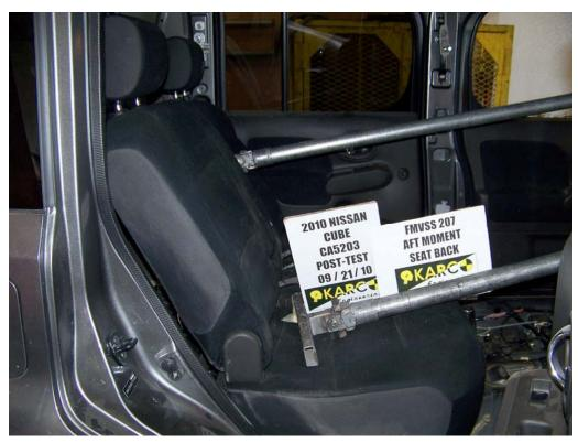
FIGURE 30. Aft Moment on Seat Back, P2, Post-Test
