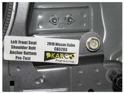
FIGURE 69. Shoulder Belt Anchor, P1, Pre-Test
