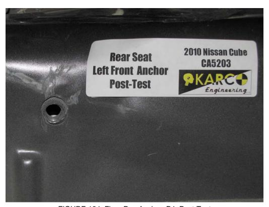
FIGURE 124. Floor Pan Anchor, P4, Post-Test
