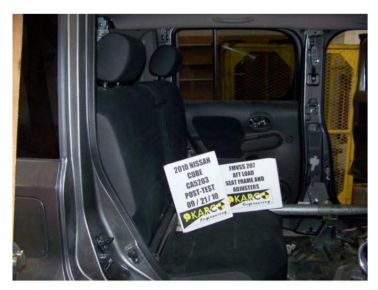
FIGURE 42. Aft Load on Seat Frame and Adjusters, P3, Post-Test
