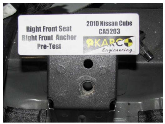
FIGURE 83. Floor Pan Anchor, P2, Pre-Test
