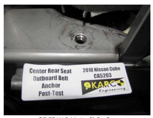
FIGURE 144. Belt Anchor, P6, Post-Test
