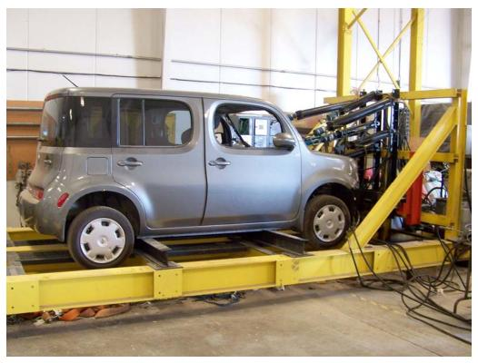
FIGURE 7. Vehicle Mounted in Test Fixture
