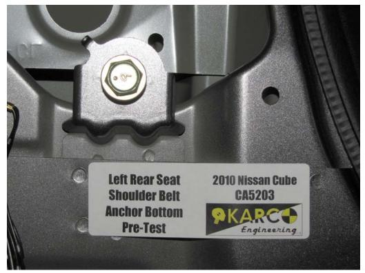
FIGURE 133. Shoulder Belt Anchor, P4, Pre-Test
