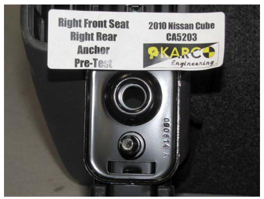
FIGURE 93. Seat Anchor, P2, Pre-Test
