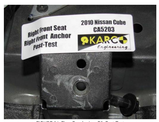
FIGURE 84. Floor Pan Anchor, P2, Post-Test
