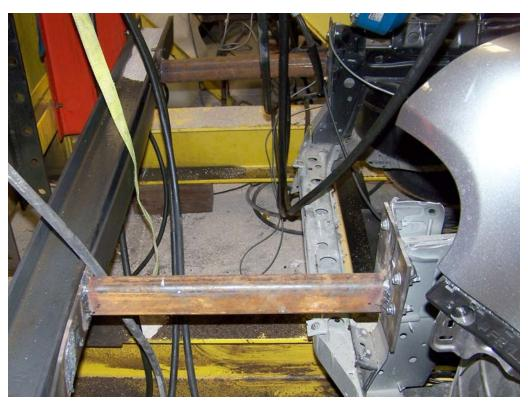
FIGURE 10. Vehicle Mounted in Test Fixture
