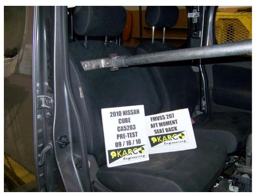
FIGURE 13. Aft Moment on Seat Back, P2, Pre-Test
