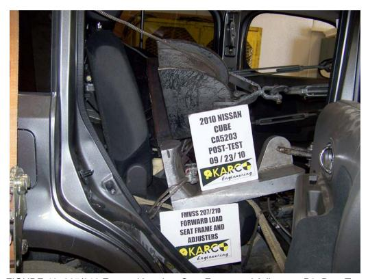
FIGURE 46. 207/210 Forward Load on Seat Frame and Adjusters, P3, Post-Test
