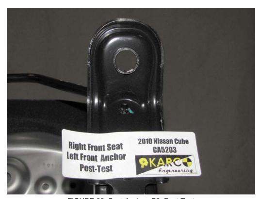
FIGURE 82. Seat Anchor, P2, Post-Test
