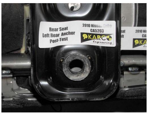
FIGURE 130. Seat Anchor, P4, Post-Test
