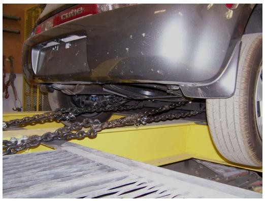
FIGURE 9. Vehicle Mounted in Test Fixture
