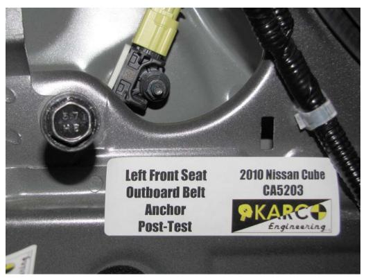
FIGURE 72. Belt Anchor, P1, Post-Test
