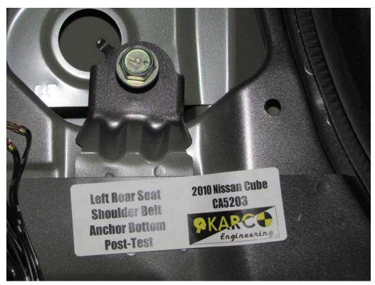
FIGURE 134. Shoulder Belt Anchor, P4, Post-Test
