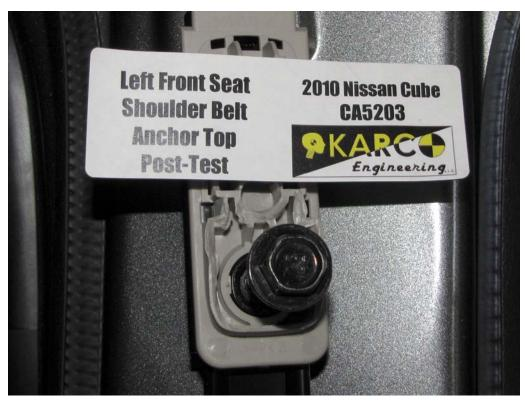
FIGURE 68. Shoulder Belt Anchor, P1, Post-Test
