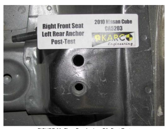
FIGURE 88. Floor Pan Anchor, P2, Post-Test
