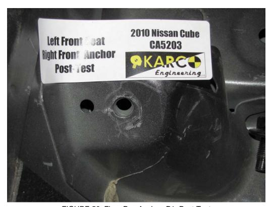
FIGURE 56. Floor Pan Anchor, P1, Post-Test
