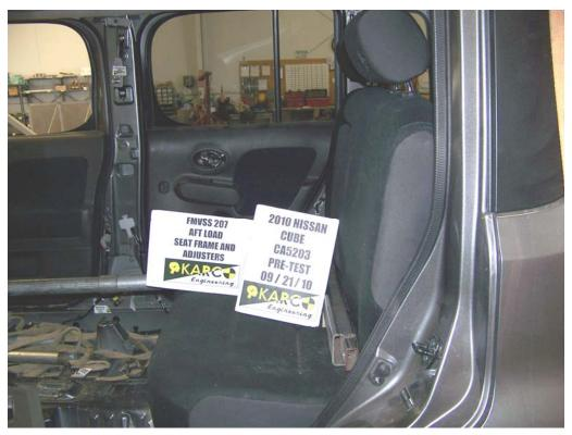
FIGURE 39. Aft Load on Seat Frame and Adjusters, P4, Pre-Test
