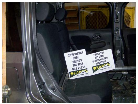
FIGURE 41. Aft Load on Seat Frame and Adjusters, P3, Pre-Test
