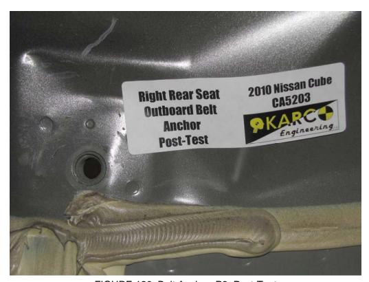
FIGURE 120. Belt Anchor, P3, Post-Test
