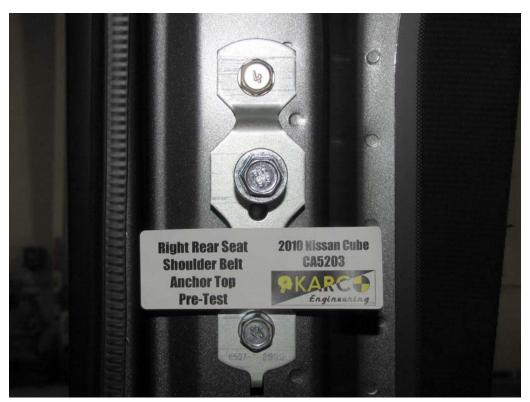
FIGURE 115. Belt Anchor, P3, Pre-Test
