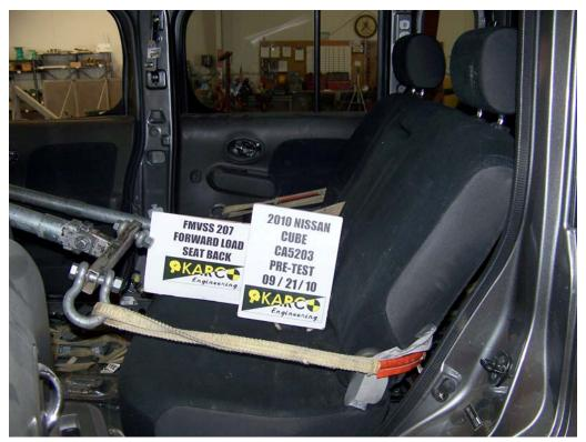
FIGURE 31. Forward Load on Seat Back, P4, Pre-Test
