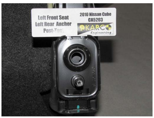
FIGURE 62. Seat Anchor, P1, Post-Test
