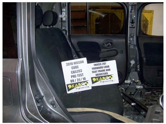
FIGURE 37. Forward Load on Seat Frame and Adjusters, P3, Pre-Test
