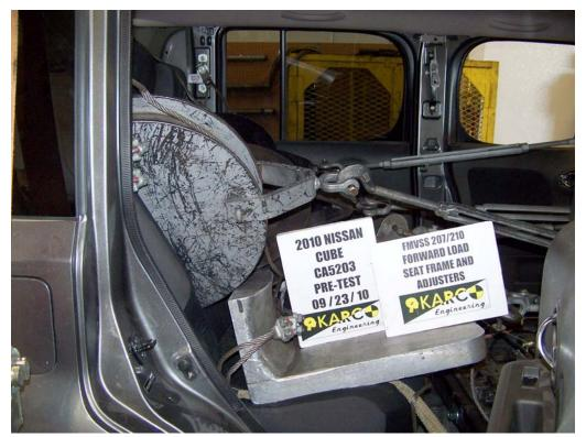
FIGURE 45. 207/210 Forward Load on Seat Frame and Adjusters, P3, Pre-Test
