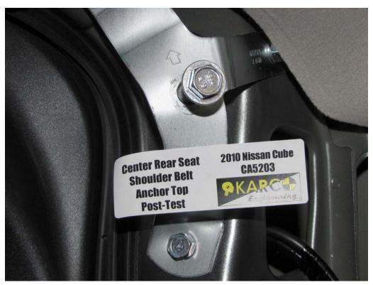
FIGURE 140. Shoulder Belt Anchor, P6, Post-Test
