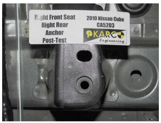
FIGURE 92. Floor Pan Anchor, P2, Post-Test
