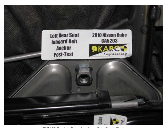
FIGURE 138. Belt Anchor, P4, Post-Test
