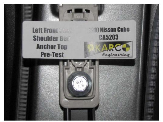
FIGURE 67. Shoulder Belt Anchor, P1, Pre-Test
