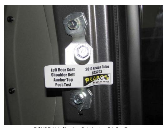
FIGURE 132. Shoulder Belt Anchor, P4, Pre-Test
