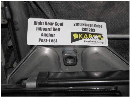
FIGURE 122. Belt Anchor, P3, Post-Test
