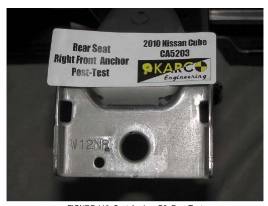
FIGURE 110. Seat Anchor, P3, Post-Test
