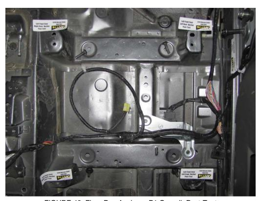
FIGURE 48. Floor Pan Anchors, P1 Overall, Post-Test
