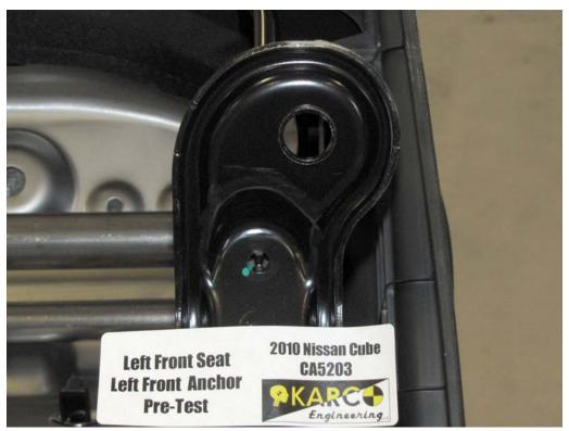
FIGURE 53. Seat Anchor, P1, Pre-Test
