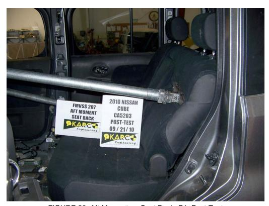
FIGURE 28. Aft Moment on Seat Back, P1, Post-Test
