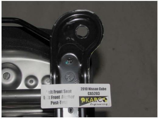
FIGURE 54. Seat Anchor, P1, Post-Test
