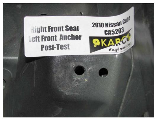
FIGURE 80. Floor Pan Anchor, P2, Post-Test
