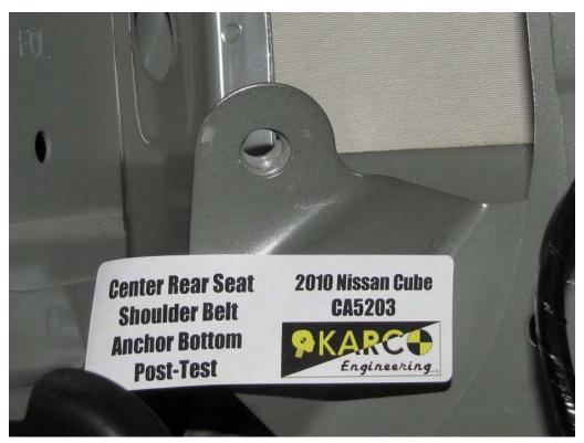
FIGURE 142. Shoulder Belt Anchor, P6, Post-Test
