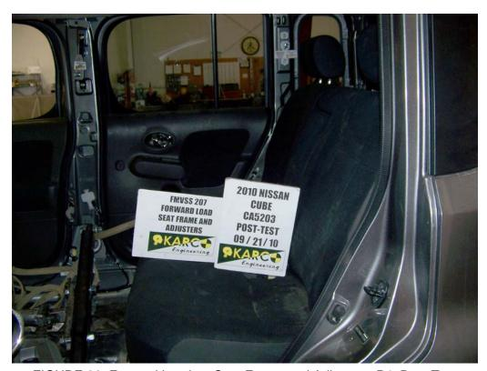
FIGURE 36. Forward Load on Seat Frame and Adjusters, P4, Post-Test
