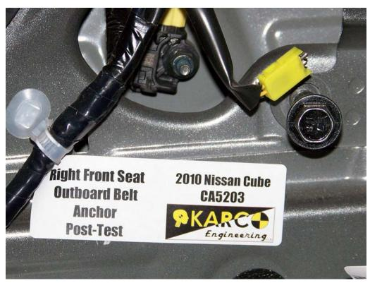
FIGURE 100. Belt Anchor, P2, Post-Test
