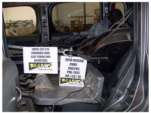
FIGURE 43. 207/210 Forward Load on Seat Frame and Adjusters, P4, Pre-Test
