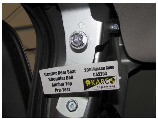
FIGURE 139. Shoulder Belt Anchor, P6, Pre-Test
