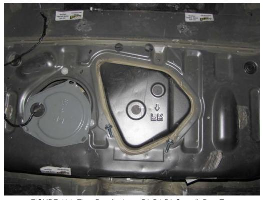
FIGURE 104. Floor Pan Anchors, P3-P4-P6 Overall, Post-Test
