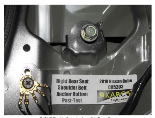
FIGURE 118. Belt Anchor, P3, Post-Test
