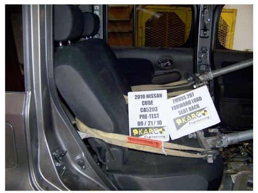
FIGURE 33. Forward Load on Seat Back, P3, Pre-Test
