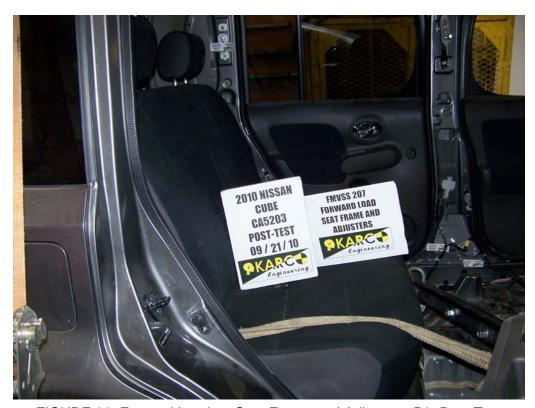
FIGURE 38. Forward Load on Seat Frame and Adjusters, P3, Post-Test
