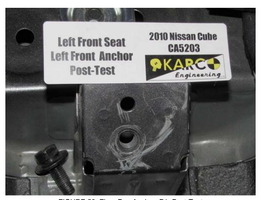
FIGURE 52. Floor Pan Anchor, P1, Post-Test
