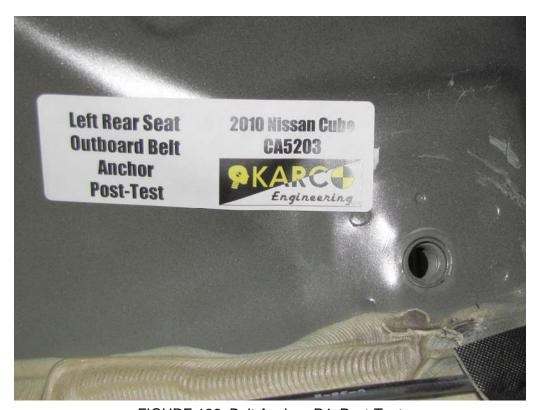
FIGURE 136. Belt Anchor, P4, Post-Test
