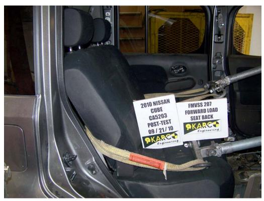
FIGURE 34. Forward Load on Seat Back, P3, Post-Test
