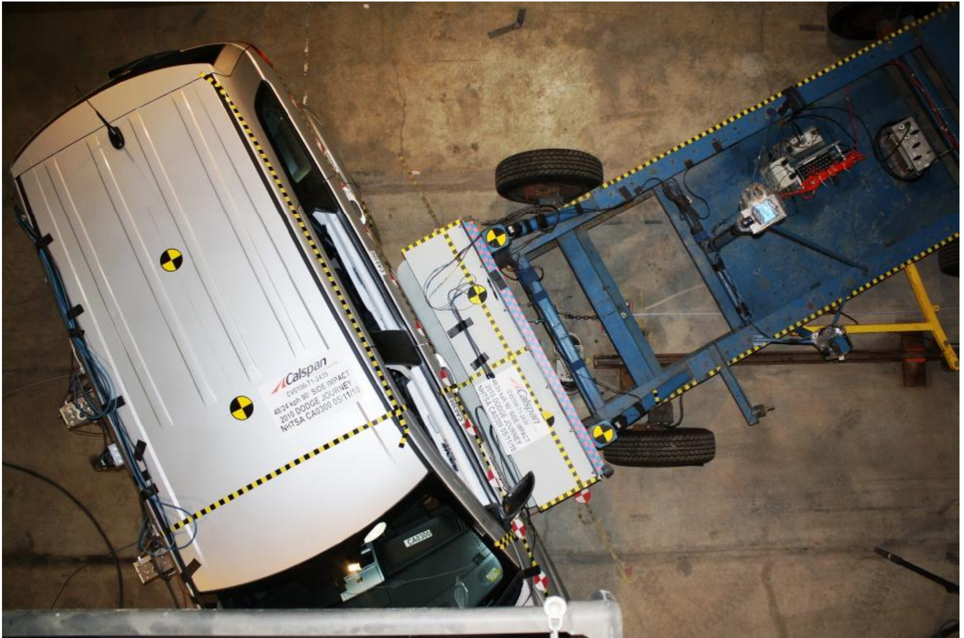
Figure A-15 Pre-Test Overhead View of Aligned MDB and Vehicle at Impact Location
