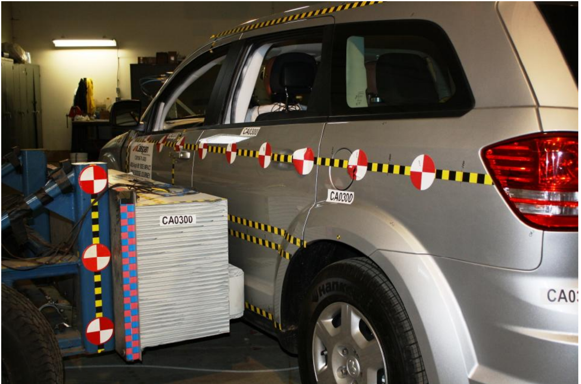
Figure A-23 Pre-Test Right Side View of Aligned MDB and Vehicle
