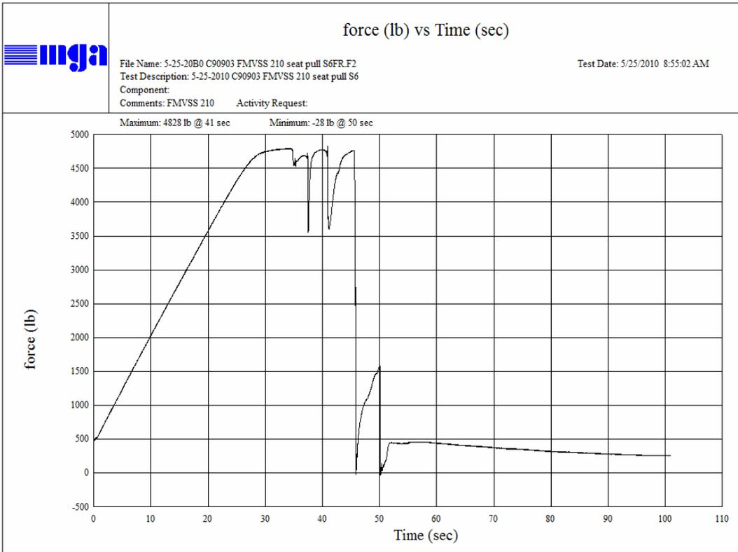
Seat S6 Anchorage Type 1 FMVSS 210
