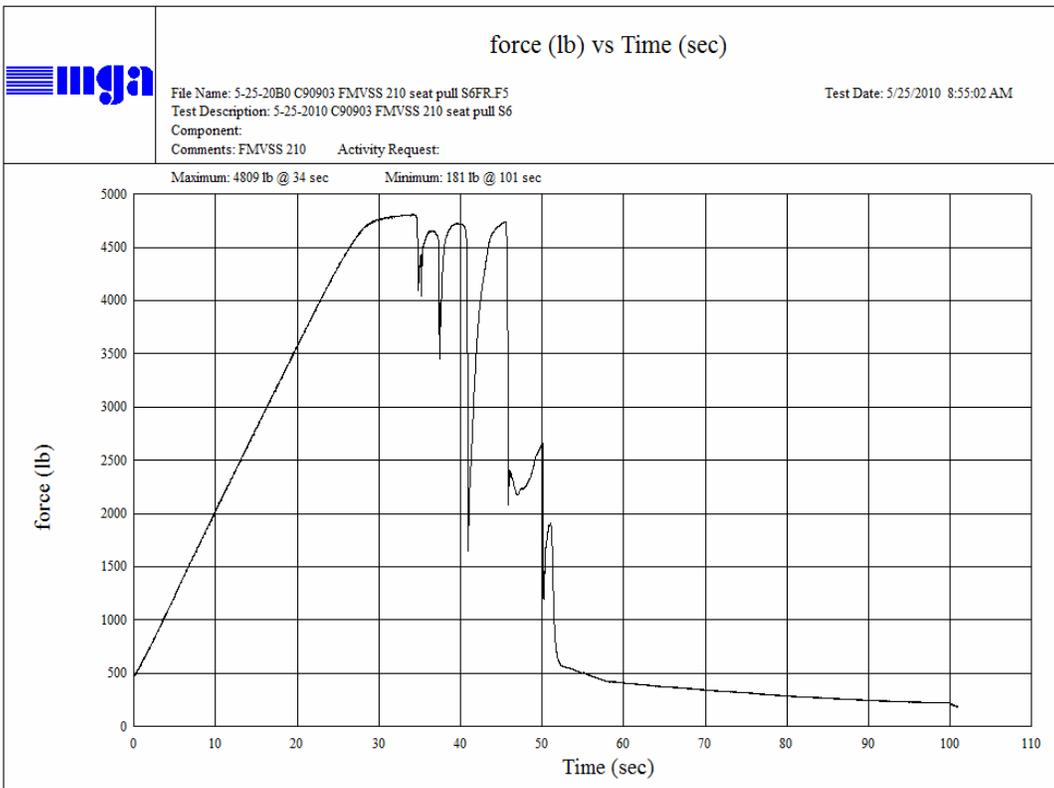
Seat S6 Anchorage Type 1 FMVSS 210
