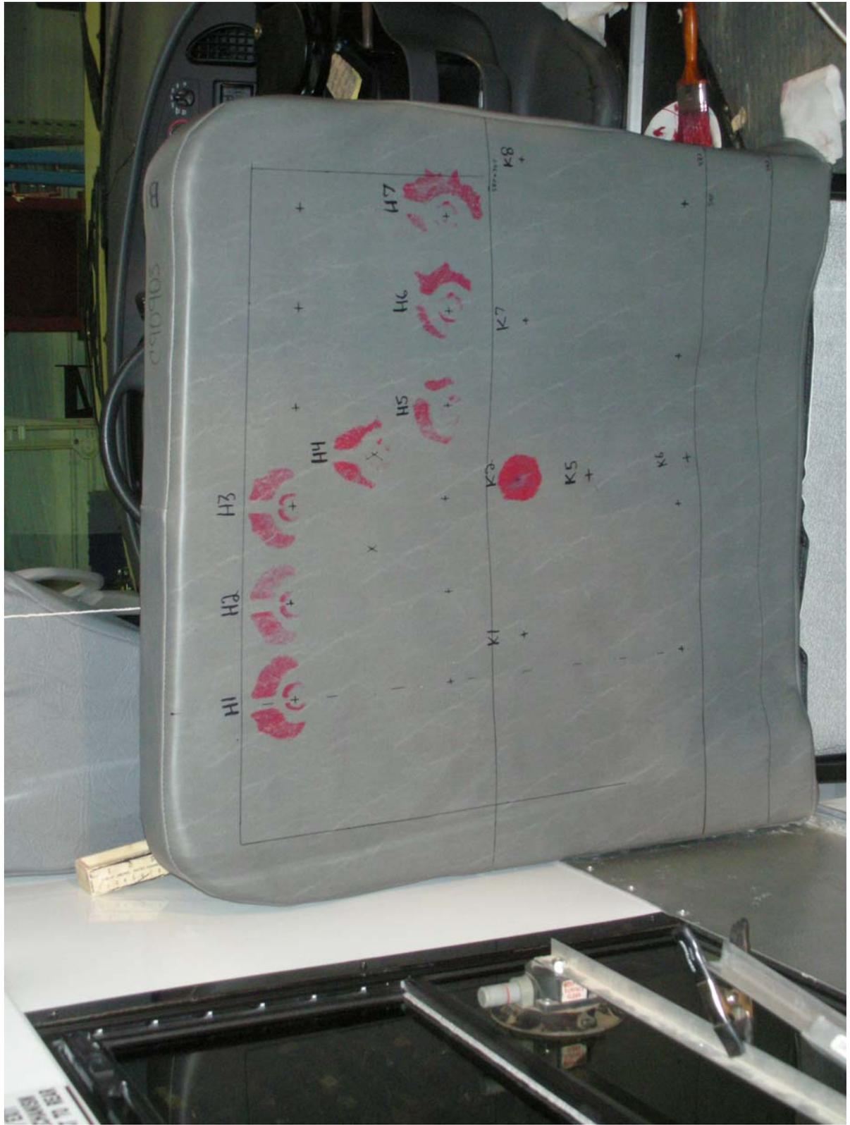
Post-Test of Head and Knee Impact Locations on Seat B1
