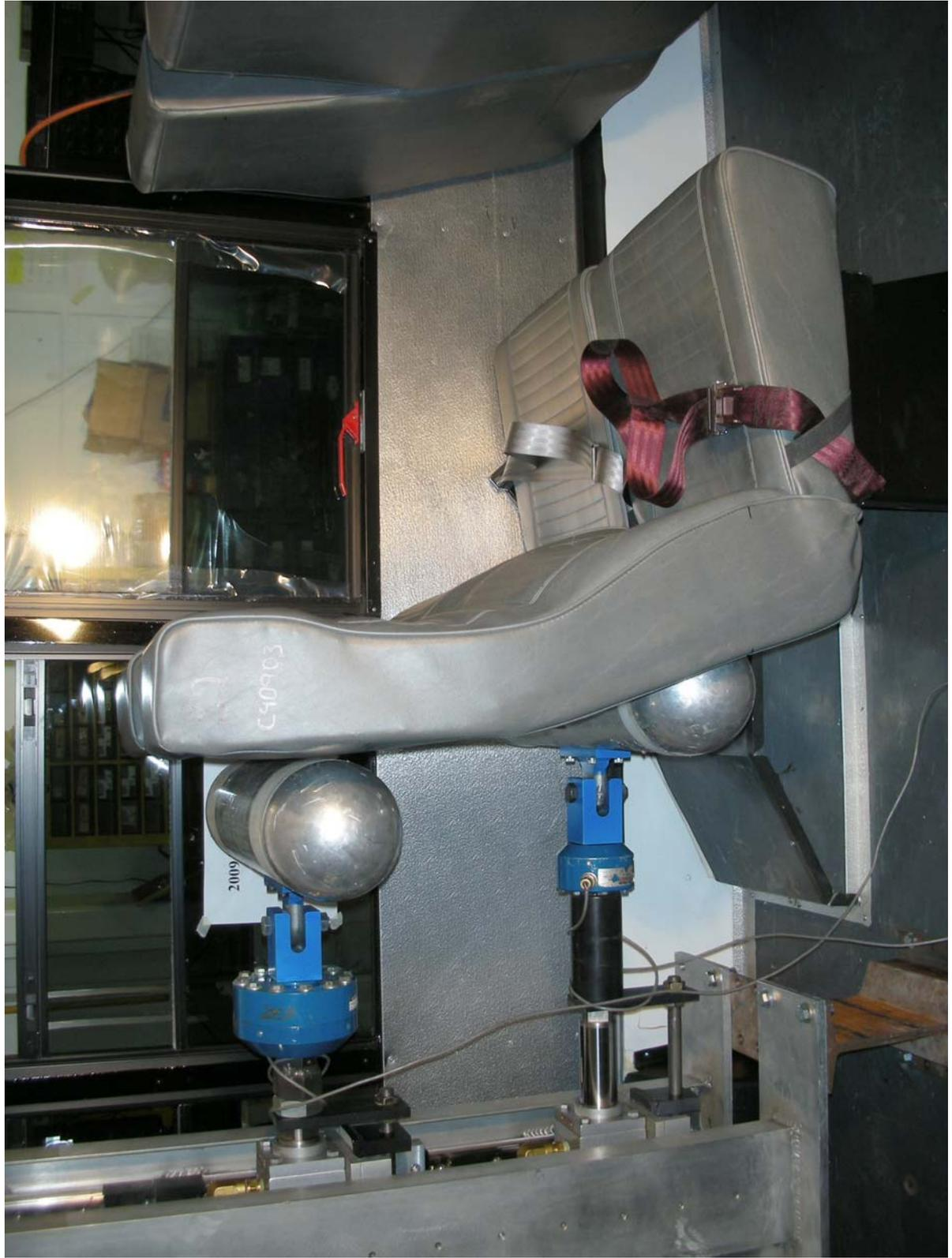
Pre-Test of Seat Back S2 Force Deflection Forward Test
