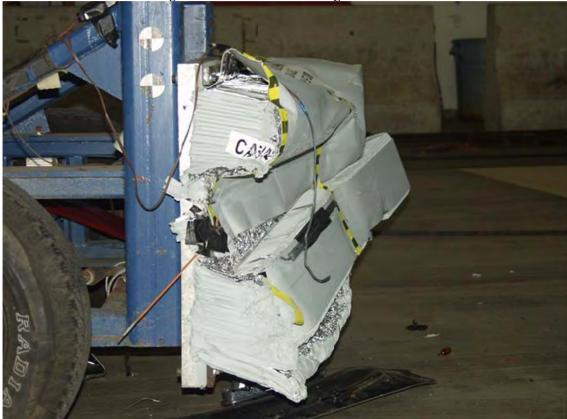
Figure A-24: Post-Test MDB Right Side View
