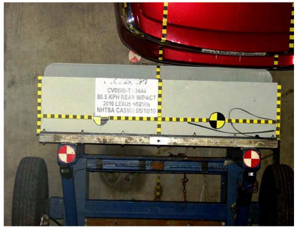
Figure A-25: Pre-Test MDB Top View
