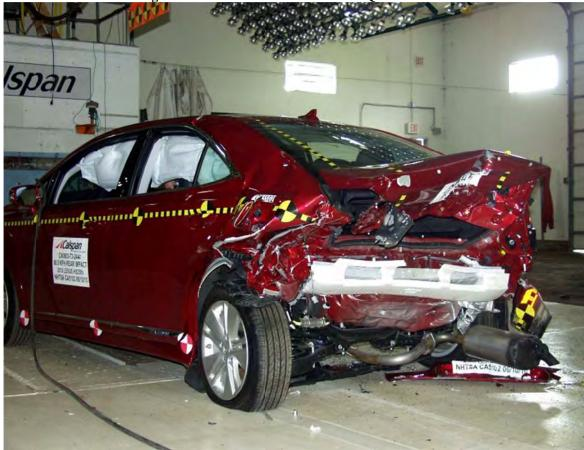
Figure A-14: Post-Test Left Rear Three-Quarter View
