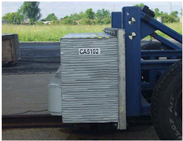
Figure A-21: Pre-Test MDB Left Side View
