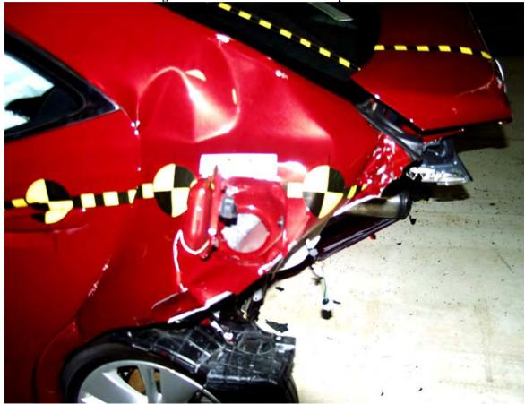
Figure A-36: Post-Test Fuel Filler Cap View
