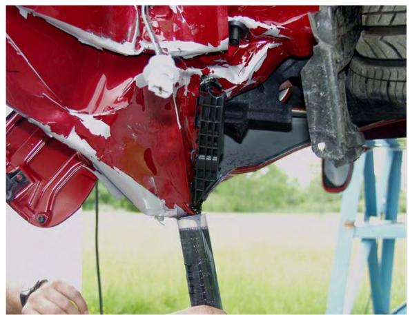
Figure A-42: leak collection at 90°
