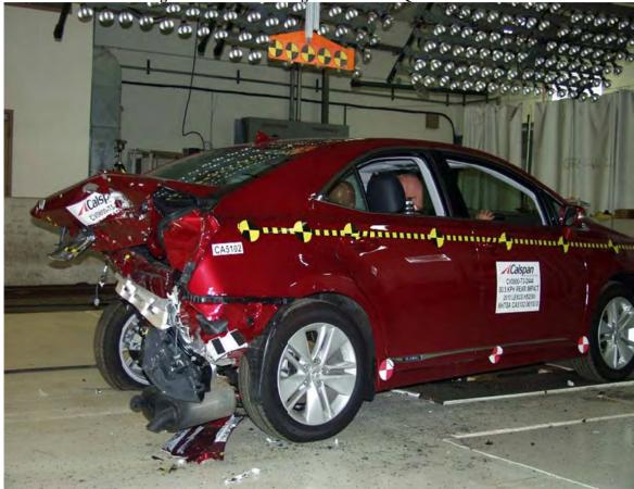
Figure A-16: Post-Test Right Rear Three-Quarter View
