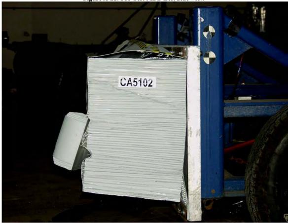
Figure A-22: Post-Test MDB Left Side View
