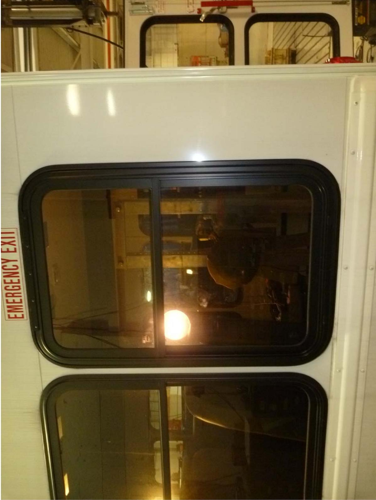
Window Retention Test of W6 Rearmost Passenger Side Lower Window Pane Pre-Test
