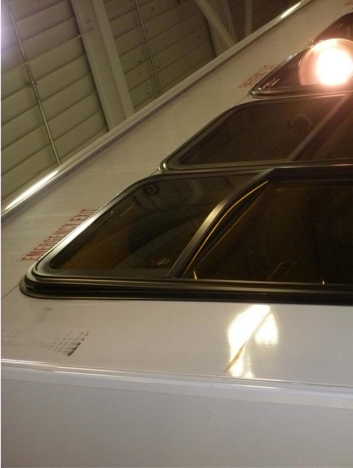
Window Retention Test of W7 Rearmost Driver Side Upper Window Pane Post-Test
