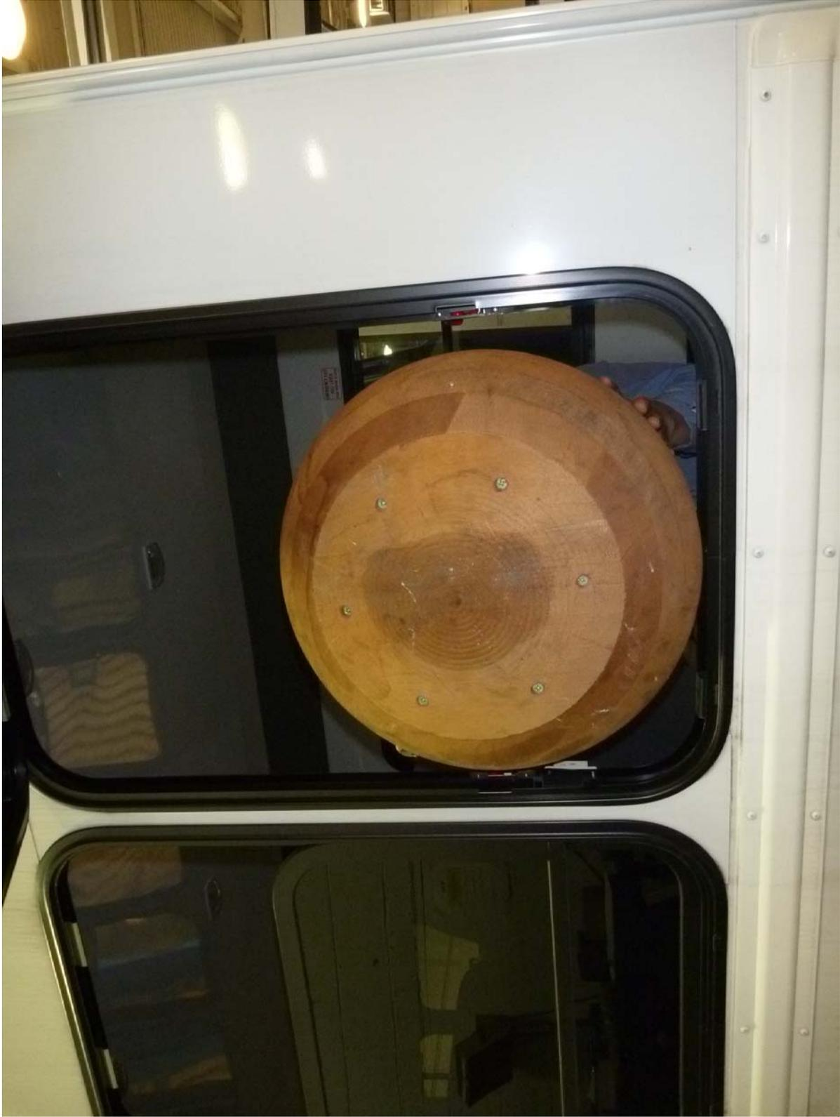
Emergency Exit Window Ellipsoid Clearance
