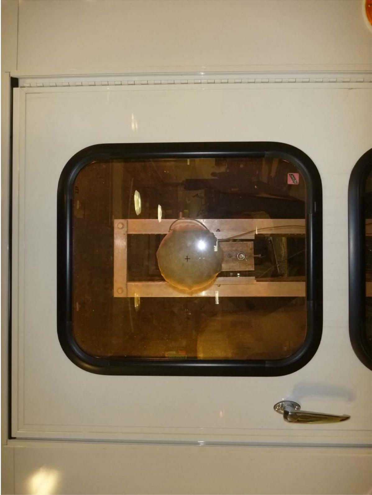
Window Retention Test of Rear Emergency Door Upper Pane Pre-Test
