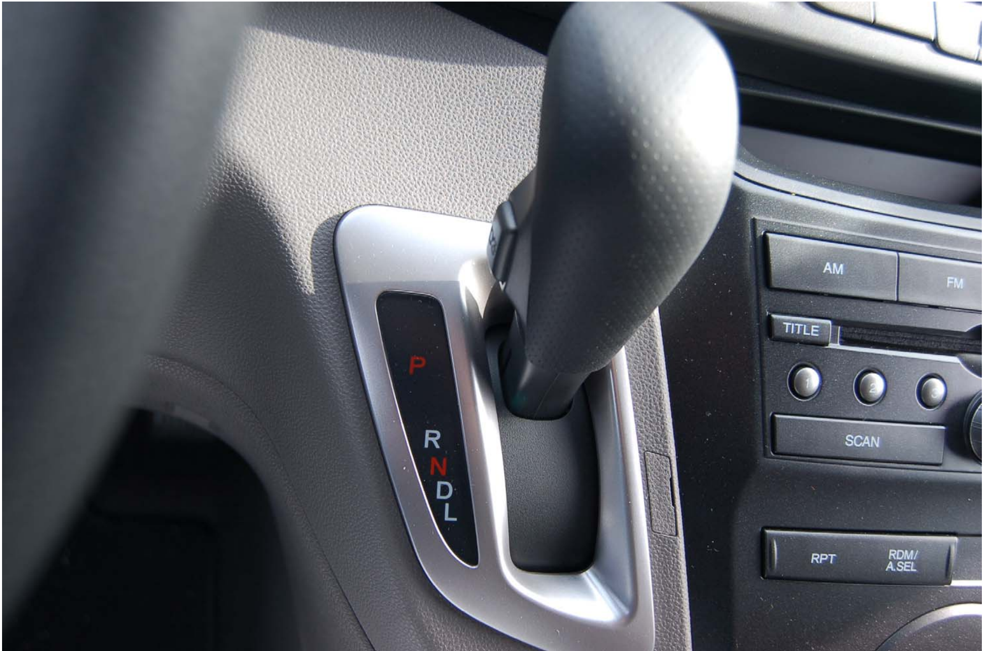
FIGURE 5.6 TRANSMISSION GEAR SELECTION CONTROL
