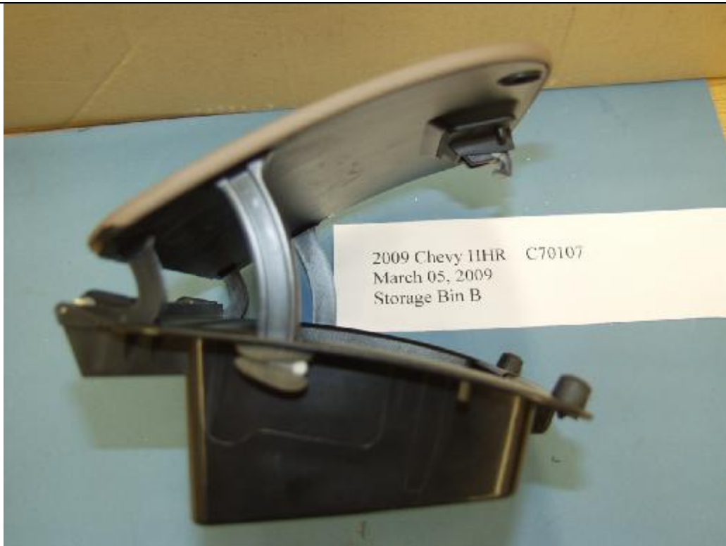
Figure A-24: INSTRUMENT PANEL STORAGE BIN B POST-TEST
