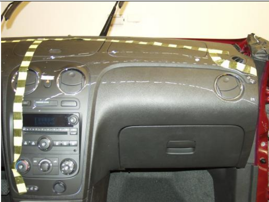
Figure A-12: DELINEATED INSTRUMENT PANEL IMPACT ZONE PRE-TEST
