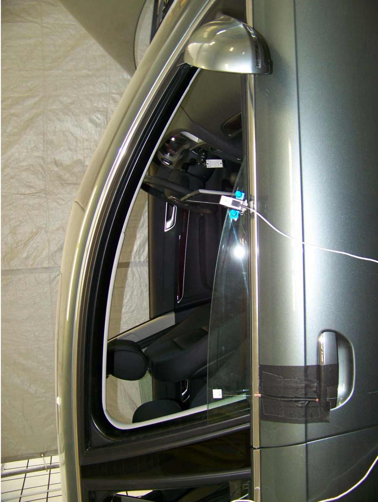
Figure 19: Right Front Window Test Set-Up Leading Edge
