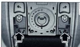
Fig. 49 Section from headliner: unscrewing the lighting unit
