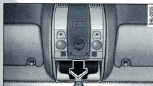
Fig. 47 Section from headliner: removing the cover
