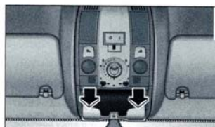
Fig. 48 Section from headliner: remove the cover for the light unit
