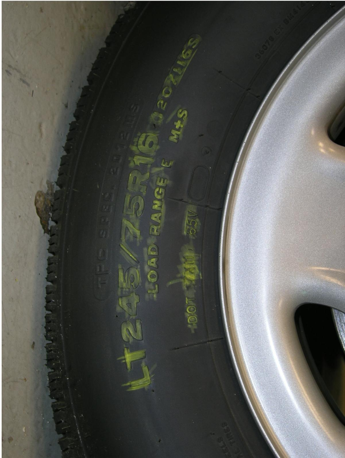
Right Front Tire DOT Serial Number, Tire Load Range Identification and Tire Size Designation
