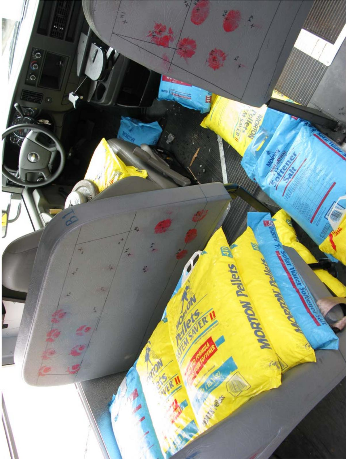
Simulated Interior Occupant Ballast
