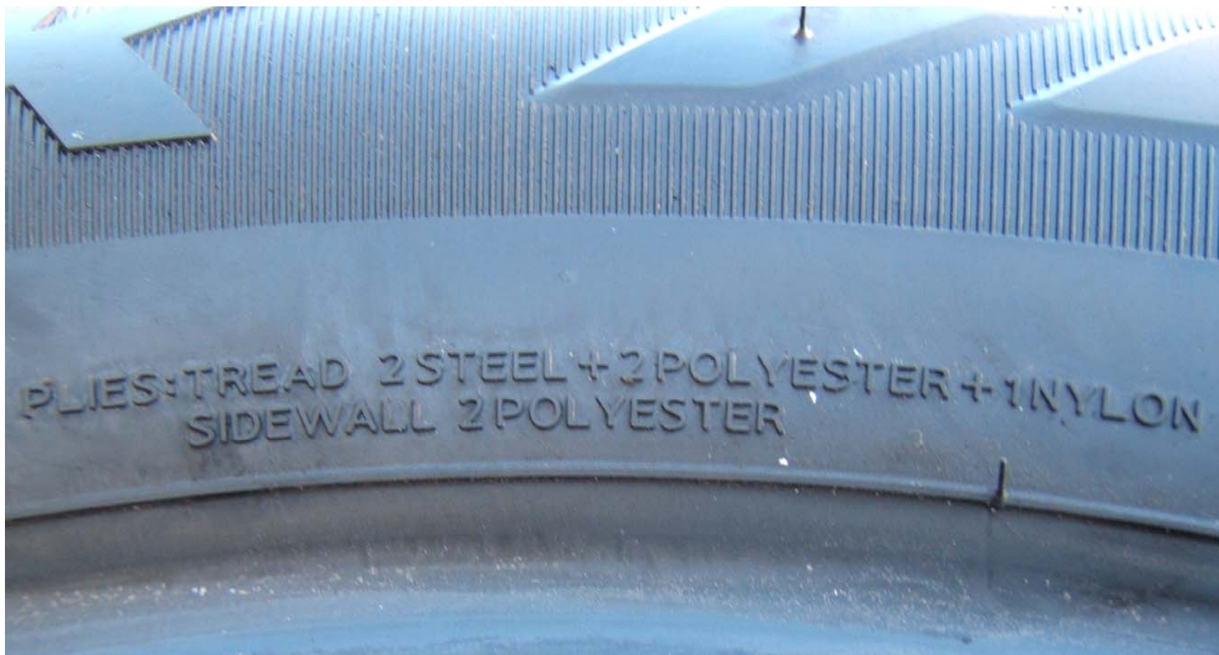
FIGURE 5.9 TIRE SHOWING SIDEWALL / TREAD CONSTRUCTION
