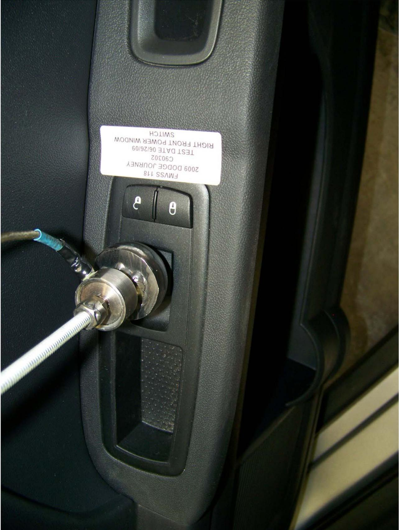
Figure 13: Sphere Test Right Front Window
