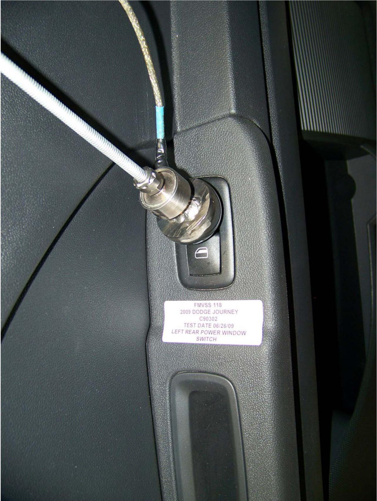
Figure 14: Sphere Test Left Rear Window
