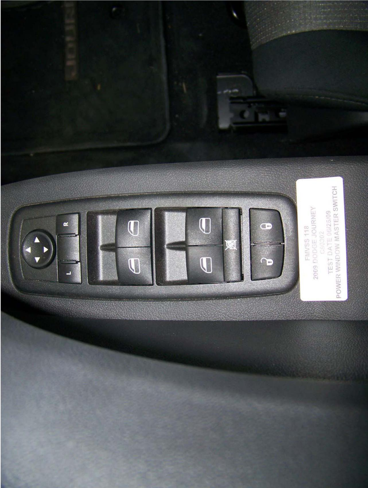
Figure 6: Left Front Master Power Window Switch
