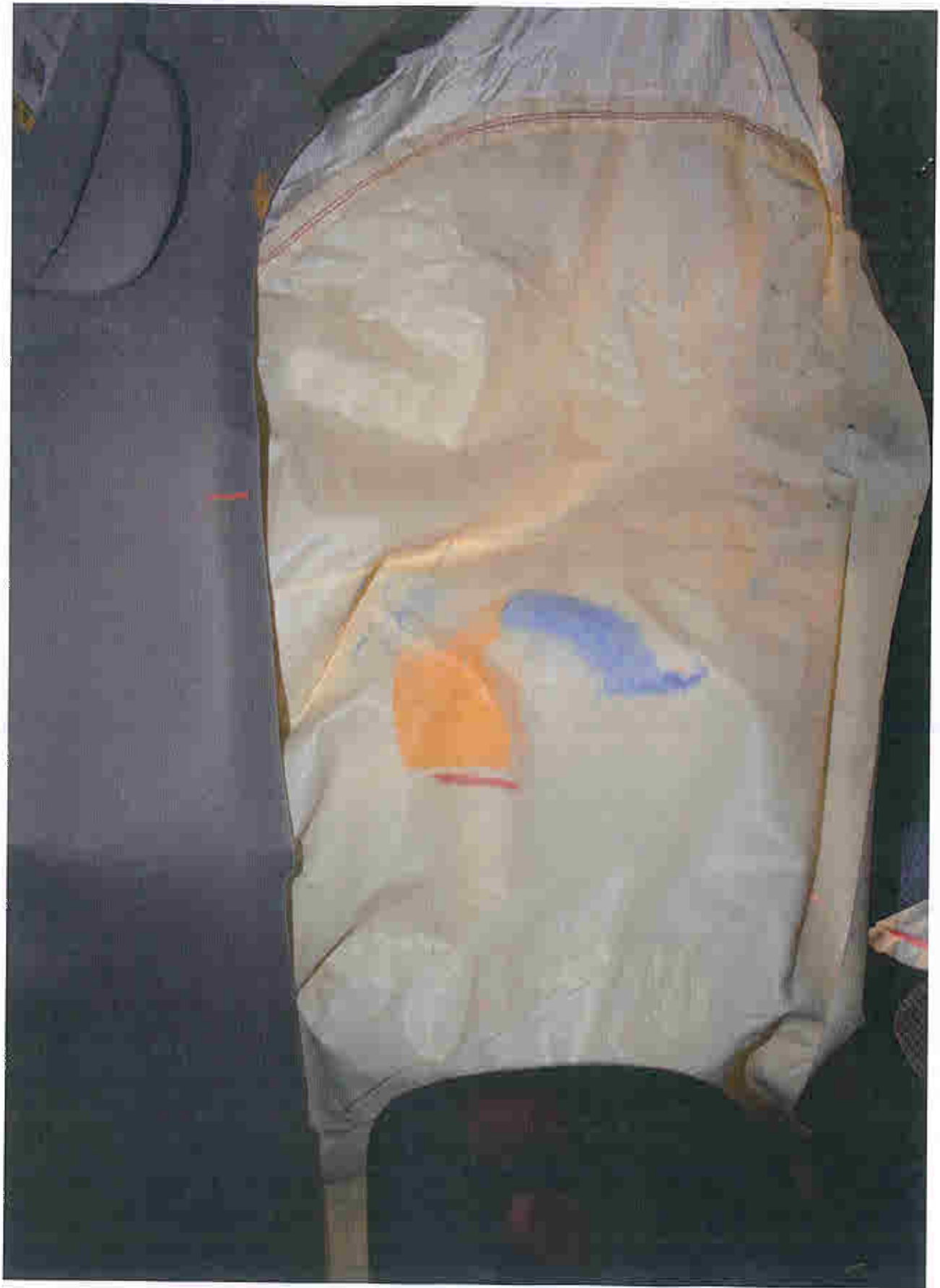
Post-Test Driver Dummy Head Contact (CAB)
