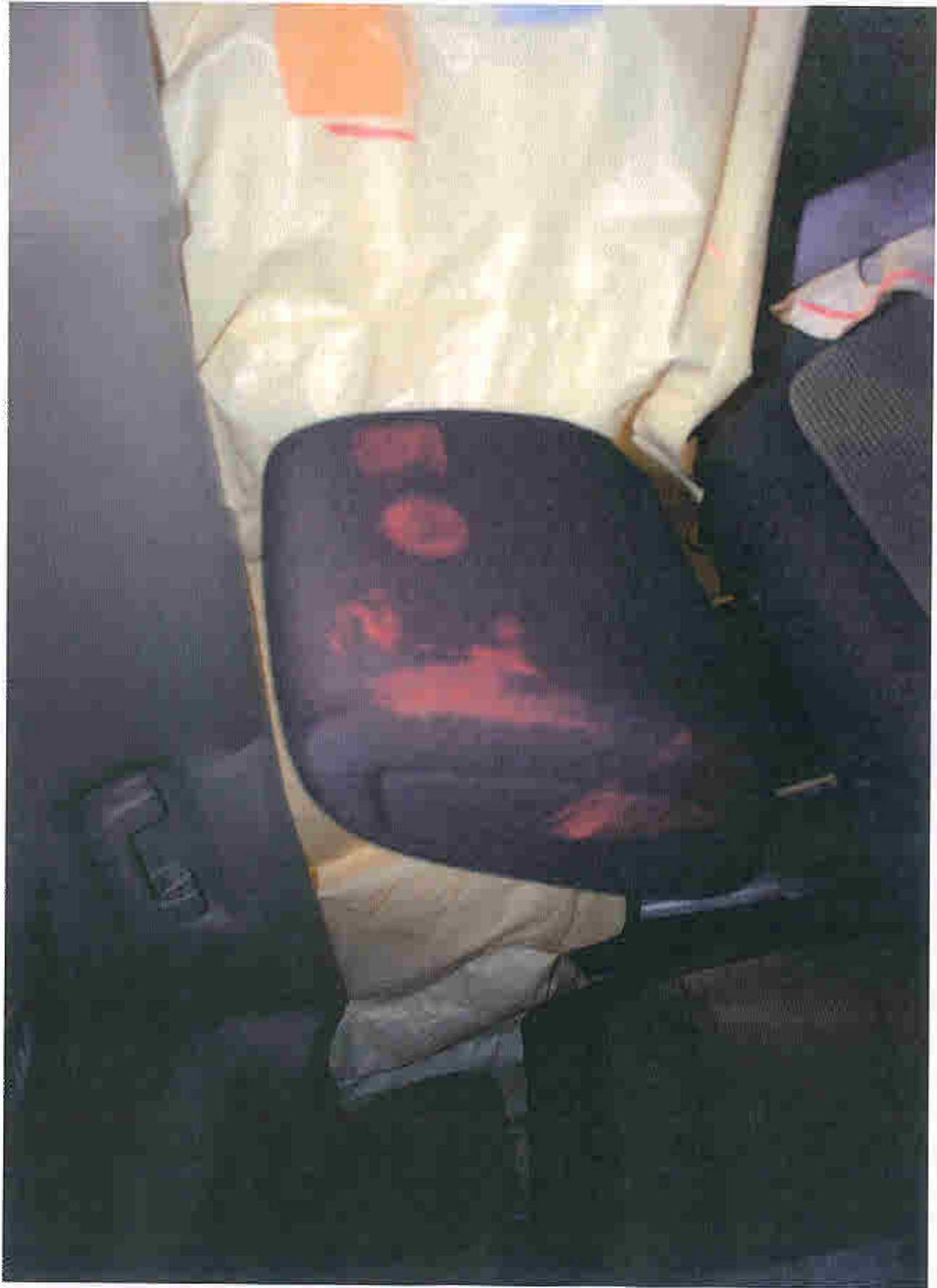
Post-Test Driver Dummy Head Contact (Headrest)
