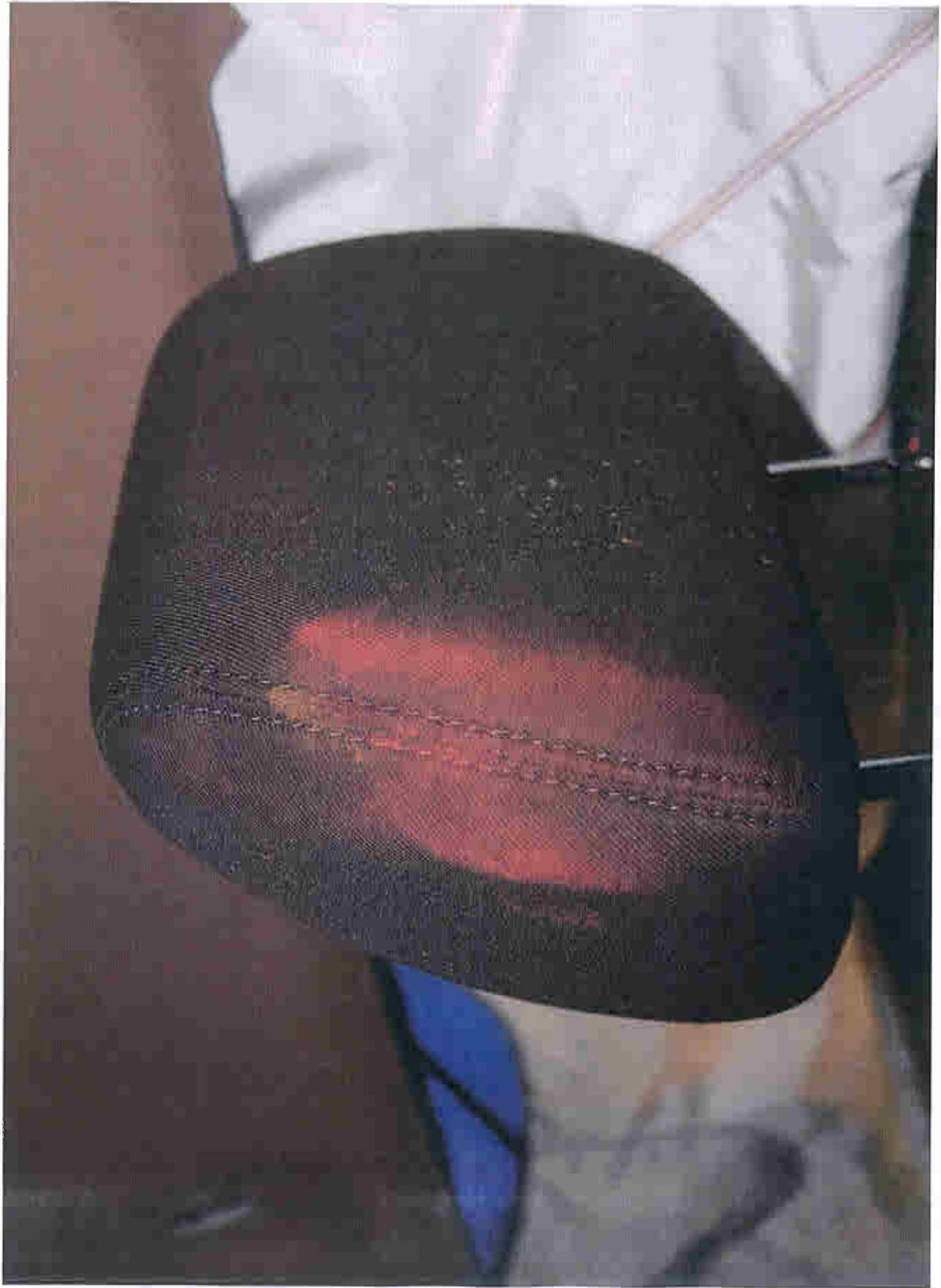
Post-Test Driver Dummy Head Contact (Headrest)
