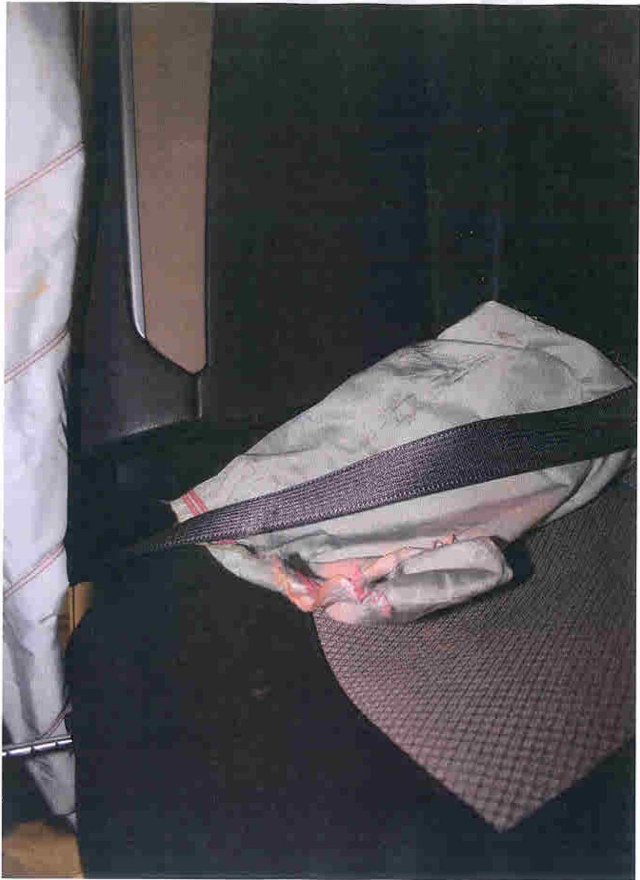
Post-Test Driver Dummy Upper Thorax Contact
