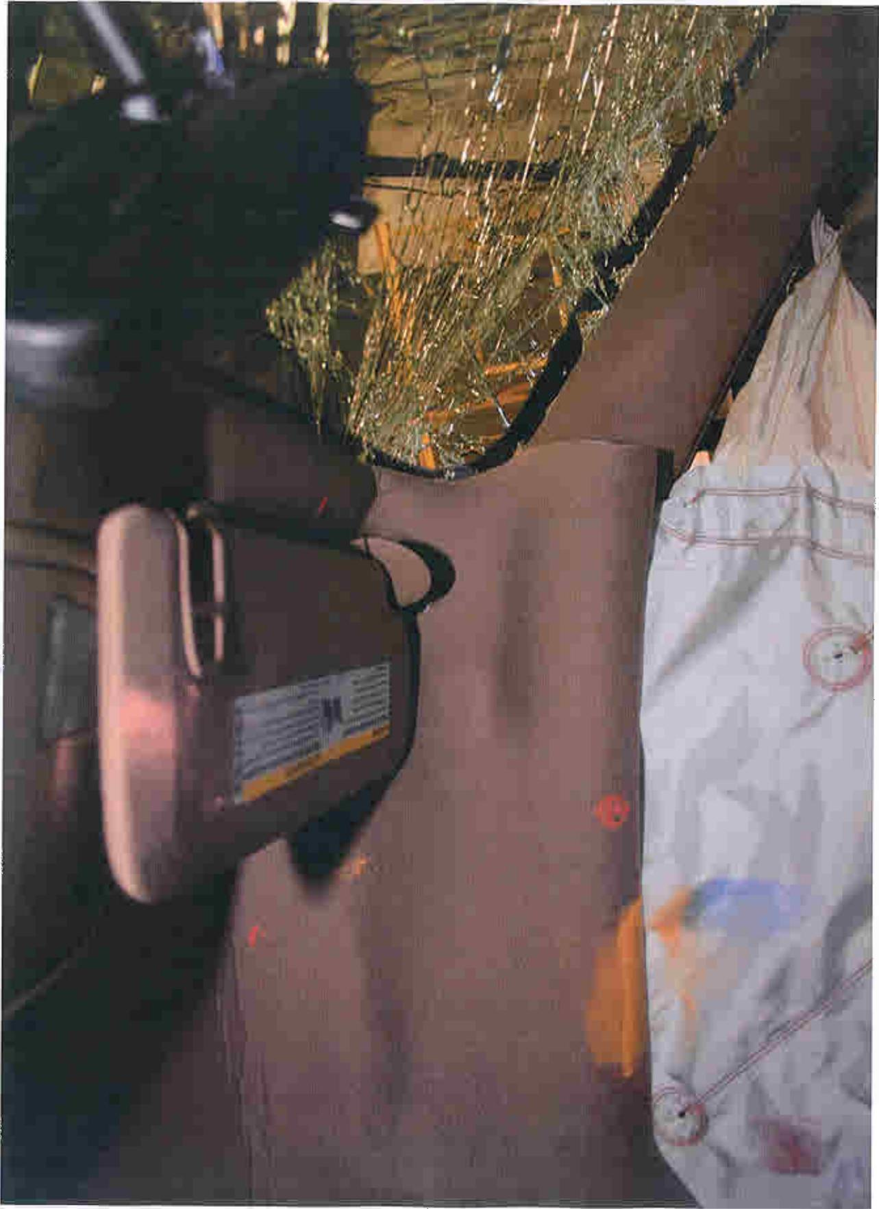
Post-Test Driver Dummy Head Contact
