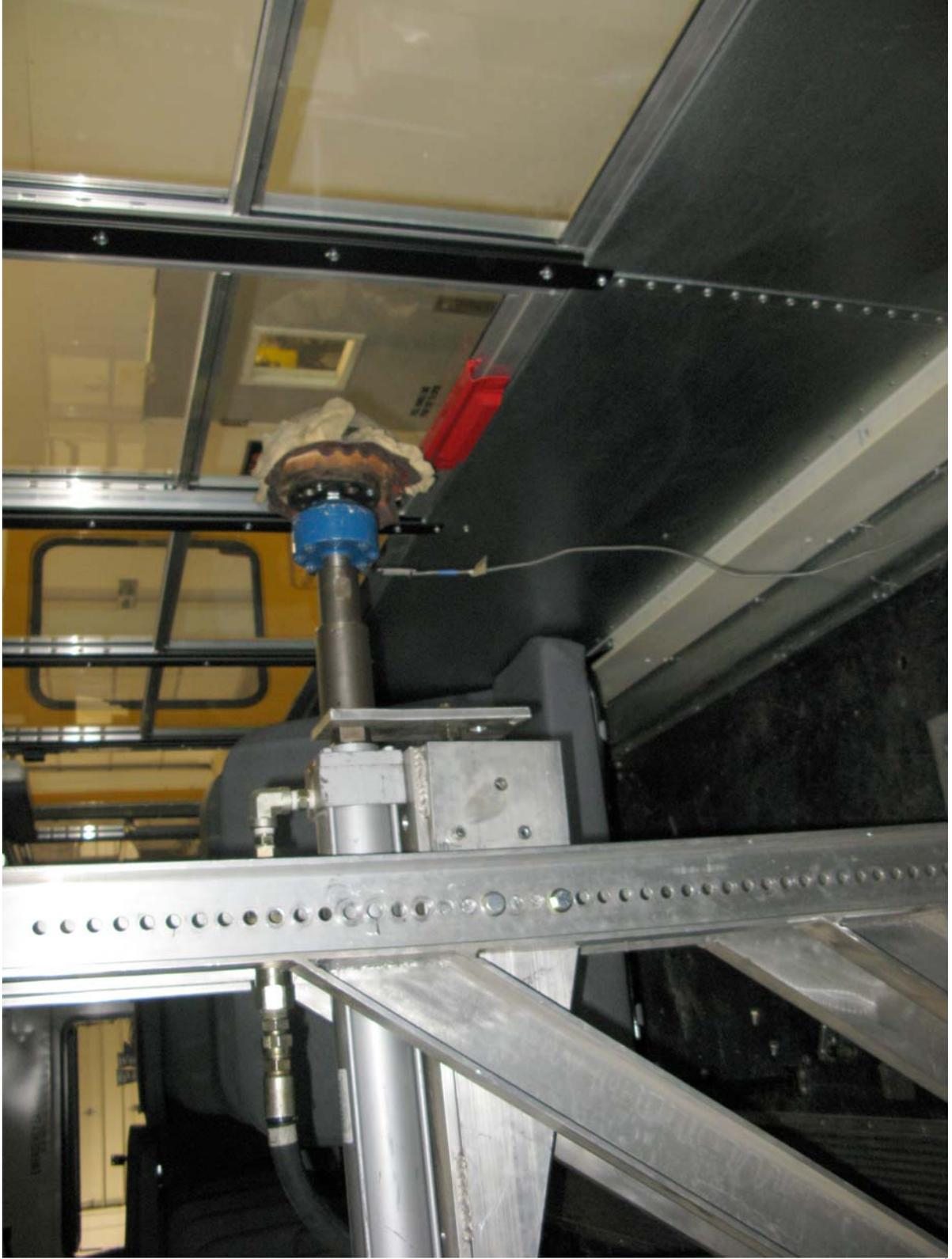
Retention Test of Left Side Window (Pre-Test)
