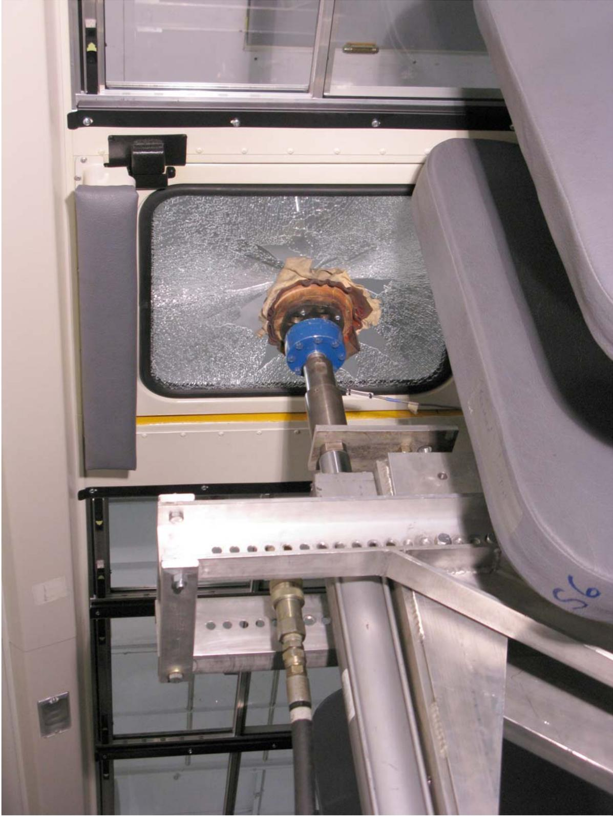
Retention Test of Left Side Door Exit (Post-Test)
