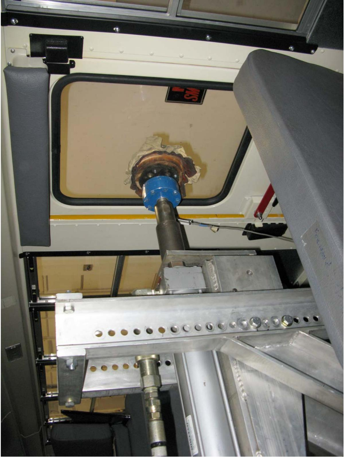
Retention Test of Left Side Door Exit (Pre-Test)
