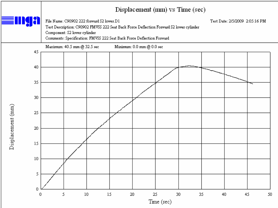
Seat Back Forward Deflection Seat S2 Lower Cylinder
