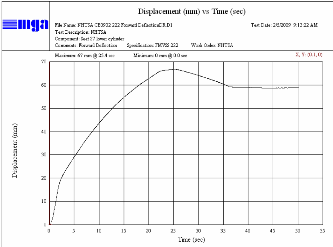
Seat Back Forward Deflection Seat S7 Lower Cylinder
