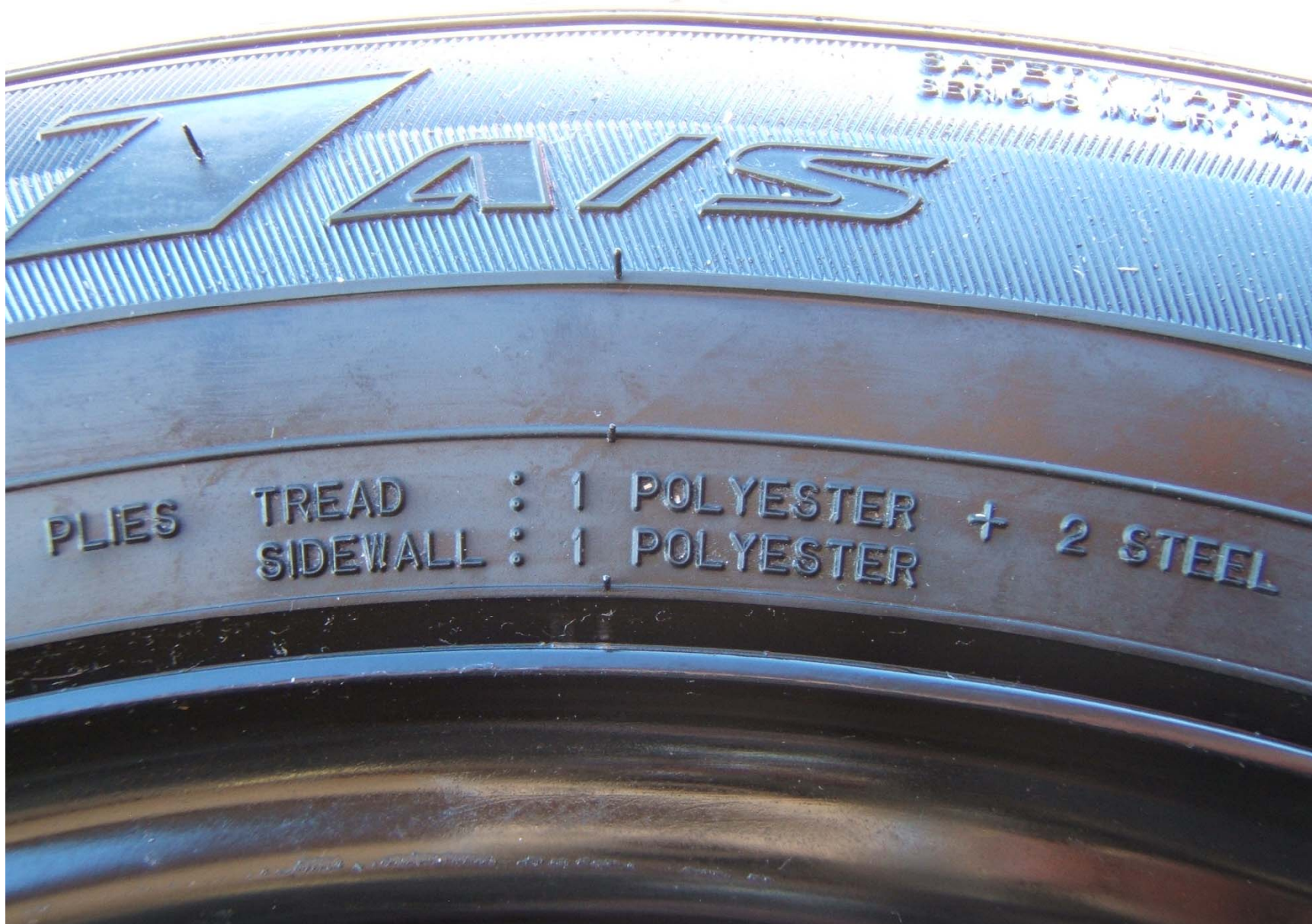
FIGURE 5.9 TIRE SHOWING SIDEWALL / TREAD CONSTRUCTION
