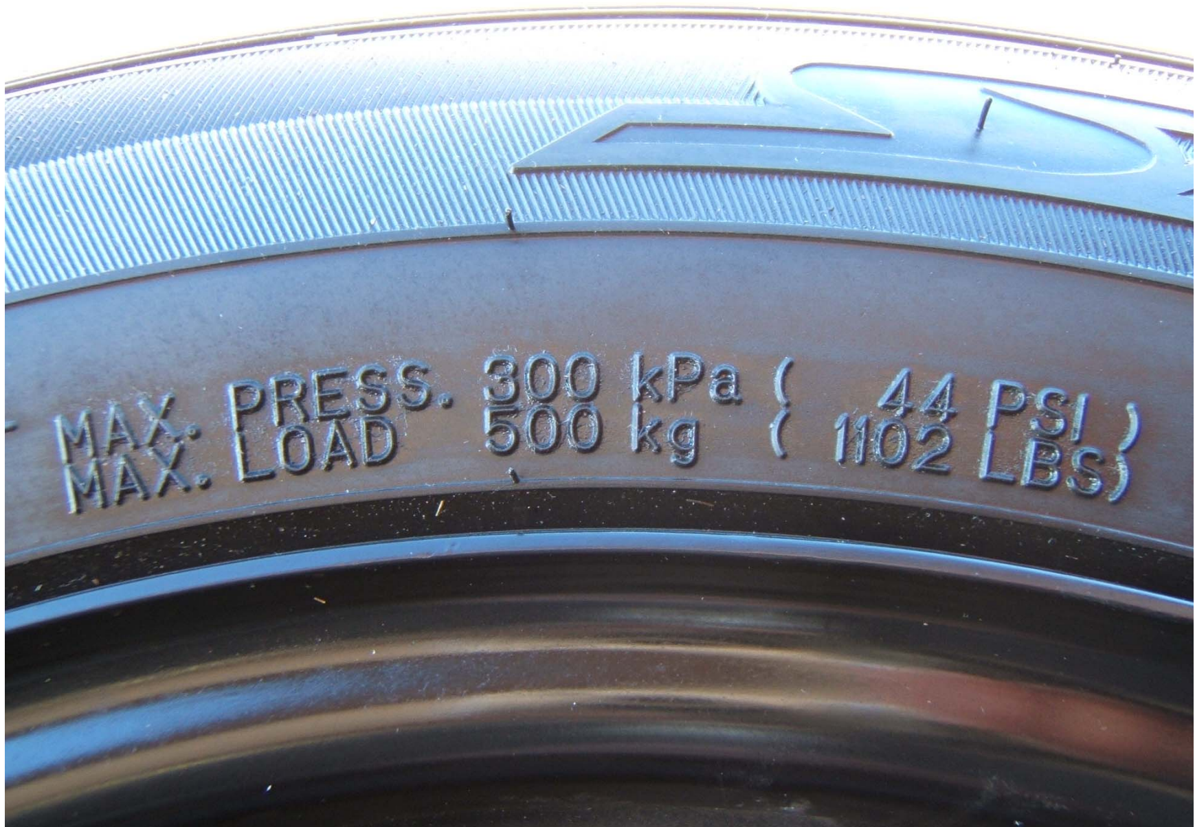
FIGURE 5.8 TIRE SHOWING MAX LOAD RATING AND MAX COLD INFLATION PRESSURE
