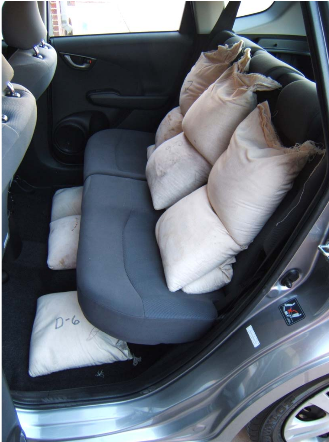
FIGURE 5.15 VEHICLE REAR SEAT BALLAST FOR UVW + VCW LOAD
