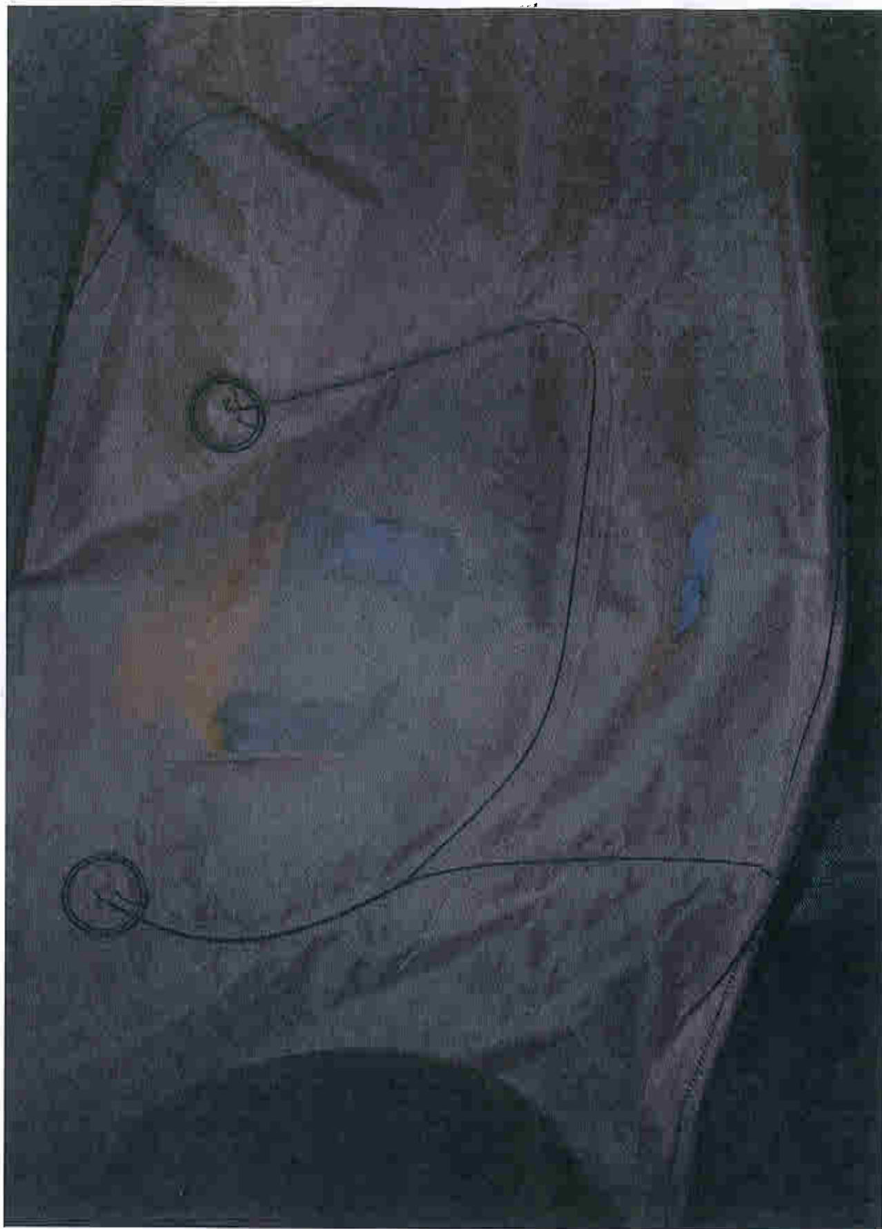
Post-Test Driver Dummy Head Contact (CAB)
