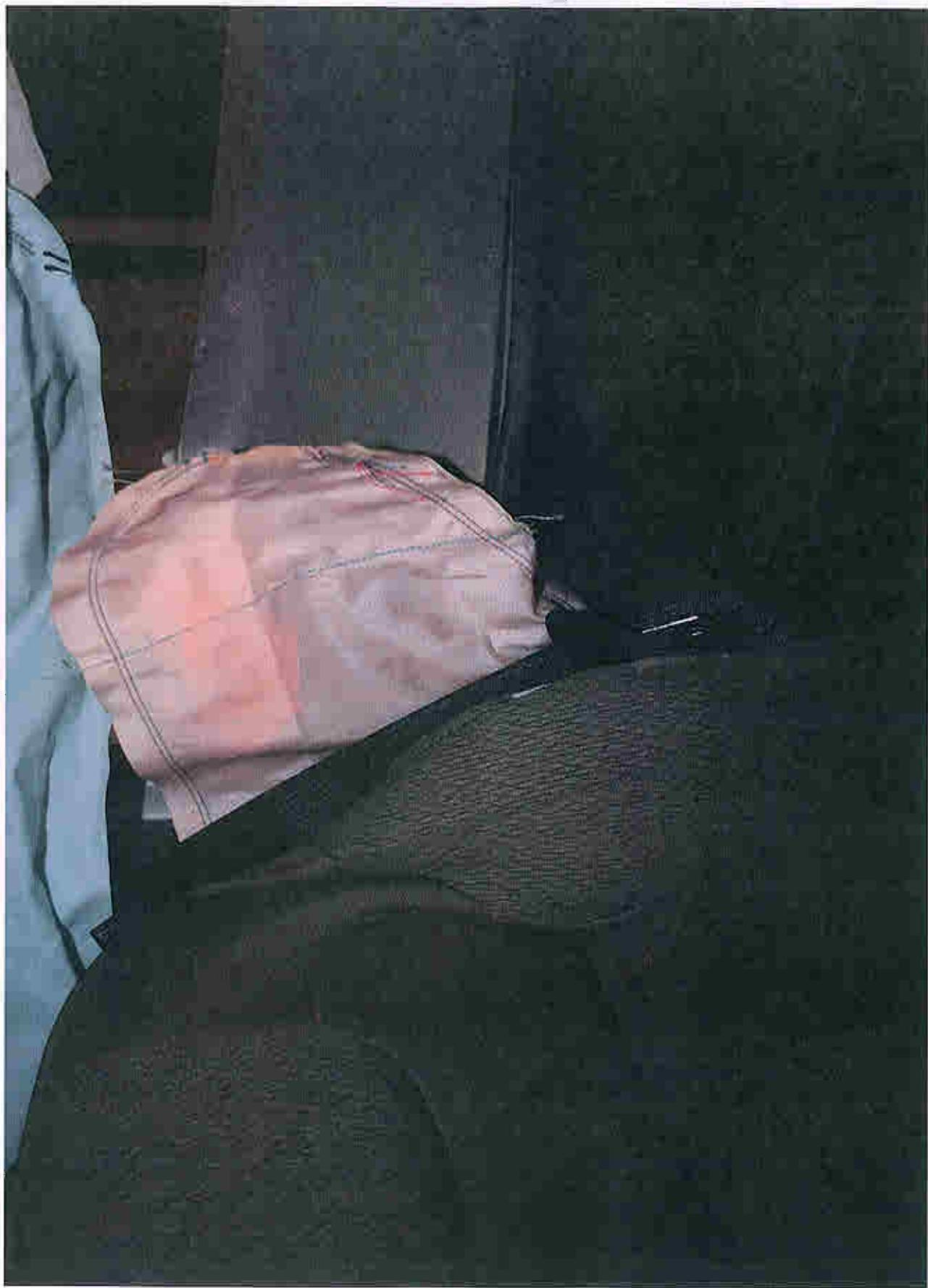
Post-Test Driver Dummy Upper Thorax Contact
