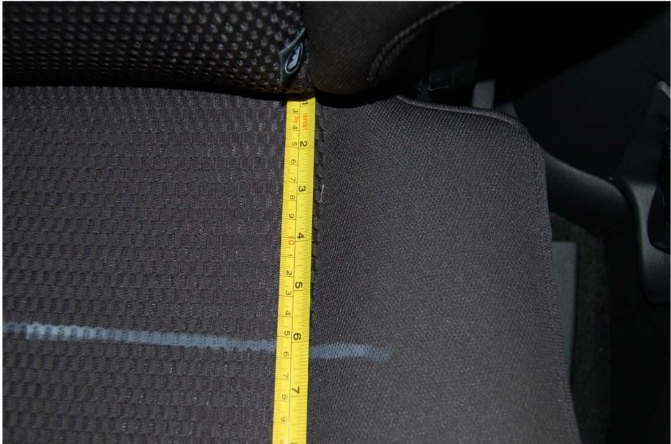
FIGURE 5.32 ROW 2, LEFT SIDE, OUTBOARD SRP MEASUREMENT
