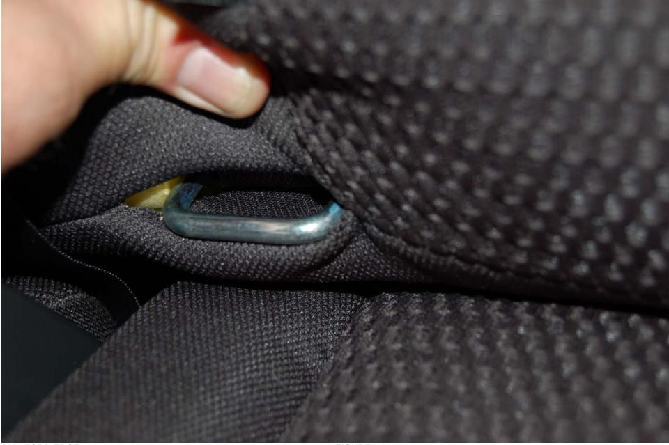
FIGURE 5.8 ROW 2, LEFT SIDE, INBOARD LOWER ANCHOR, PRE-TEST
