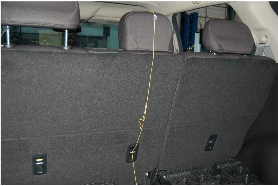
FIGURE 5.25 ROW 2, CENTER, TOP TETHER ROUTING
