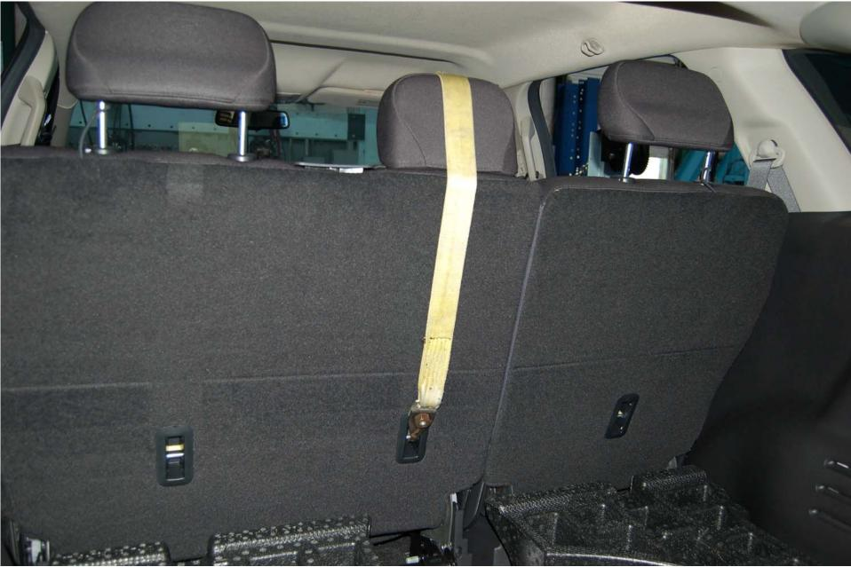
2008 FORD EDGE NHTSA NO. C80207 FMVSS NO. 225 FIGURE 5.49 POST TEST ROW 2, CENTER WITH SFAD 1
