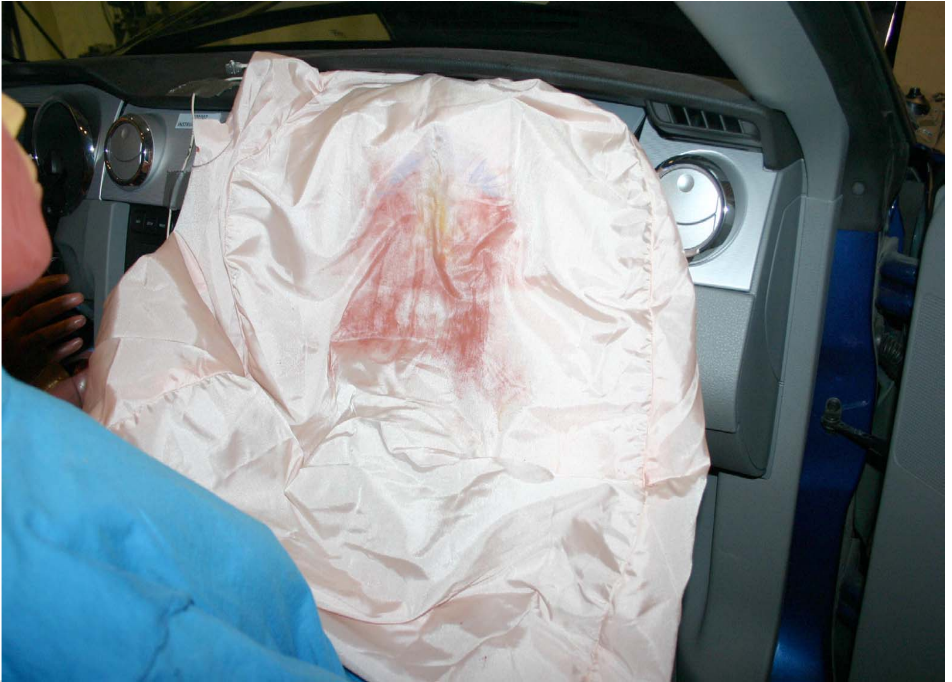
Post-Test Passenger Dummy Airbag Contact
