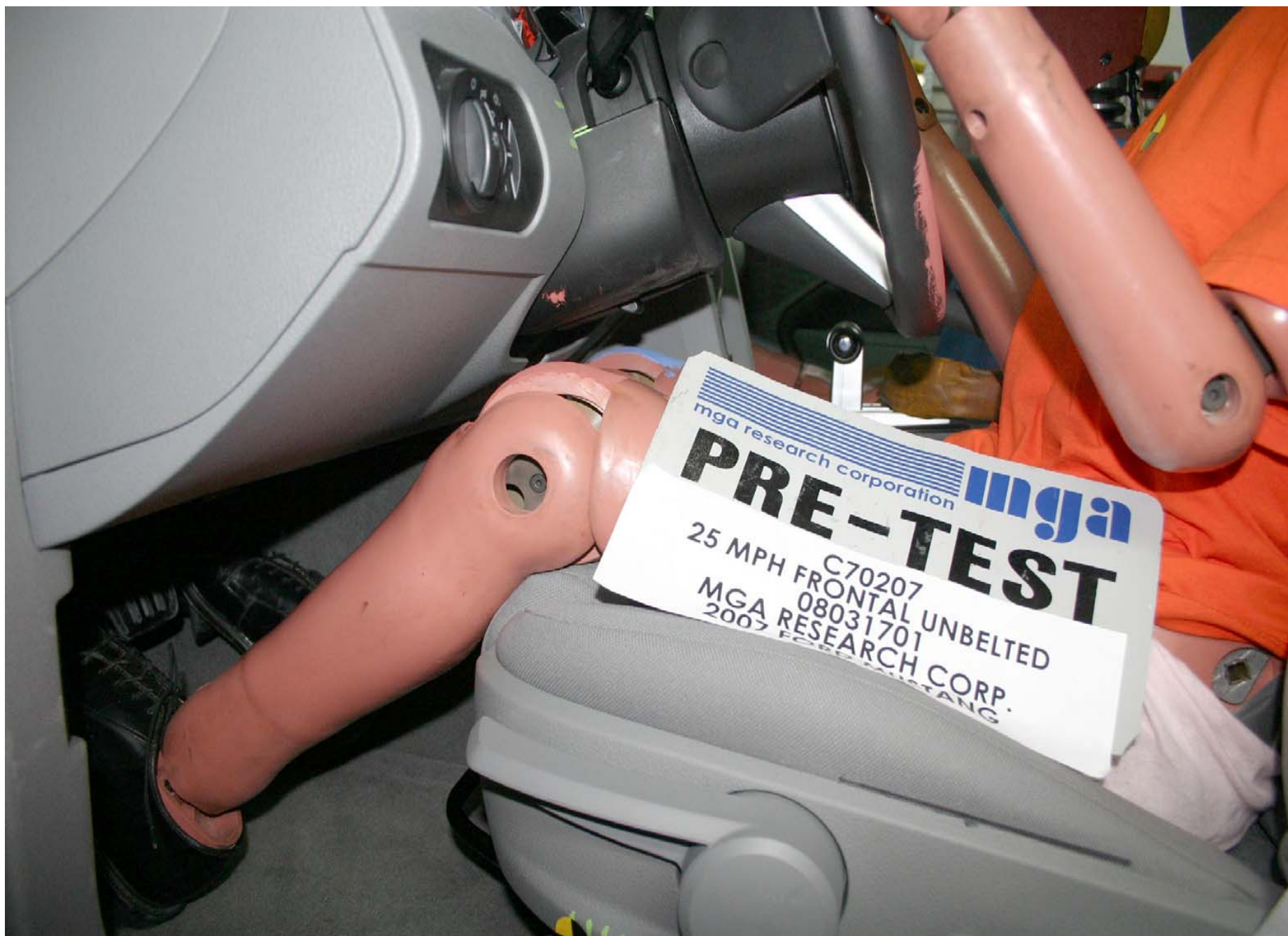
Pre-Test Driver Side Knee Bolster View
