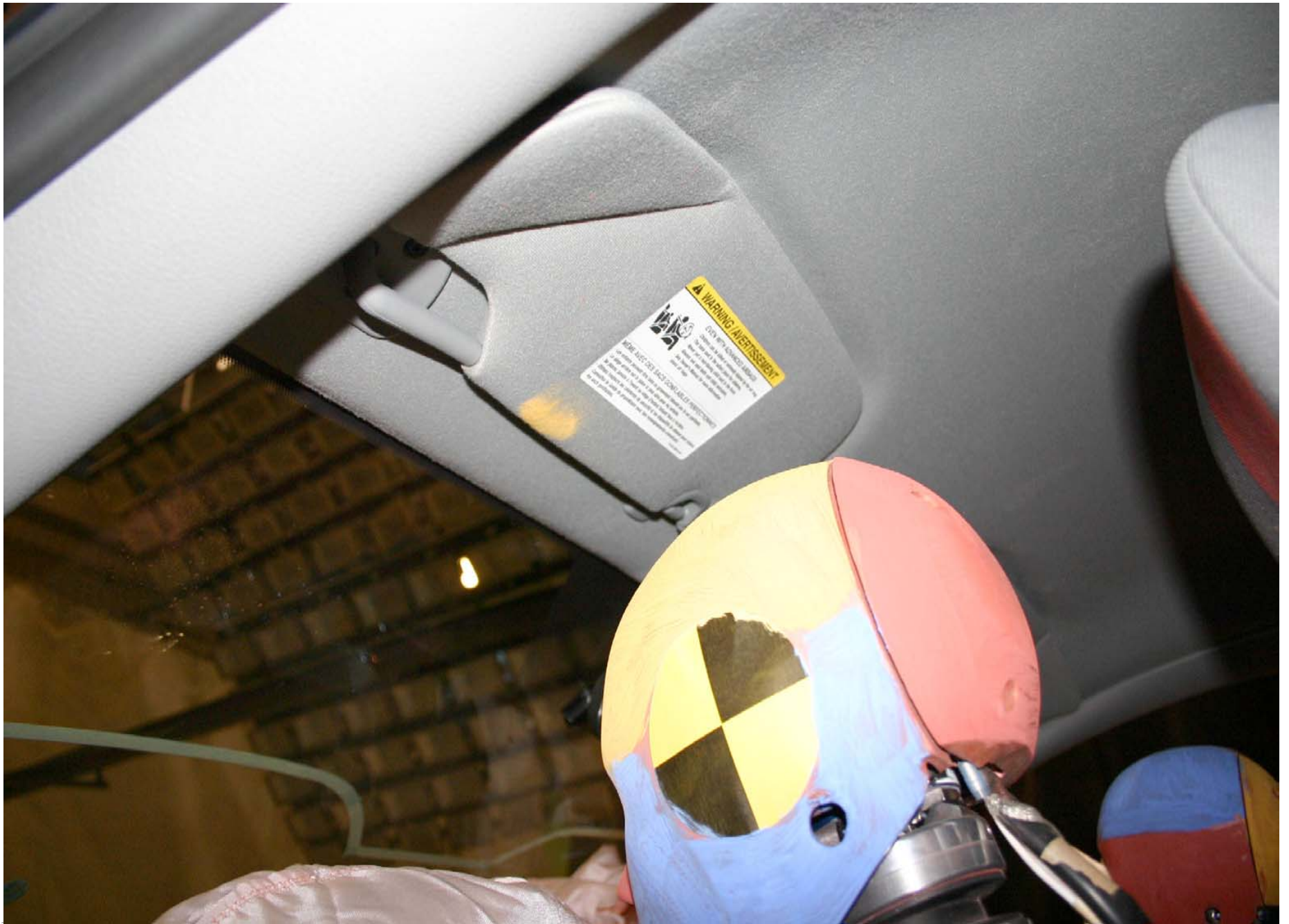
Post-Test Driver Dummy Head Contact (visor)
