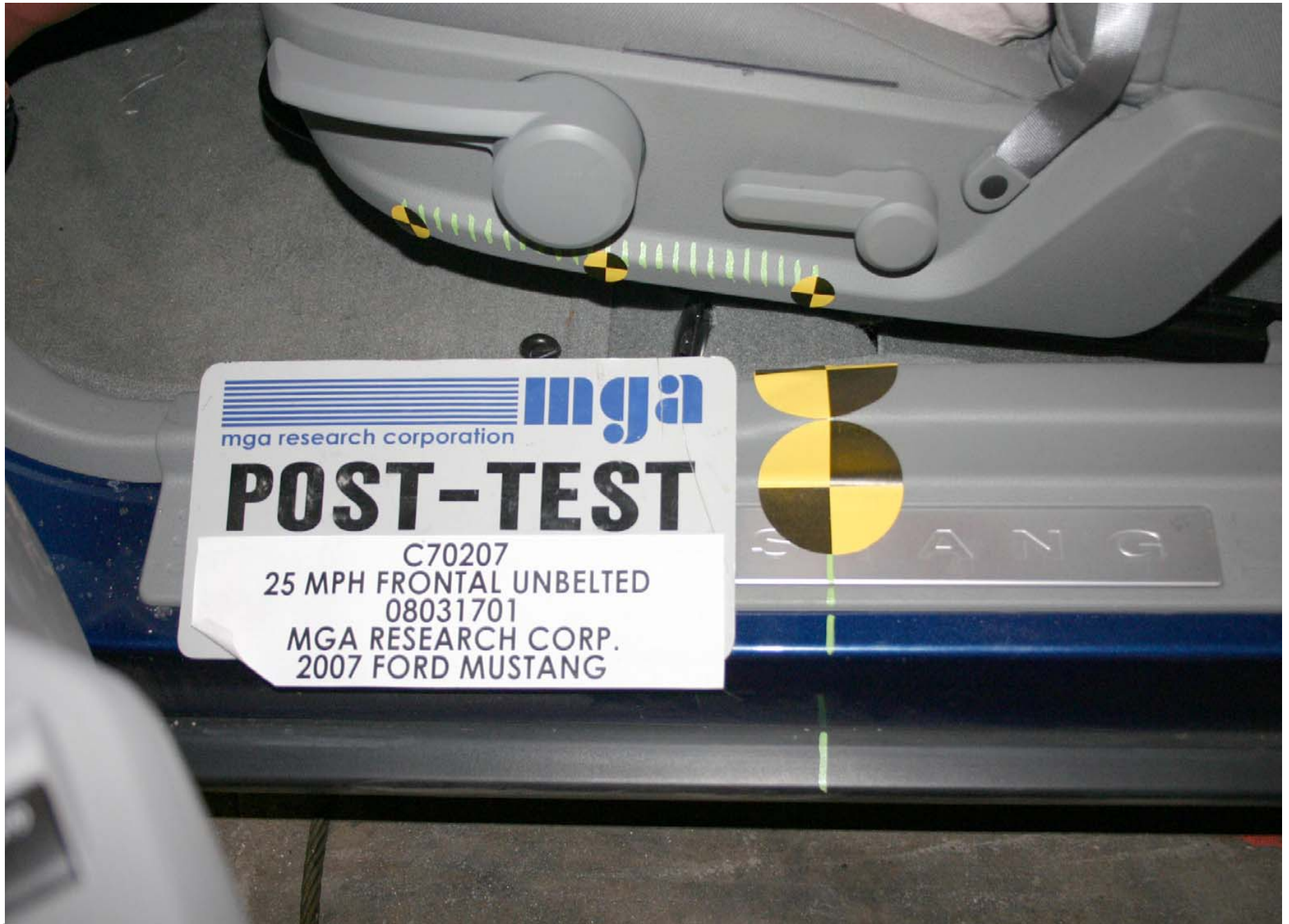
Post-Test Driver Dummy Seat Position
