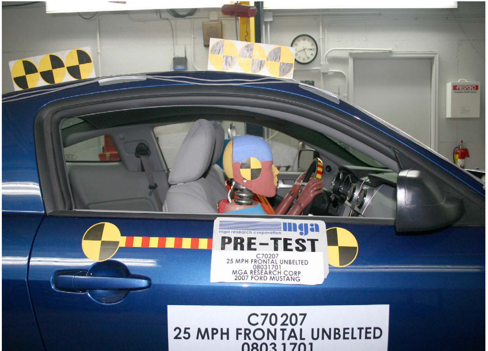
Pre-Test Passenger Dummy Position Right Side View
