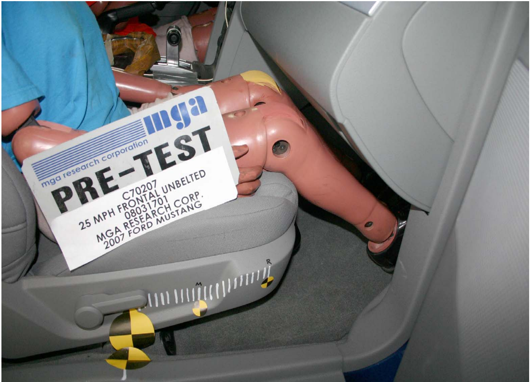
Pre-Test Passenger Side Knee Bolster View
