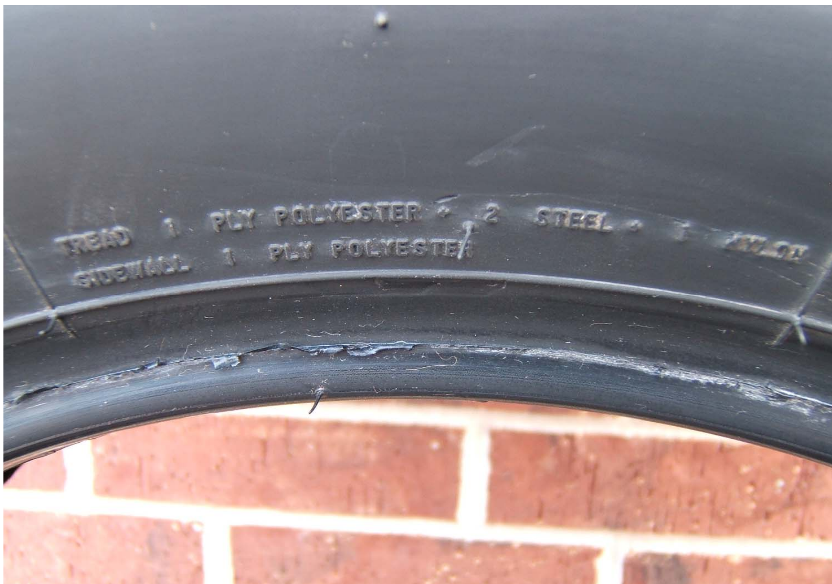
FIGURE 5.9 TIRE SHOWING SIDEWALL/TREAD CONSTRUCTION
