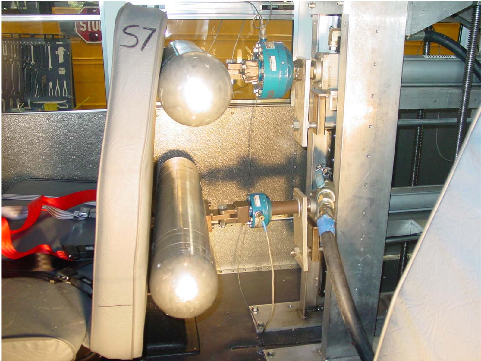
Pre-Test of Seat Back S7 Force Deflection Forward Test
