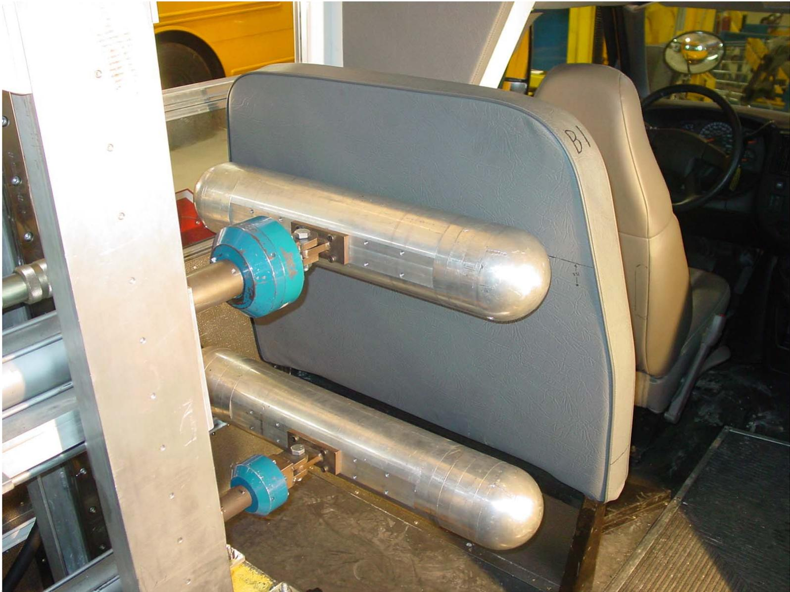
Pre-Test of Barrier B1 Force Deflection Forward Test
