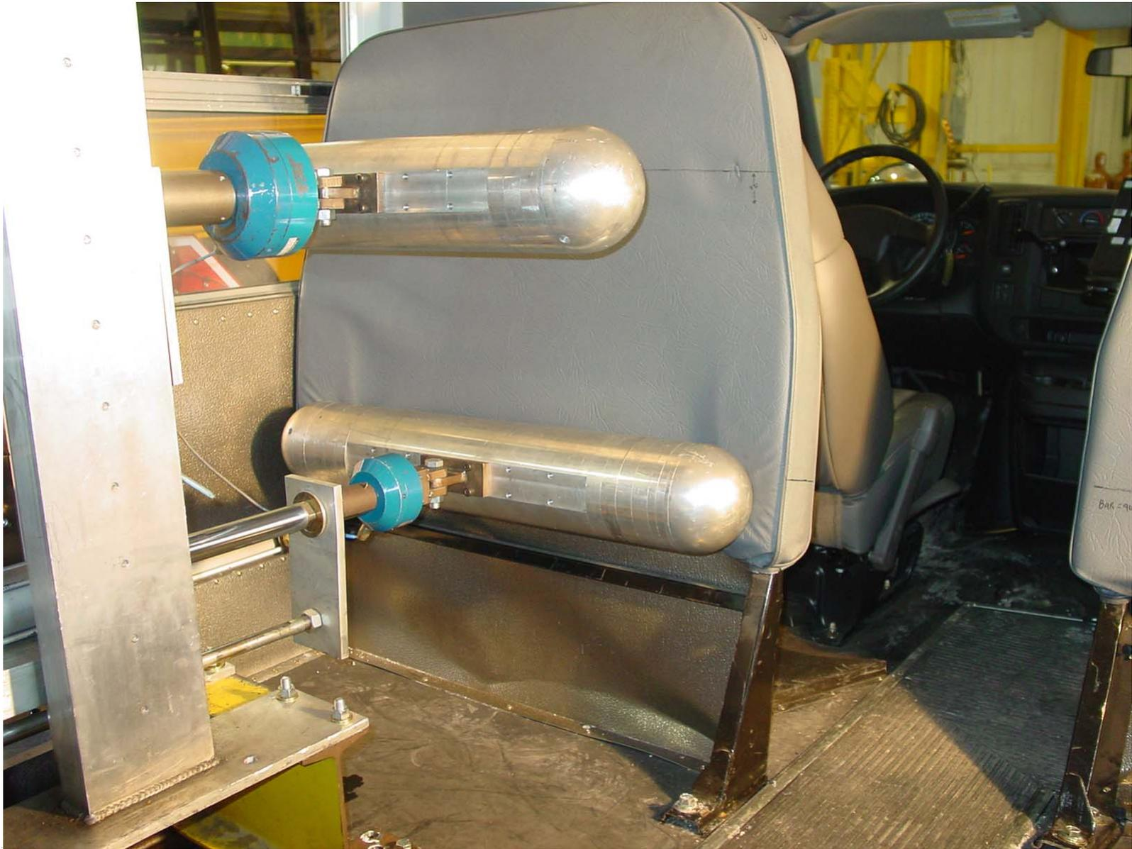
Post-Test of Barrier B1 Force Deflection Forward Test
