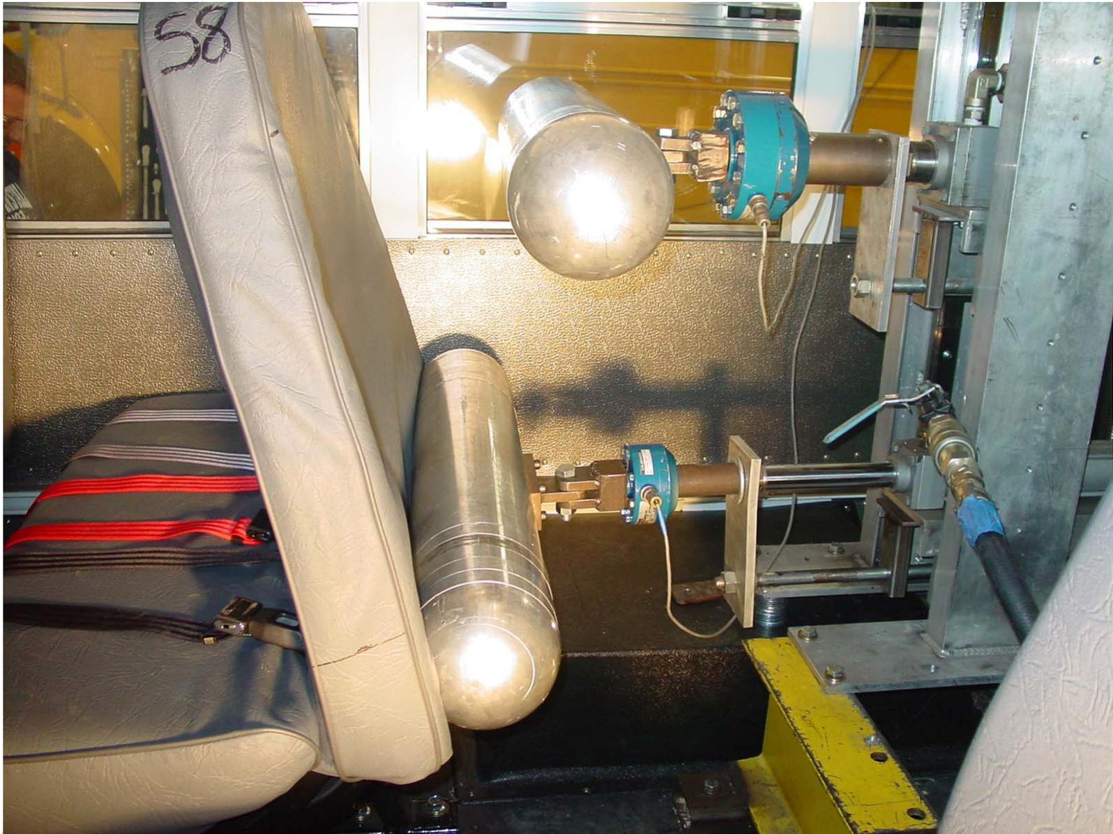
Post-Test of Seat Back S8 Force Deflection Forward Test
