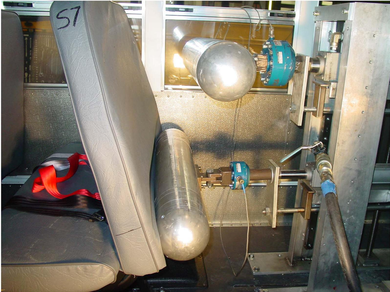
Post-Test of Seat Back S7 Force Deflection Forward Test
