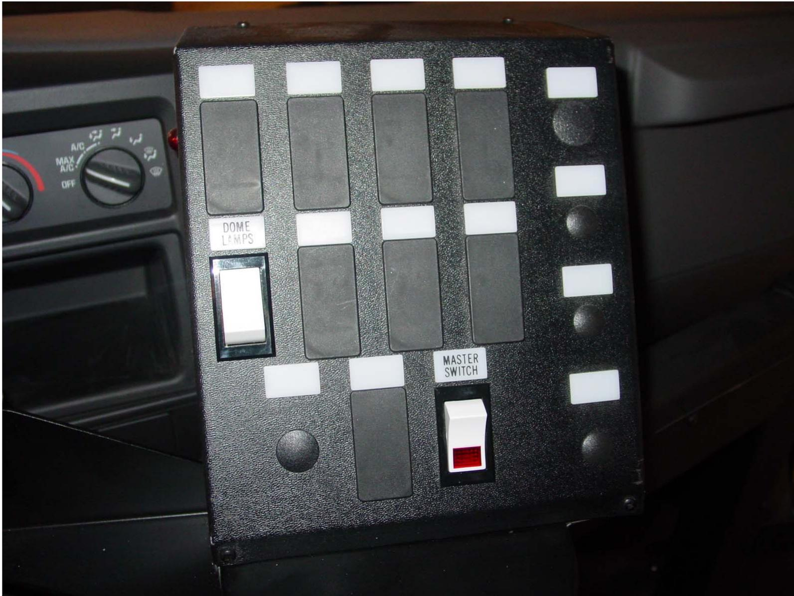
Photo 7 - Close Up View of the Switches That Allow Extension of the Stop Signal Arm(s)
