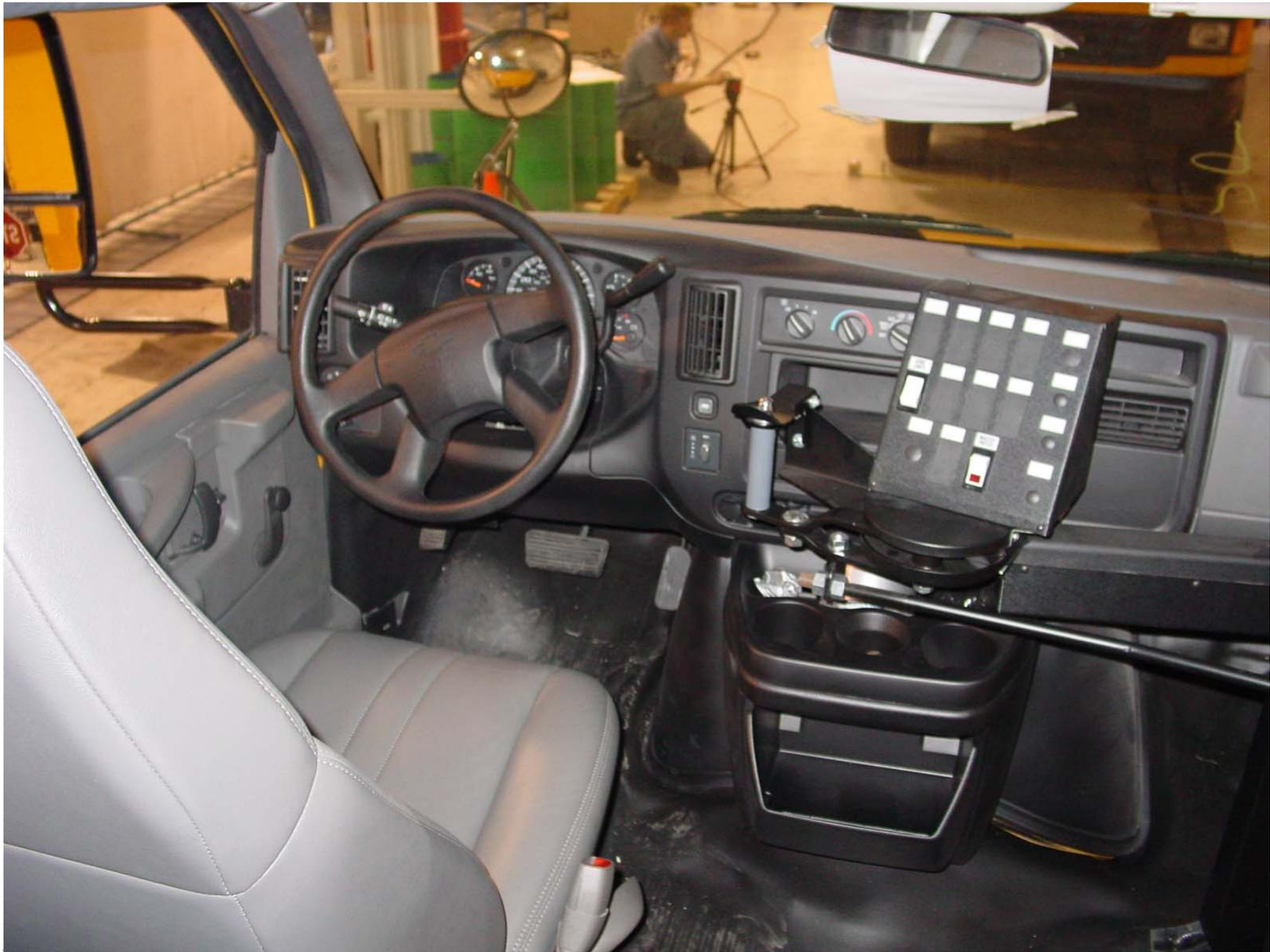
Photo 8 - Switch Console Relative to the Driver Seating Position
