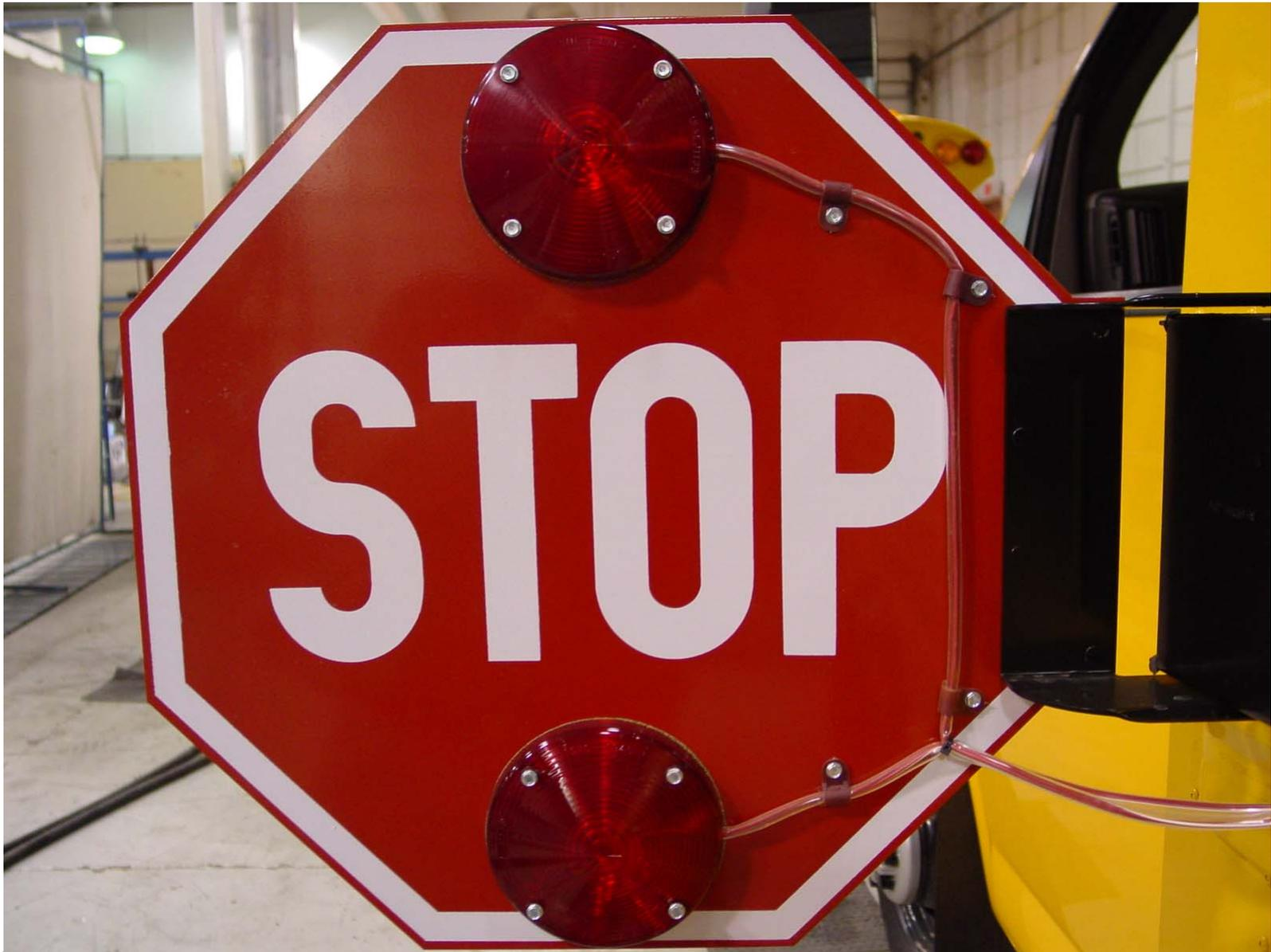
Photo 6 - Back Close Up View of Stop Signal Arm
