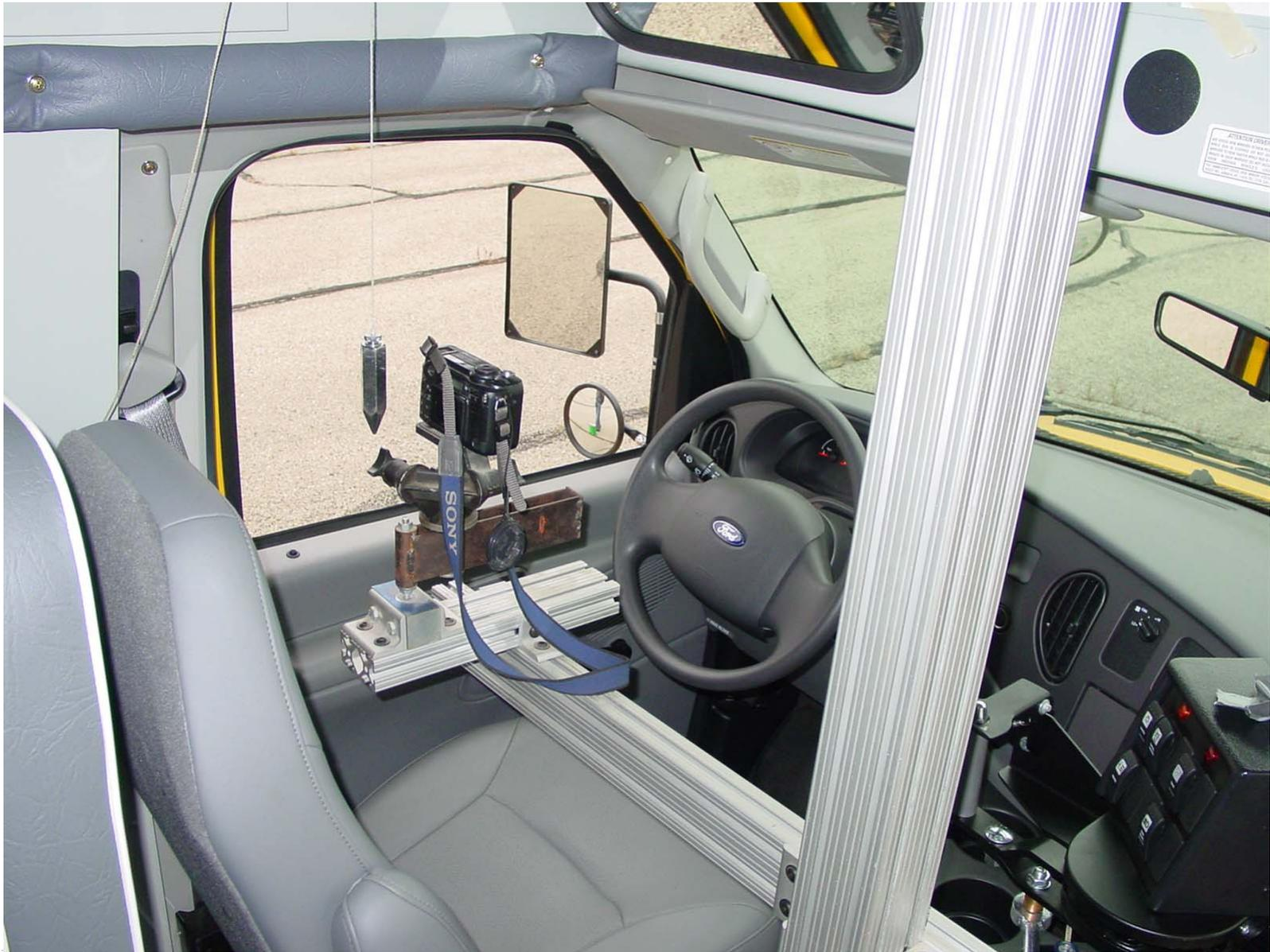
Photo 11 -Field of View Instrument Setup
