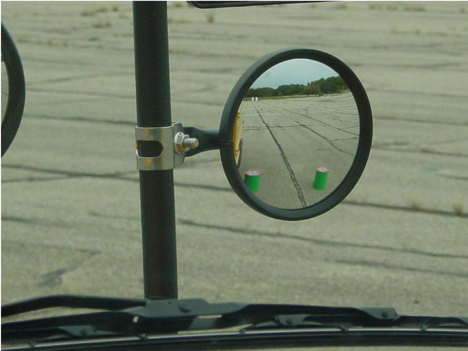
Photo 17 -Mirror #6 System A Field of View
