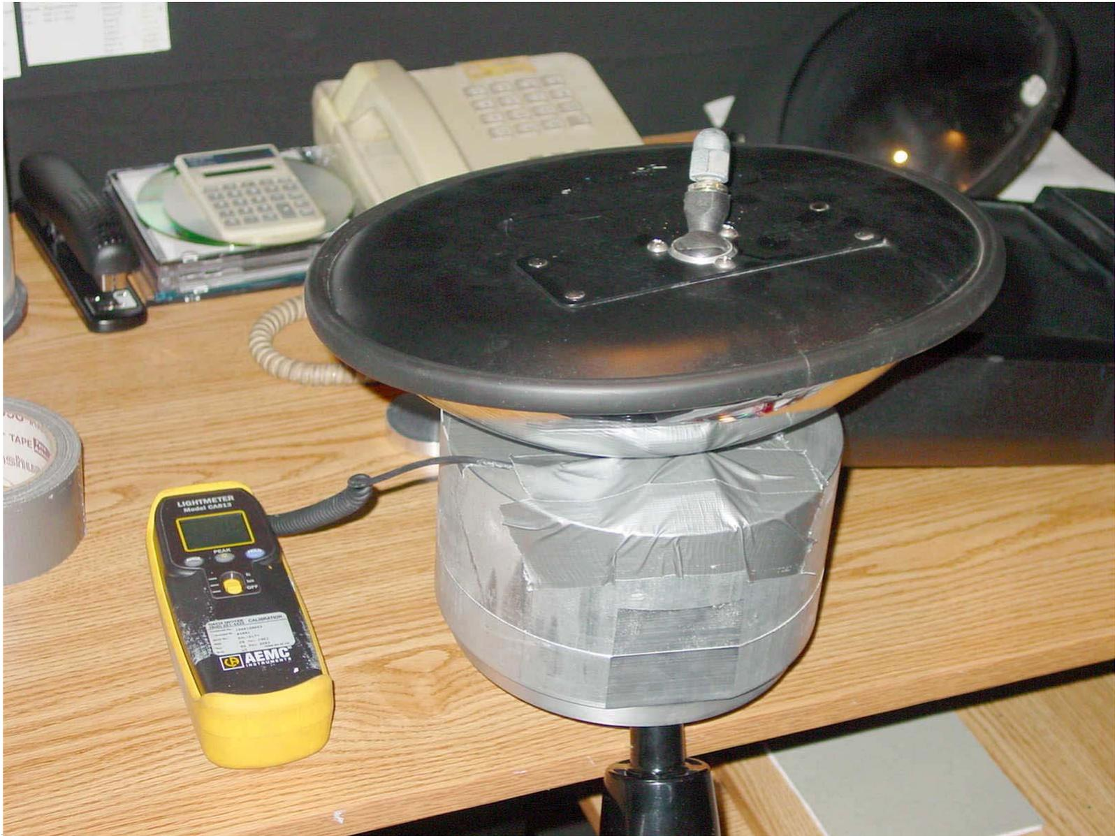
Photo 22 -Reflectance Test Set-up
