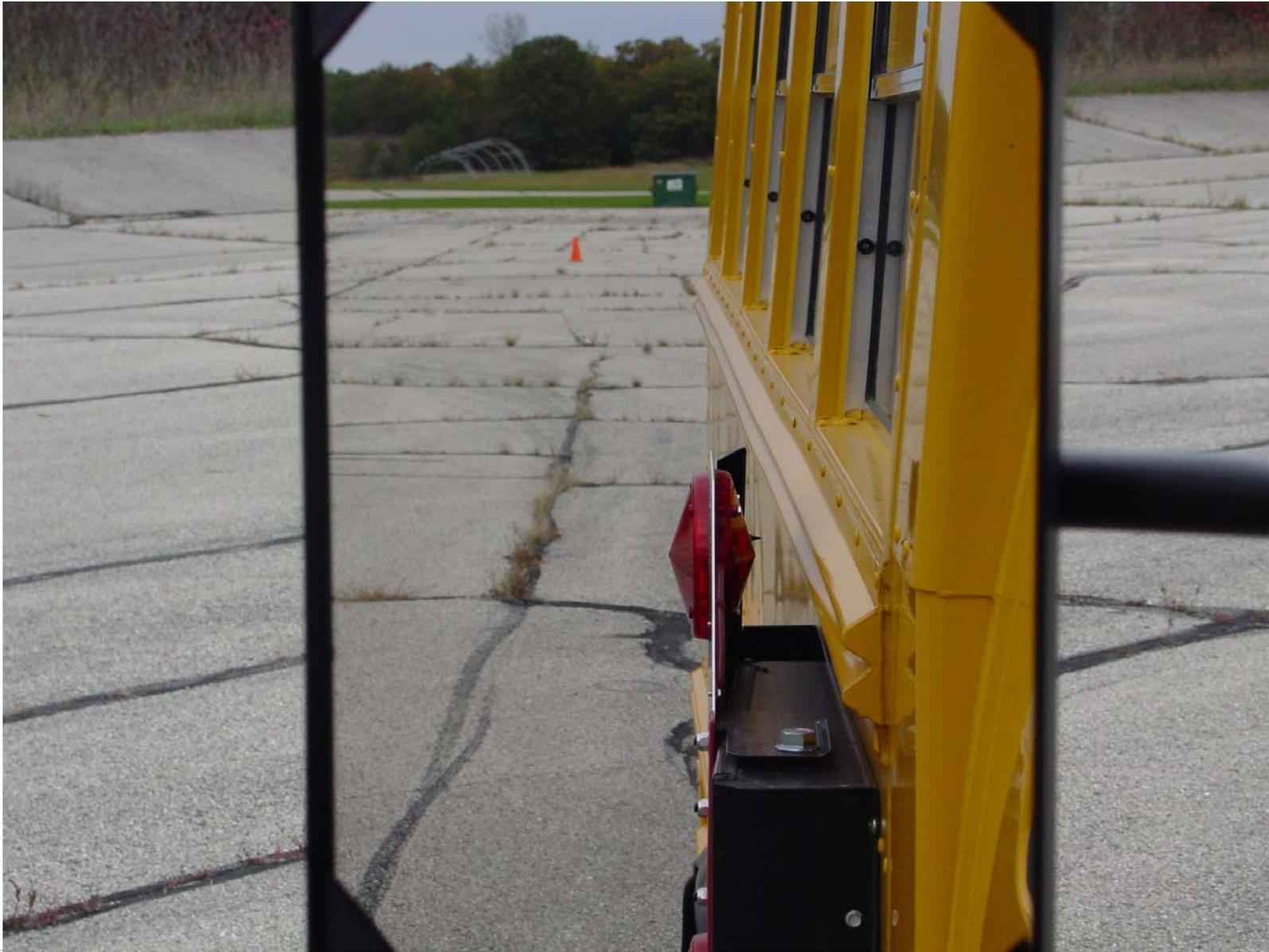
Photo 16 -Mirror #3 System A Field of View
