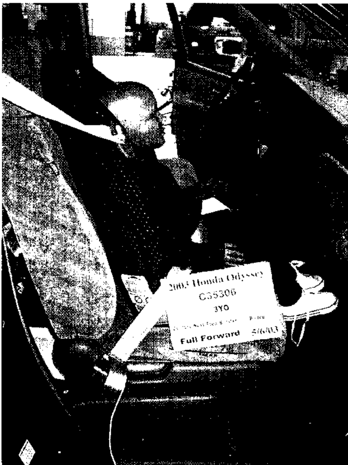
Figure 7-29: Century Next Step, Belted, w/ a Booster Harness, Full Forward as Possible Seat Position
