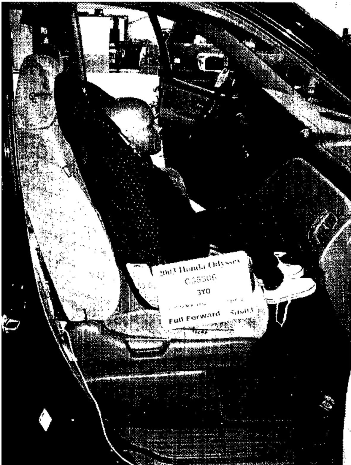
Figure 7-28: Century Next Step, Unbelted, w/o Booster Harness, Full Forward as Possible Seat Position
