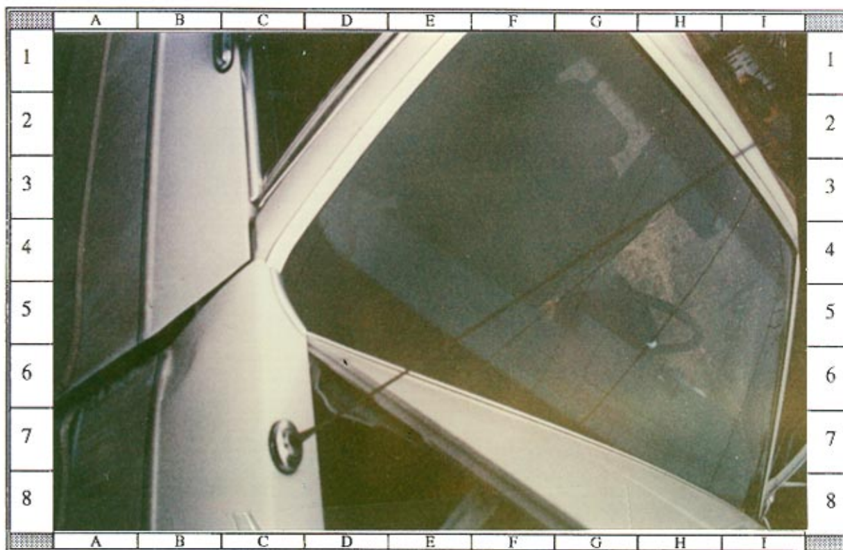
# 04 -- 1991 Ford Crown Victoria LX's R fender & RF door showing induced damage from deer impact; NOTE: windshield damage not visible
