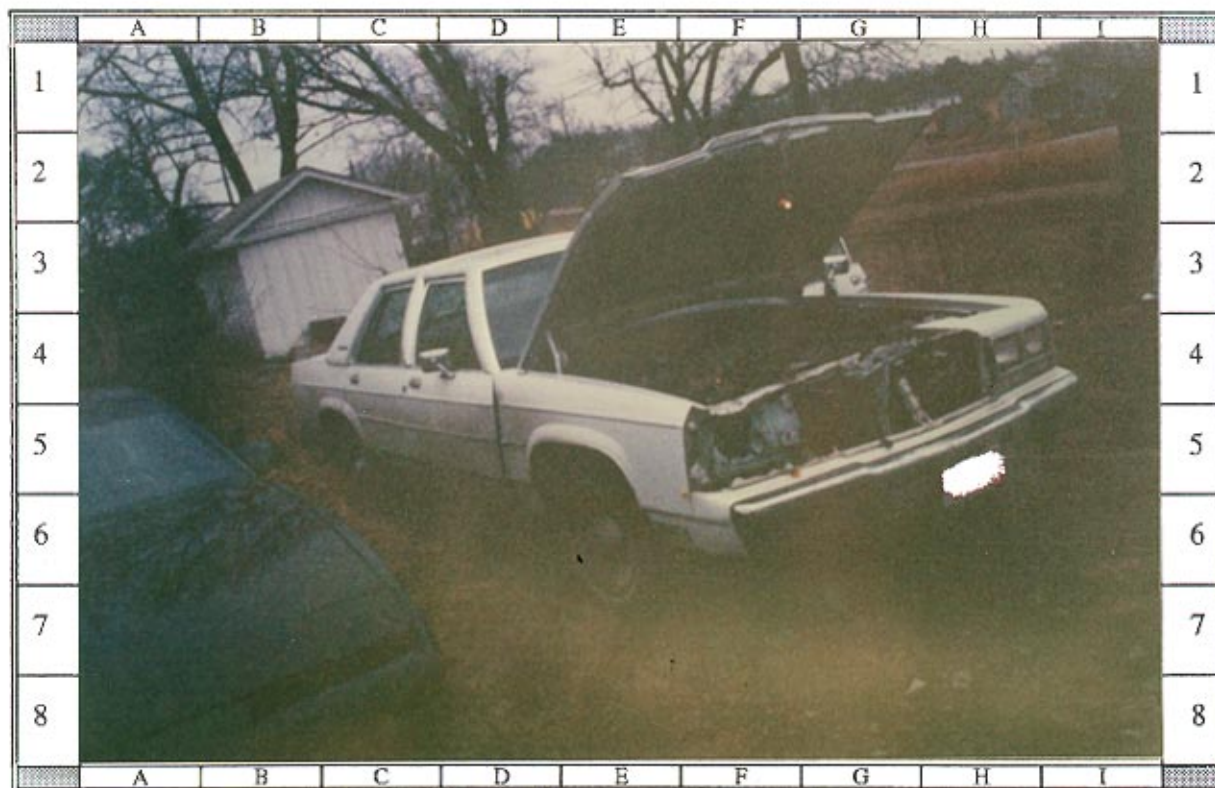
# 02 -- 1991 Ford Crown Victoria LX's front center & right damage viewed from front right; NOTE: induced damage near right front door
