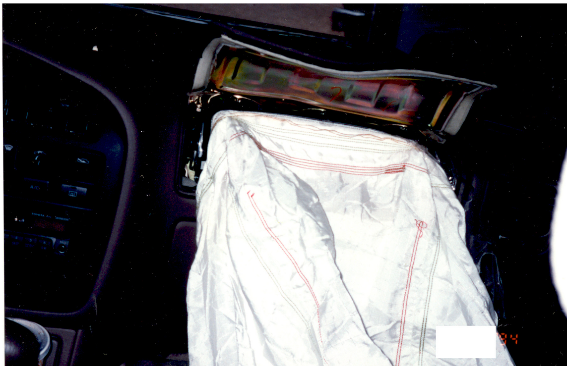
Photo #3 Toyota Avalon interior passenger side air bag module cover.
