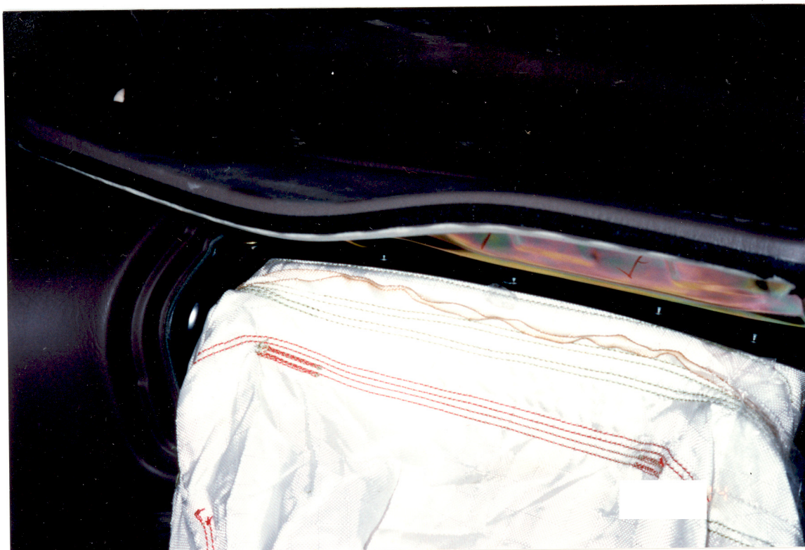
Photo #4 1995 Toyota Avalon interior passenger side air bag module cover close-up.
