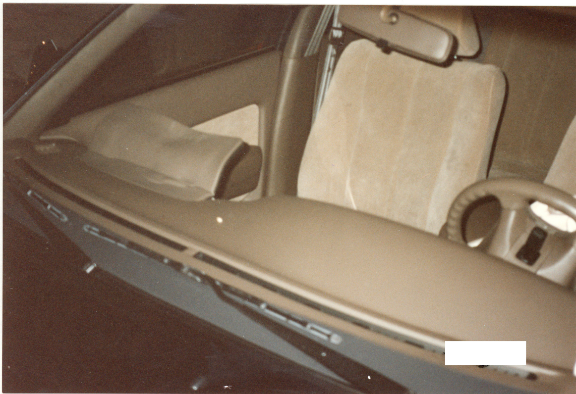
Photo #2 1995 Toyota Avalon interior through windshield Note: Head contact to the passenger side air bag module cover
