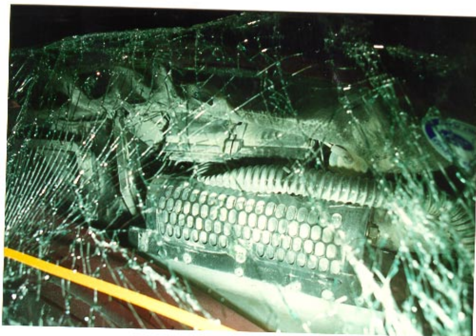
16. Heater tube compressed against the air bag generator.
