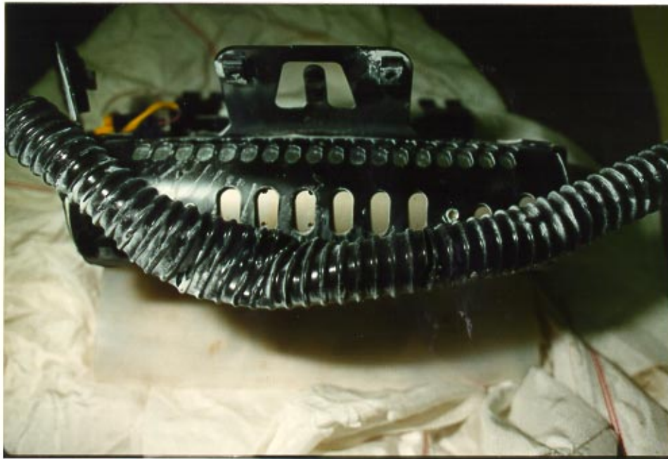
17. Melted heater tube fused to the heat shield around the generator.
