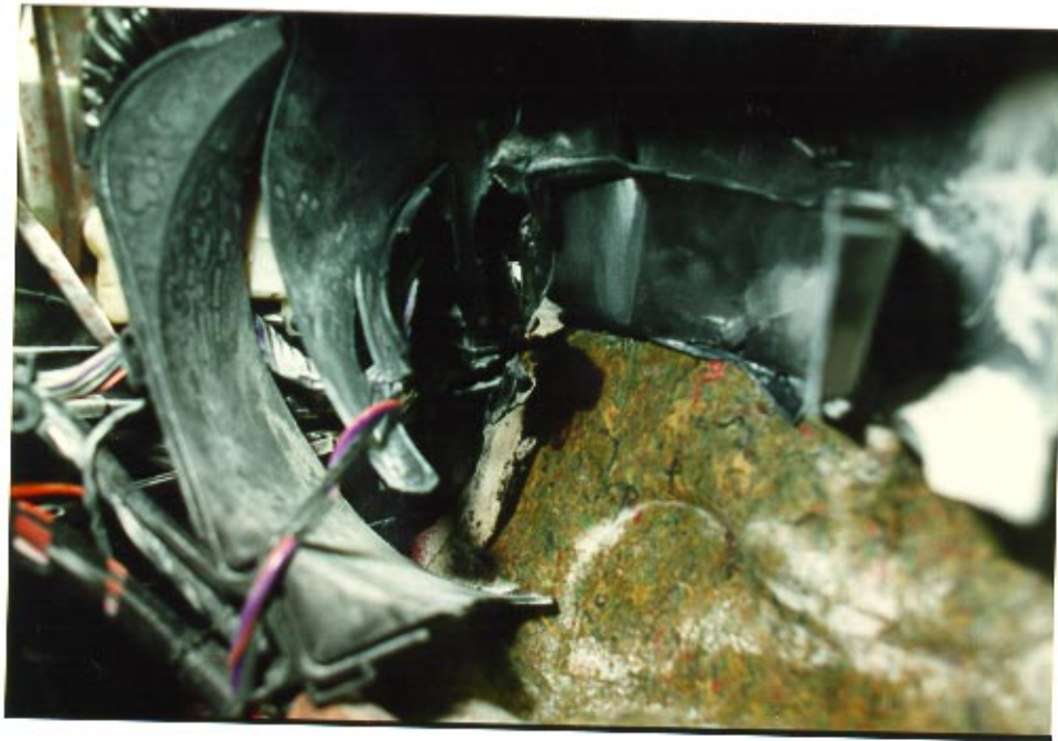
25. Source of the fire at the heater blower switch resistor assembly.
