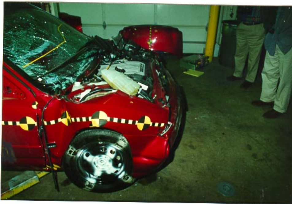
3. & 4. Perpendicular views showing the extent of frontal crush.
