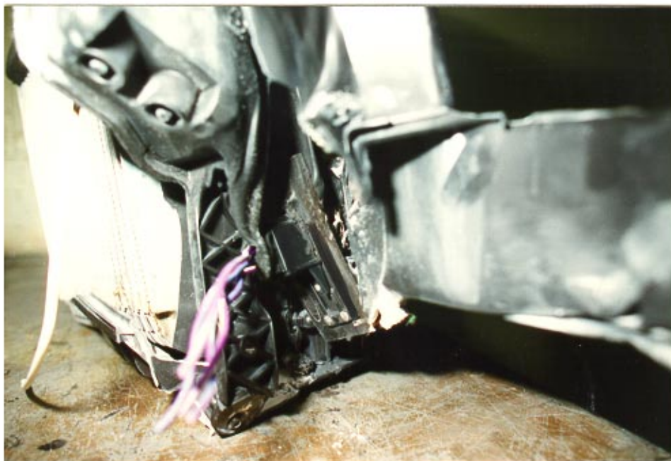
30. Damaged switch with the exposed resistor coils.
