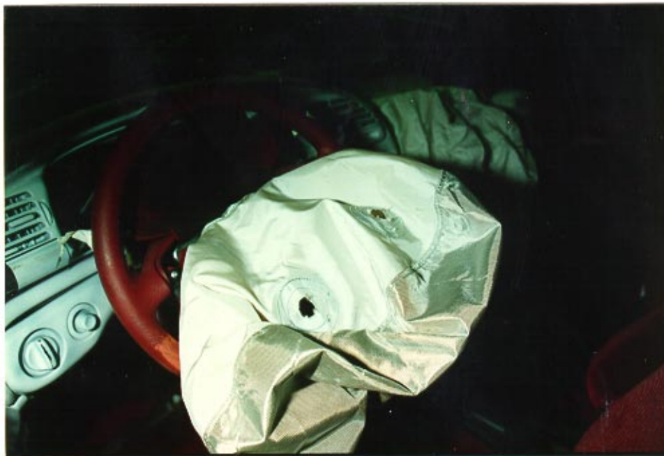
8. Vent ports and upper flap configuration of the driver's side air bag.
