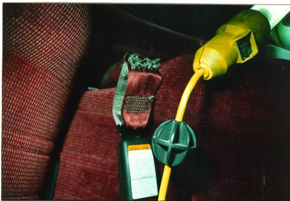
10. Separated energy management stitching in the right front belt buckle assembly.
