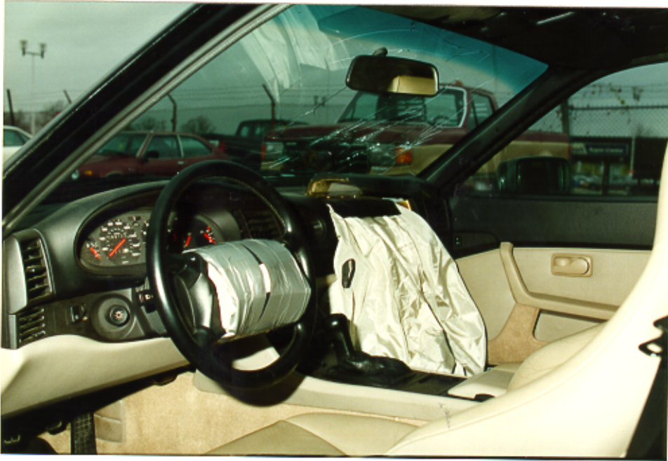
17. Overall view of the inadvertently deployed driver and passenger side air bags.
