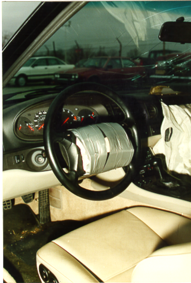
18. Driver/owner taped driver's side air bag module closed.
