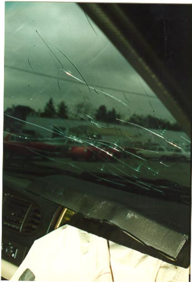
22. Passenger side module cover flap contact damage to the right windshield.
