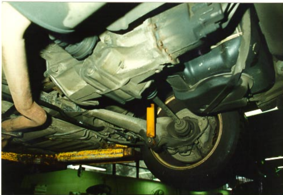
14. Transaxle, rear suspension components, and the retrofitted OEM rear anti-sway bar.
