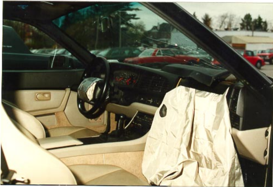
20. Inadvertently deployed passenger's side air bag.
