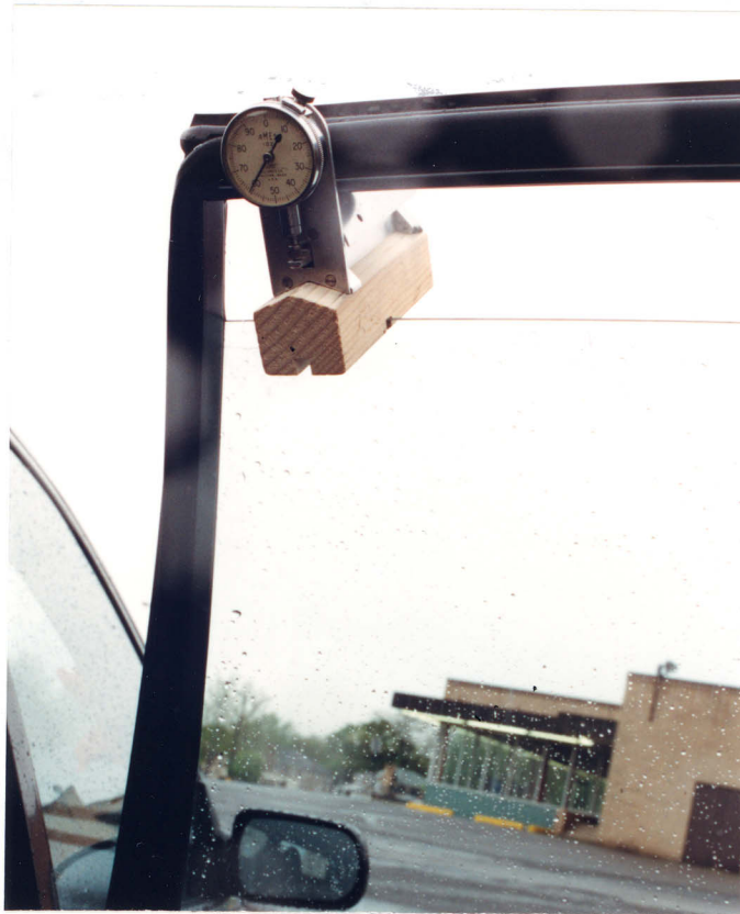
13. Force gauge positioned between the right rear window and the window frame adjacent to the B-pillar.
