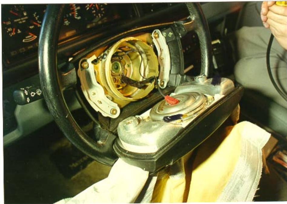
Air Bag Module Removed From Steering Wheel
