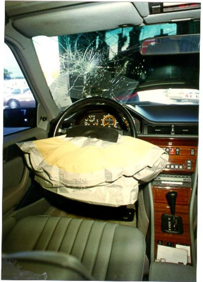
Overall Views Of The Driver's Seated Area, Related Contact Points, And Deployed Air Bag
