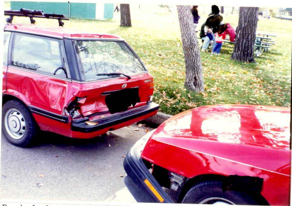
3. Back-left view of the Subaru showing impact damage and left-front corner of the Sundance.
